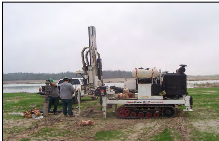
Groundwater sampling for PAH detection study.
