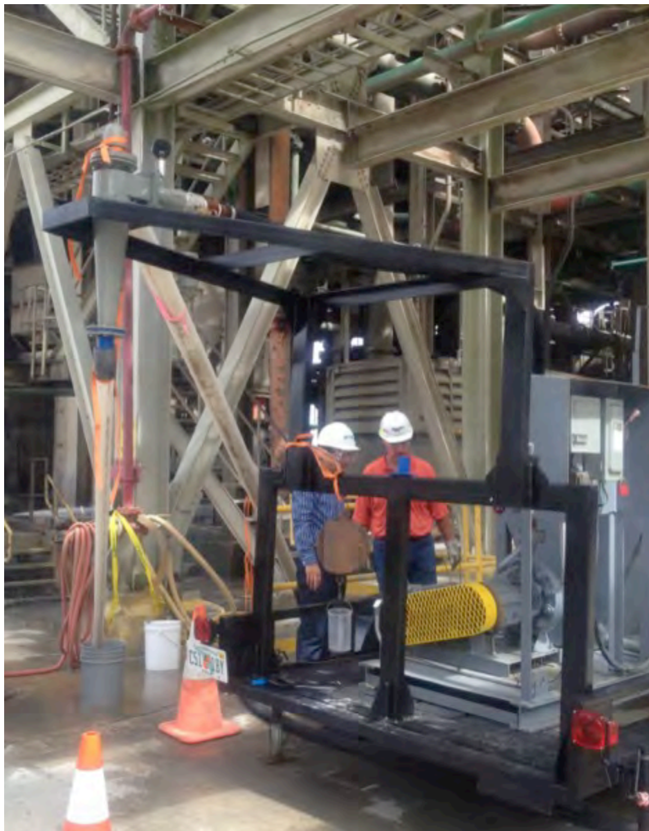
Continuous separation of waste clay using a hydrocyclone in pilot testing.
