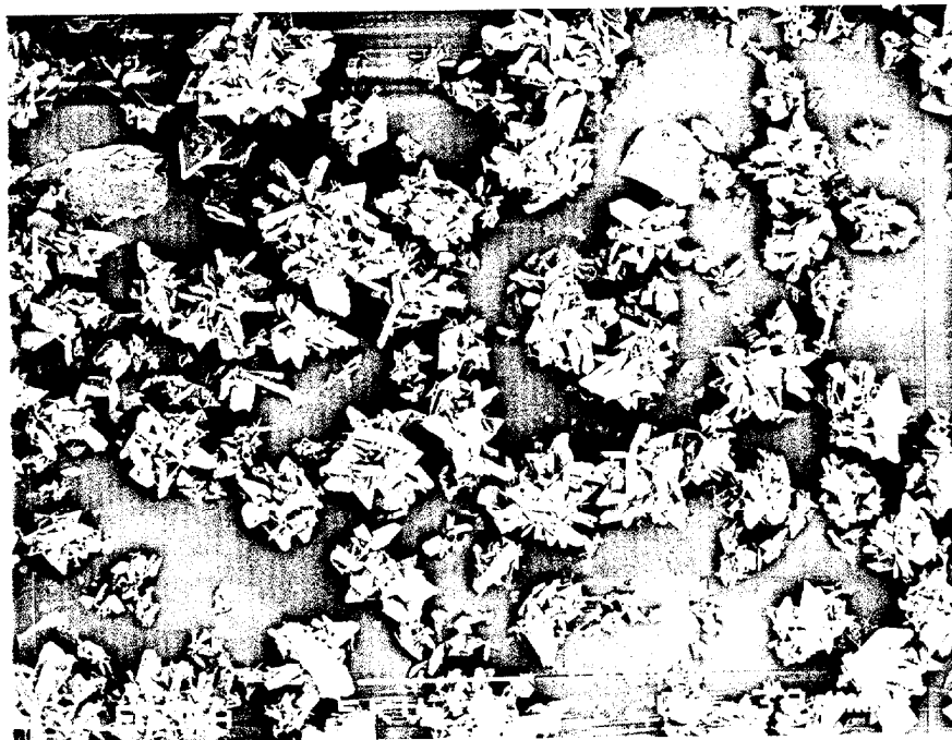
Figure 40: SEM micrograph of PEO-treated phosphogypsum (2.5 % sulfate)
