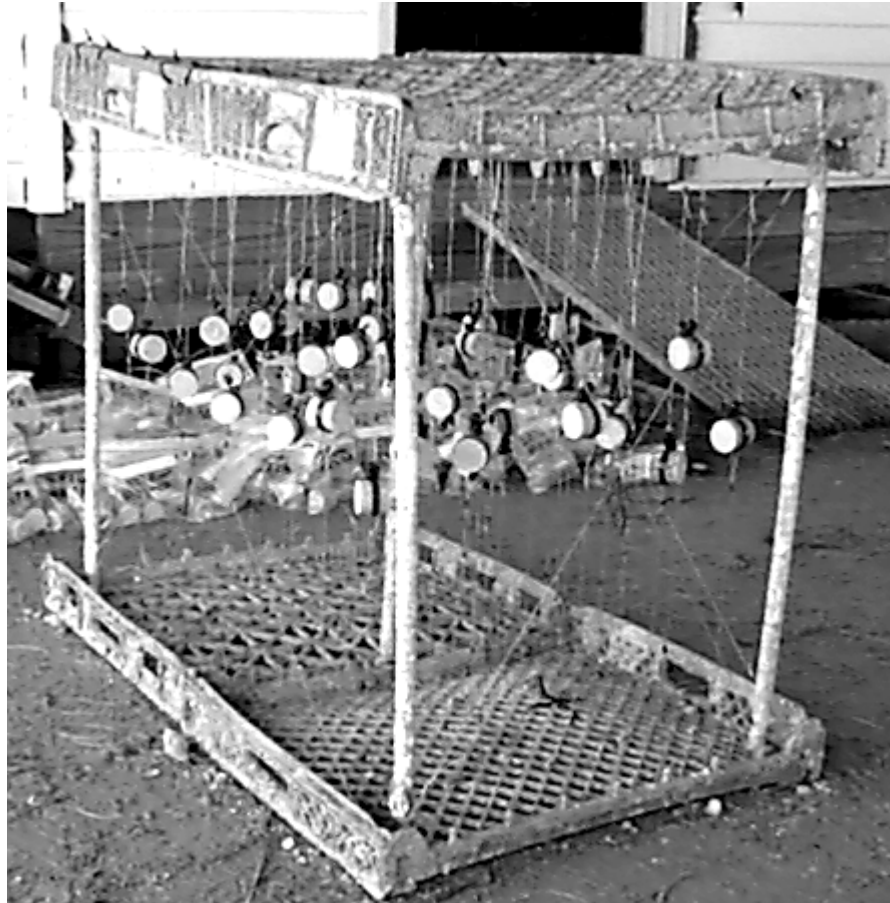
Figure 1. A Bread Crate-PVC Pipe Frame Used in the Field Submergence Tests. The Blocks Were Suspended Using Tie Strap and 100-lb Test Lines.
