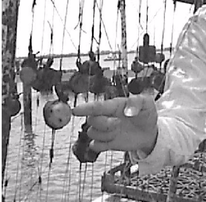
Figure 15. An Example of a Deteriorating PG/Cement/Lime Block Submersed at Grand Isle, LA. Edges Tend to Erode First, Rounding the Blocks.
