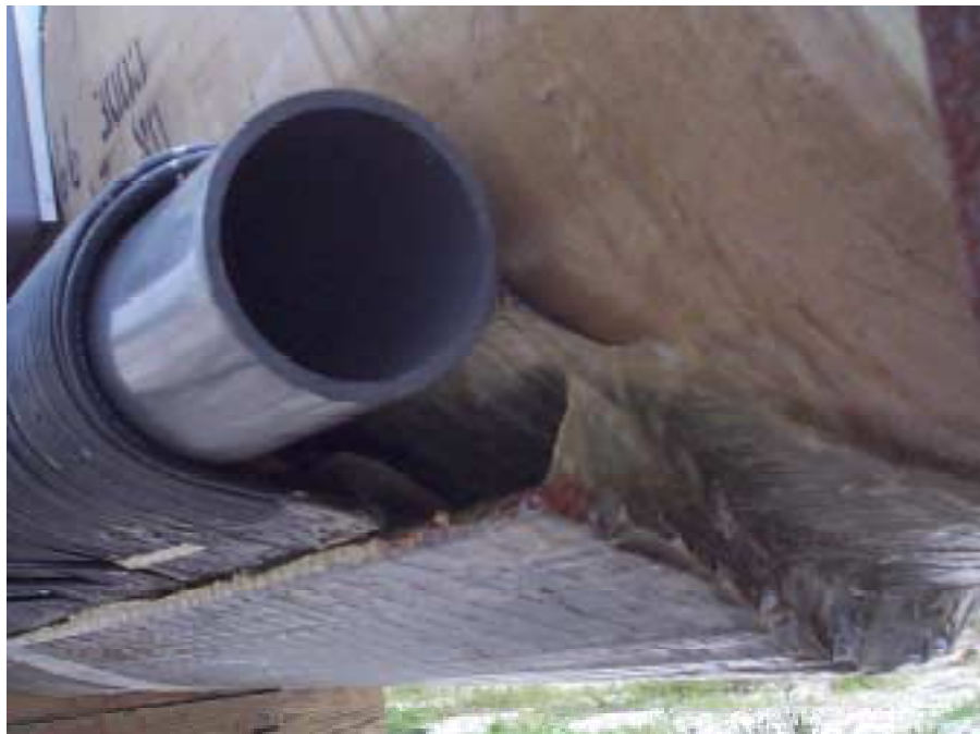
Figure 7. Close-Up of LSM Winding Showing End Turns and Back Iron.
