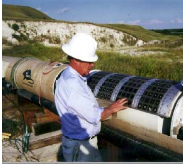
Figure 4. Magnet Assembly Rotated 180 Degrees for Inspection Purposes.
