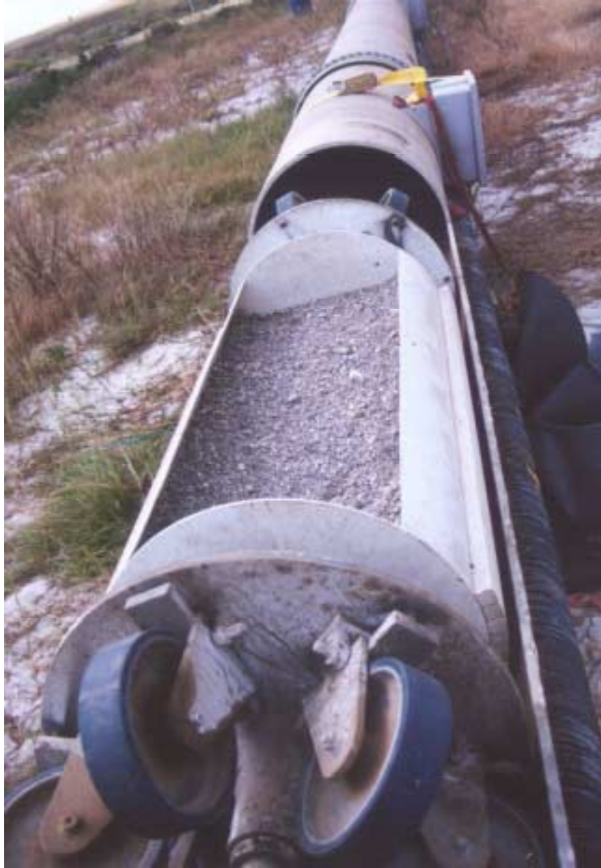
Figure 3. Car Loaded with 660 Pounds of Phosphate Rock Parked in the Opening Above Motor Number 3.
