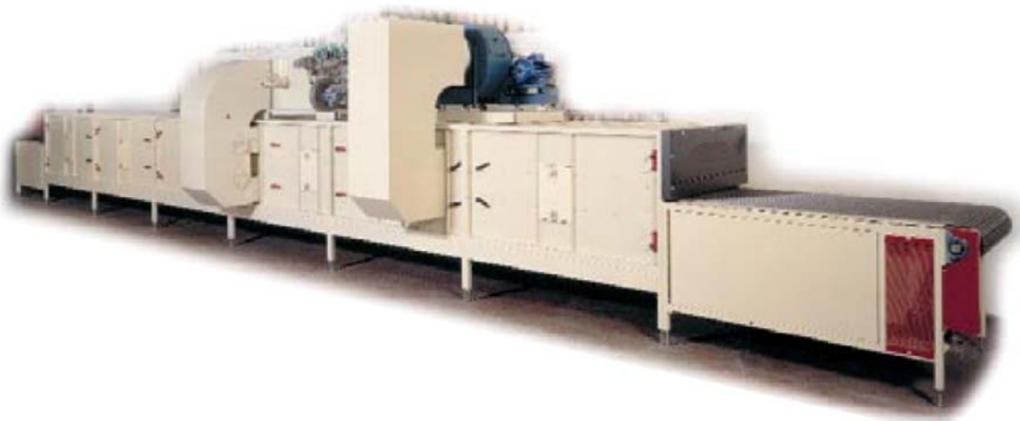
Figure 19b. Pictorial Representation of Press Body Dryer.
