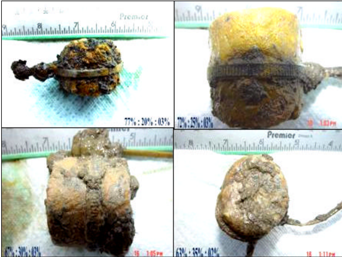
Figure 4. PG:Class C Fly Ash:Portland Type II Cement Briquettes After Nine Months of Submergence.
