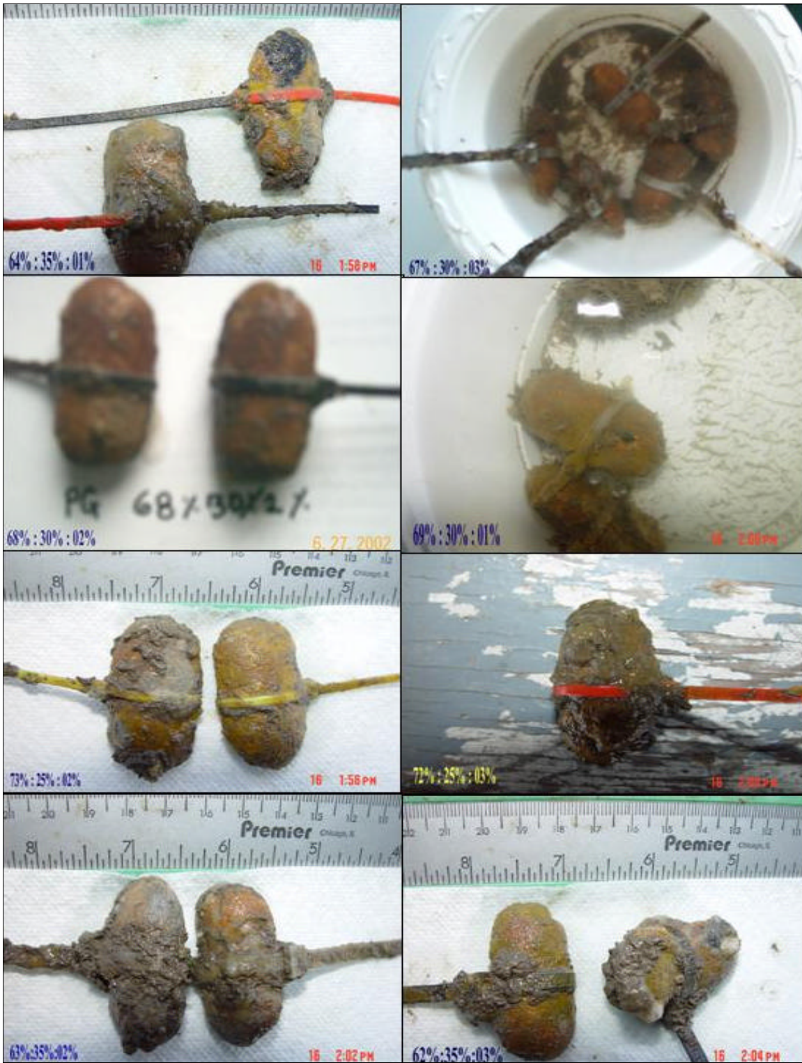
Figure 5. PG:Class C Fly Ash:Portland Type II Cement Composite Briquettes After Four Months of Submergence.
