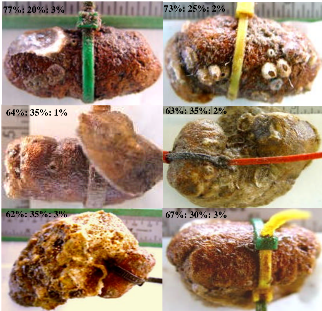
Figure 21. Physical Conditions of the Nine PG Composite Combinations After Fifteen Months of Submergence.
