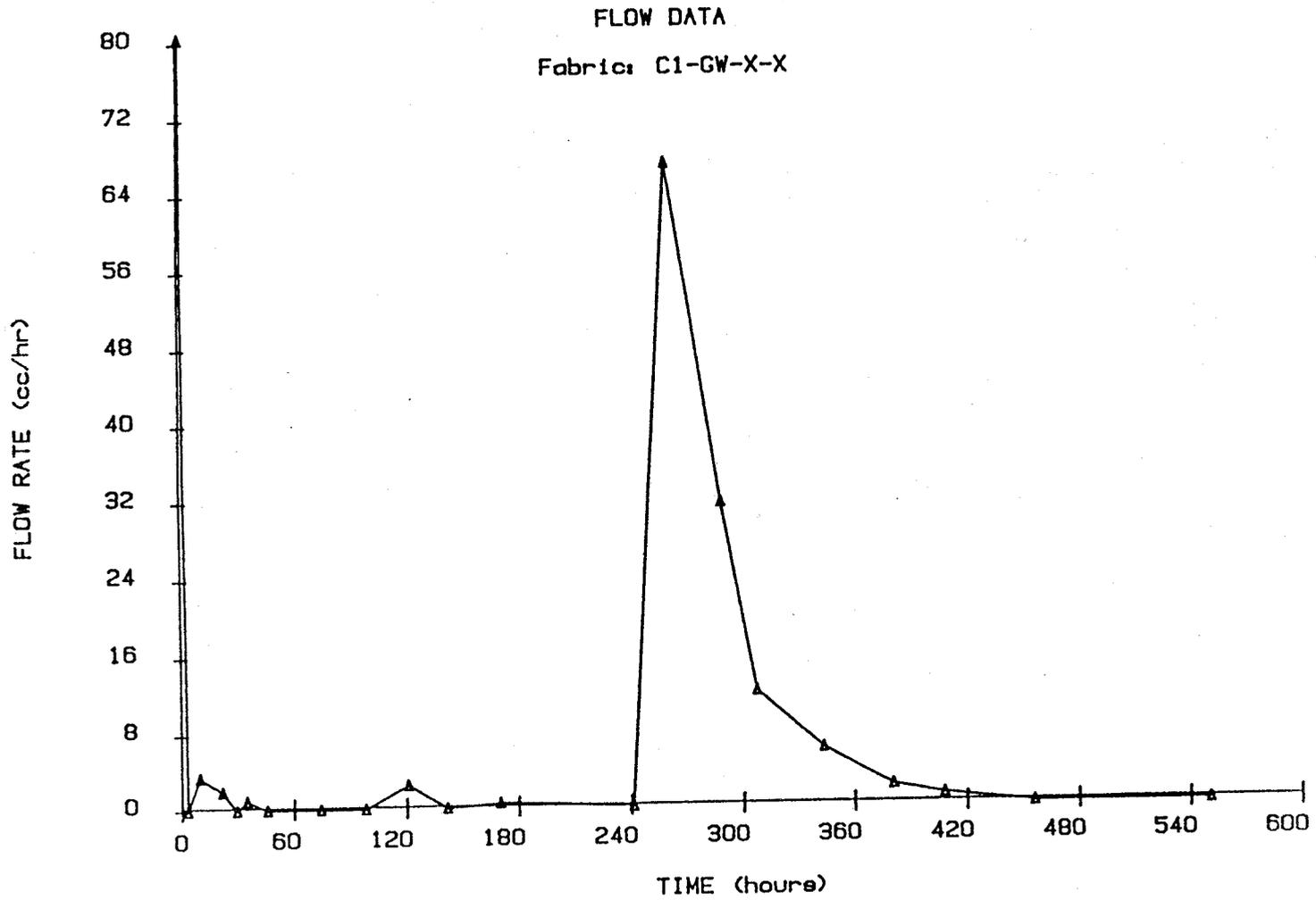
Figure A9: Flow Rate Versus Time for Geotextile C1-GW-X-X
