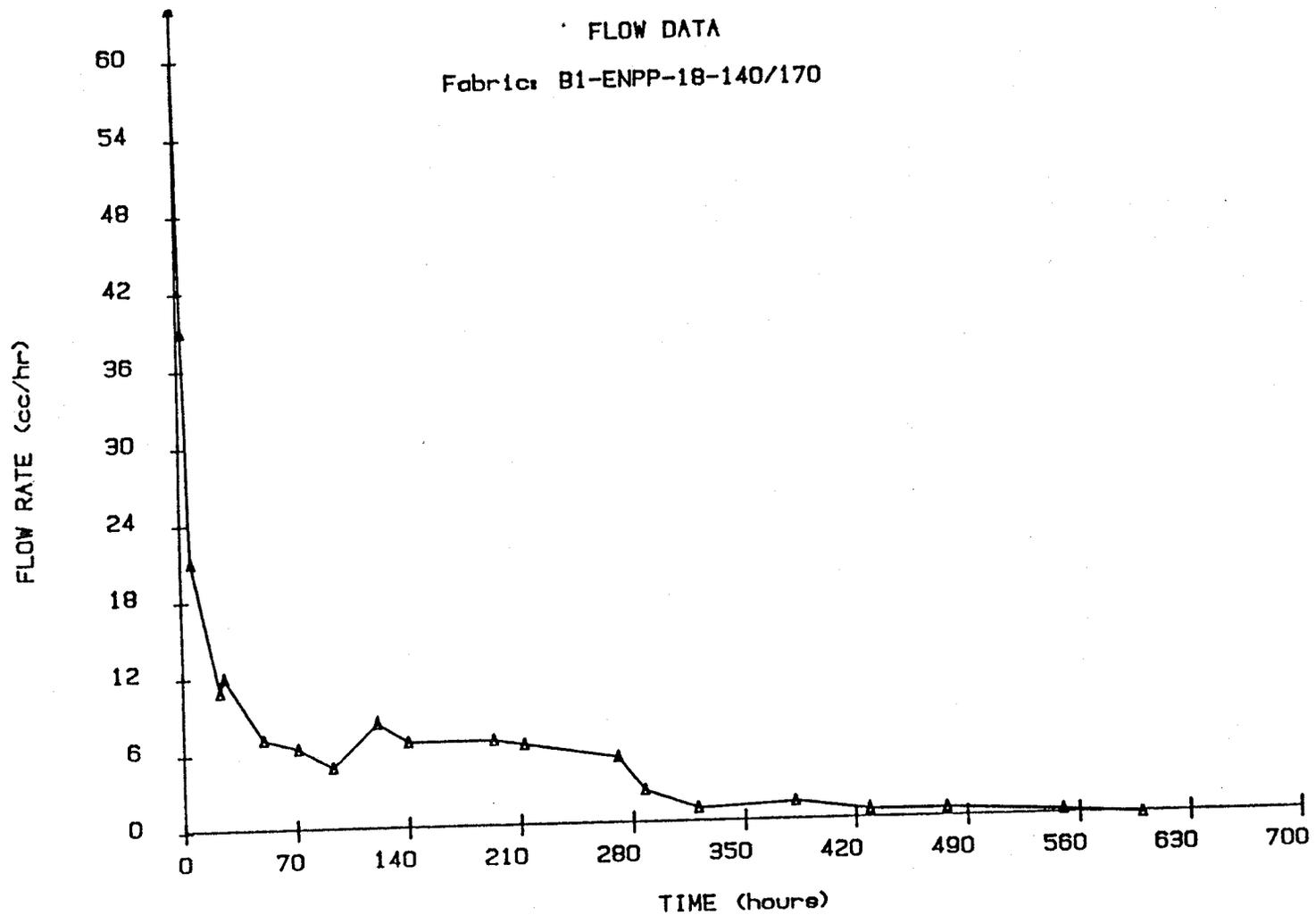
Figure A5: Flow Rate Versus Time for Geotextile B1-ENPP-18-140/170
