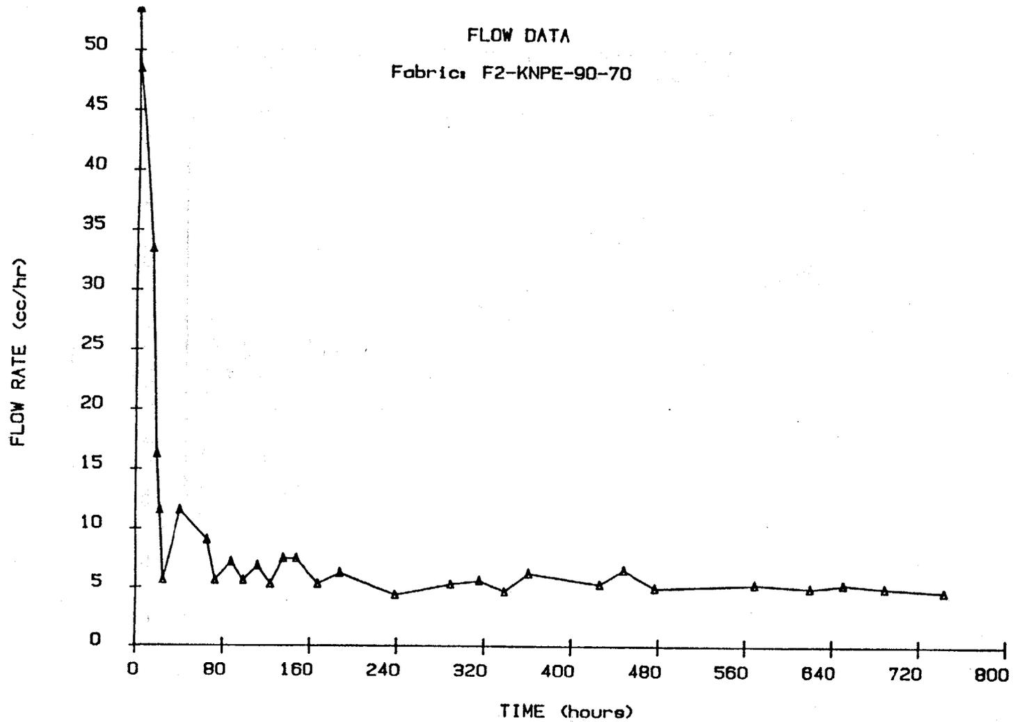
Figure A20: Flow Rate Versus Time for Geotextile F2-KNPE-90-70
