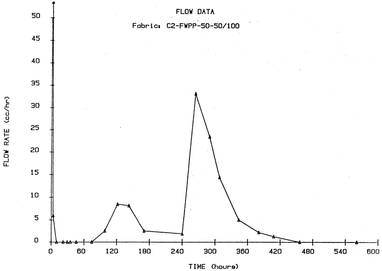
Figure A10: Flow Rate Versus Time for Geotextile C2-FWPP-50-50/100
