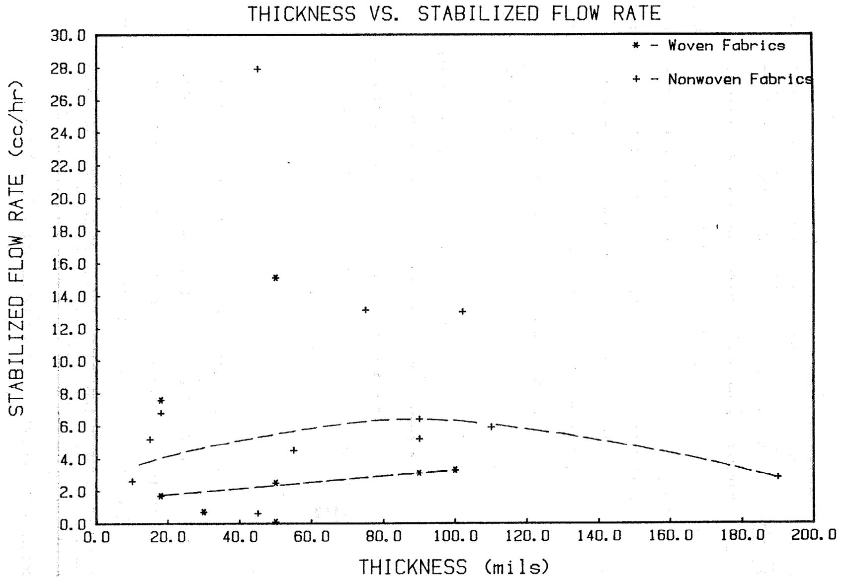
Figure 20: Thickness Versus Stabilized Flow Rate for Woven and Nonwoven Geotextiles
