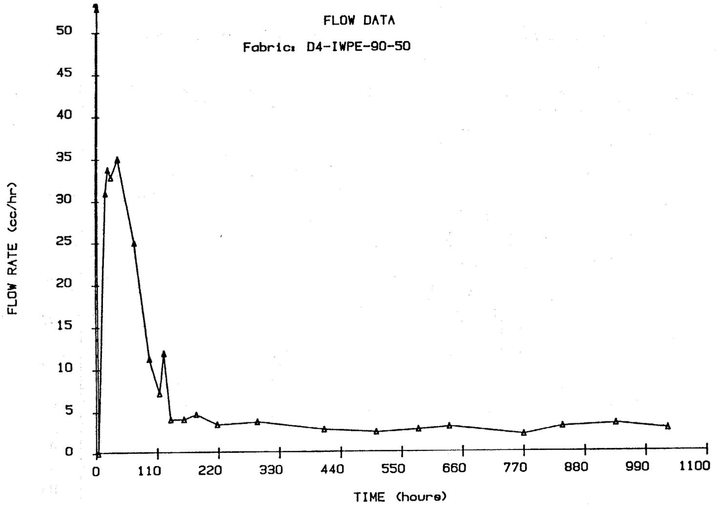
Figure A16: Flow Rate Versus Time for Geotextile D4-IWPE-90-50
