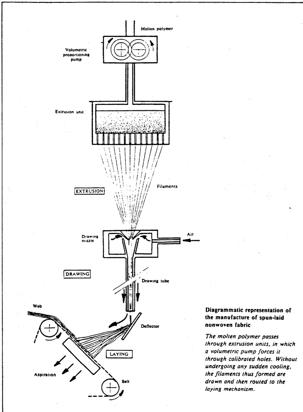
Figure 4: General Manufacturing Process of Spun-Bonded Nonwoven Geotextiles (After Rankilor, 1981)
