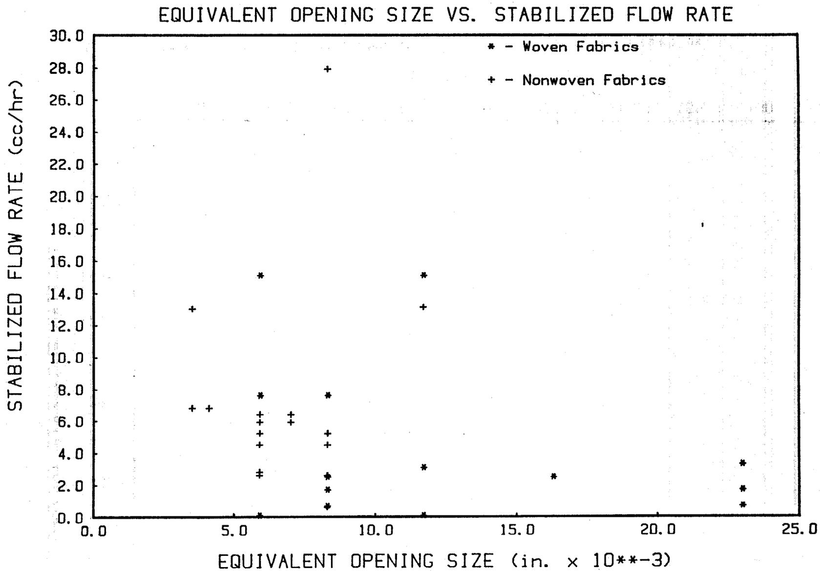
Figure 18: Equivalent Opening Size Versus Stabilized Flow Rate for Woven and Nonwoven Geotextiles
