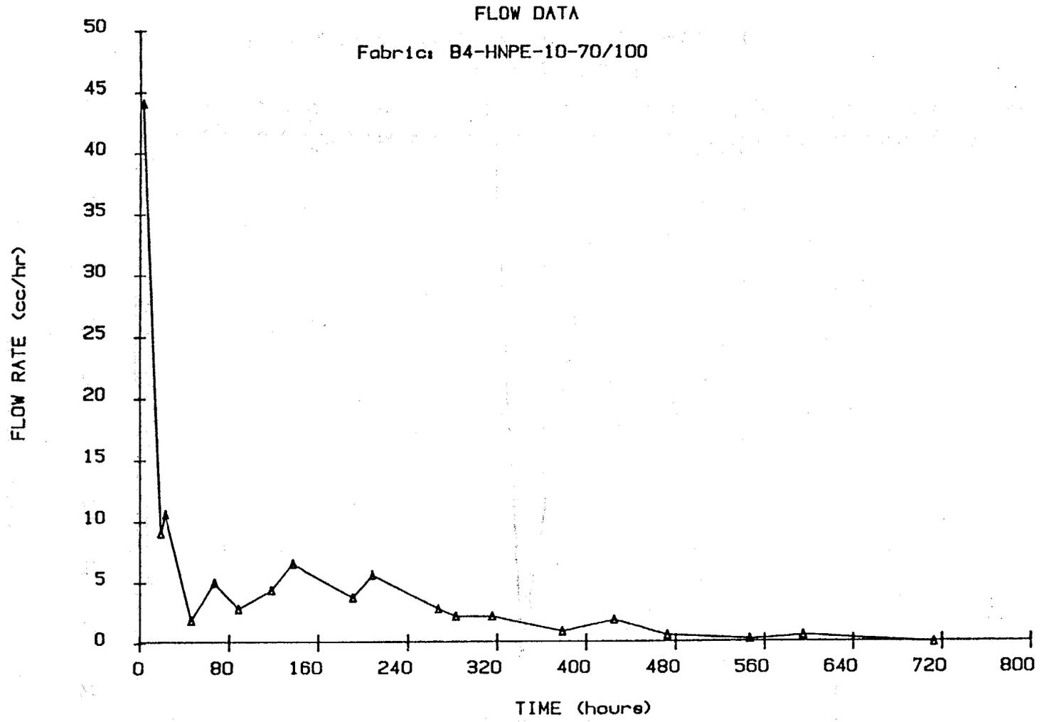
Figure A8: Flow Rate Versus Time for Geotextile B4-HNPE-10-70/100
