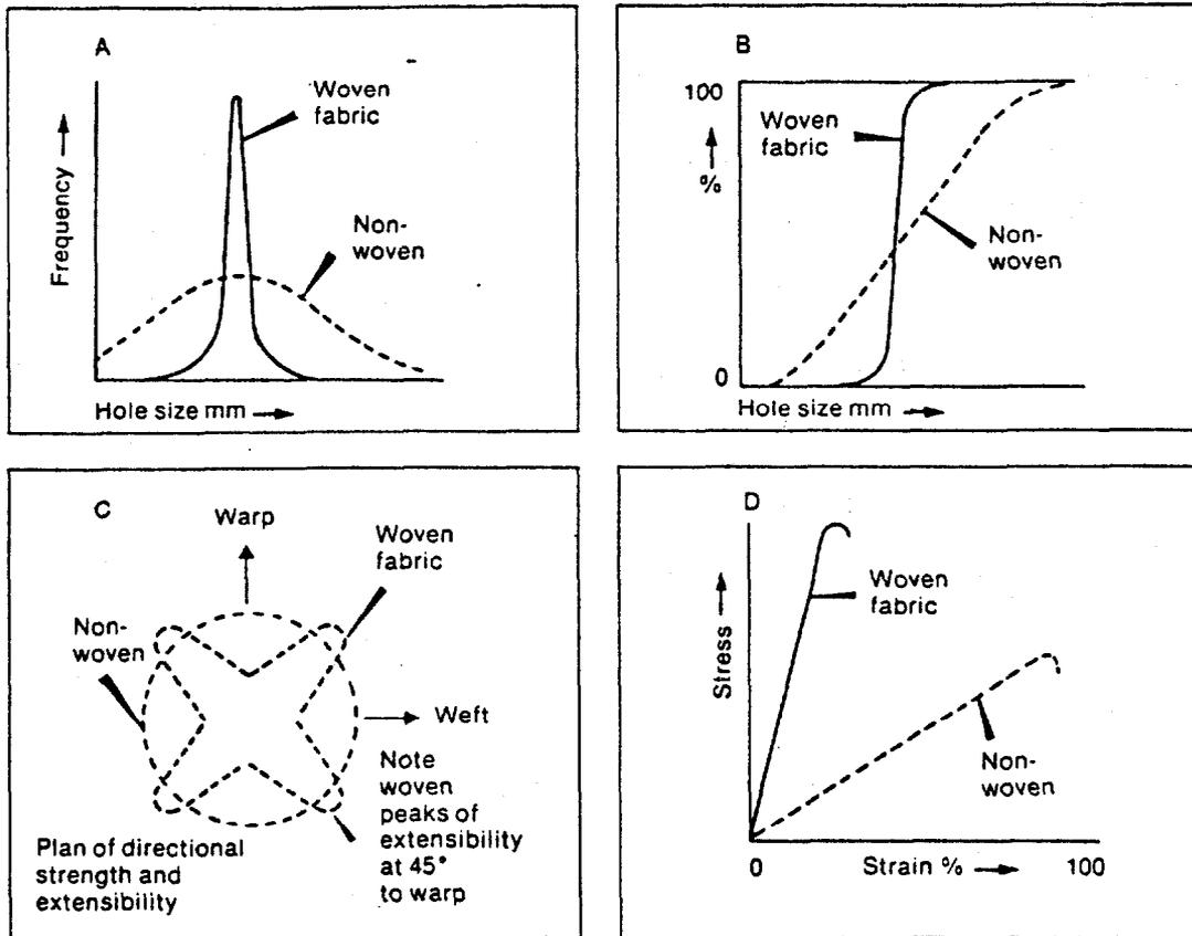
Figure 6: Comparison of Nonwoven and Woven Geotextile Properties (After Rankilor, 1981)
