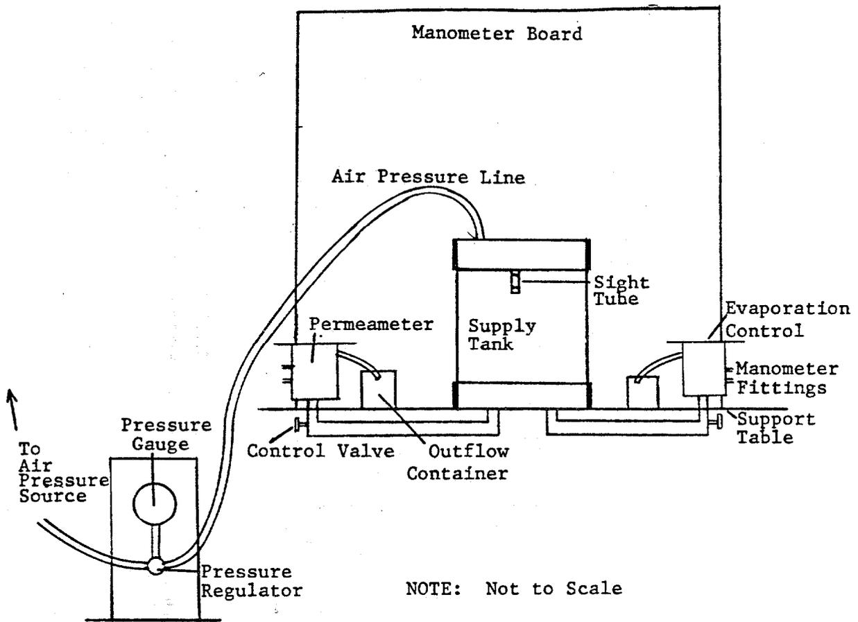
Figure 15: Schematic Diagram of Flow Rate Test Apparatus
