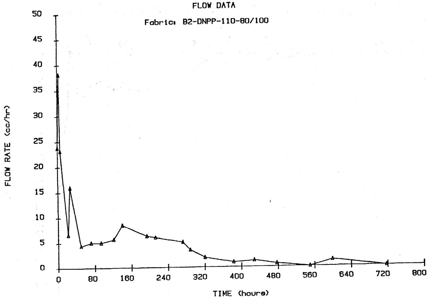
Figure A6: Flow Rate Versus Time for Geotextile B2-DNPP-110-80/100
