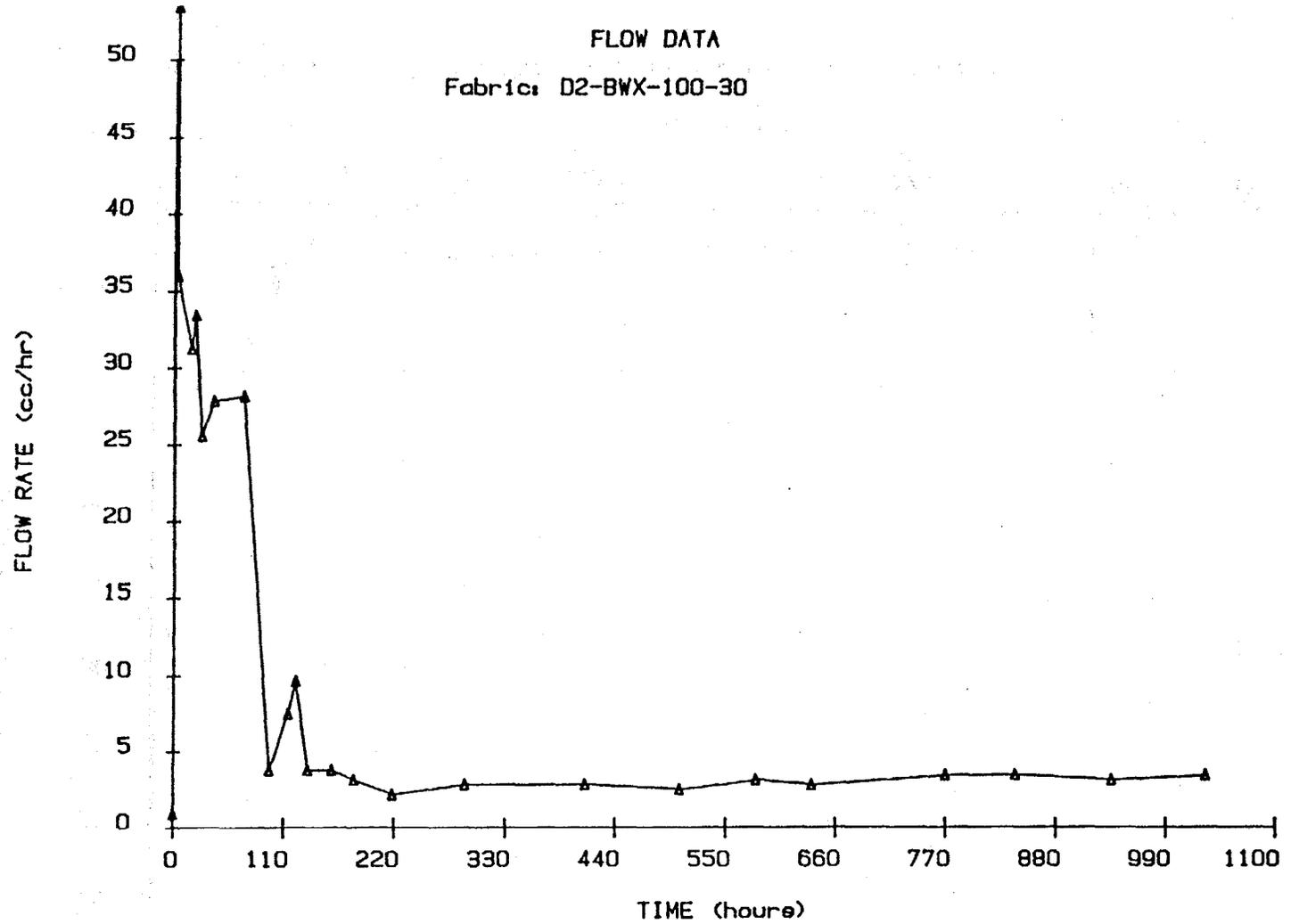
Figure A14: Flow Rate Versus Time for Geotextile D2-BWX-100-30
