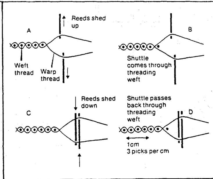
Figure 3: General Manufacturing Process of Woven Geotextiles
