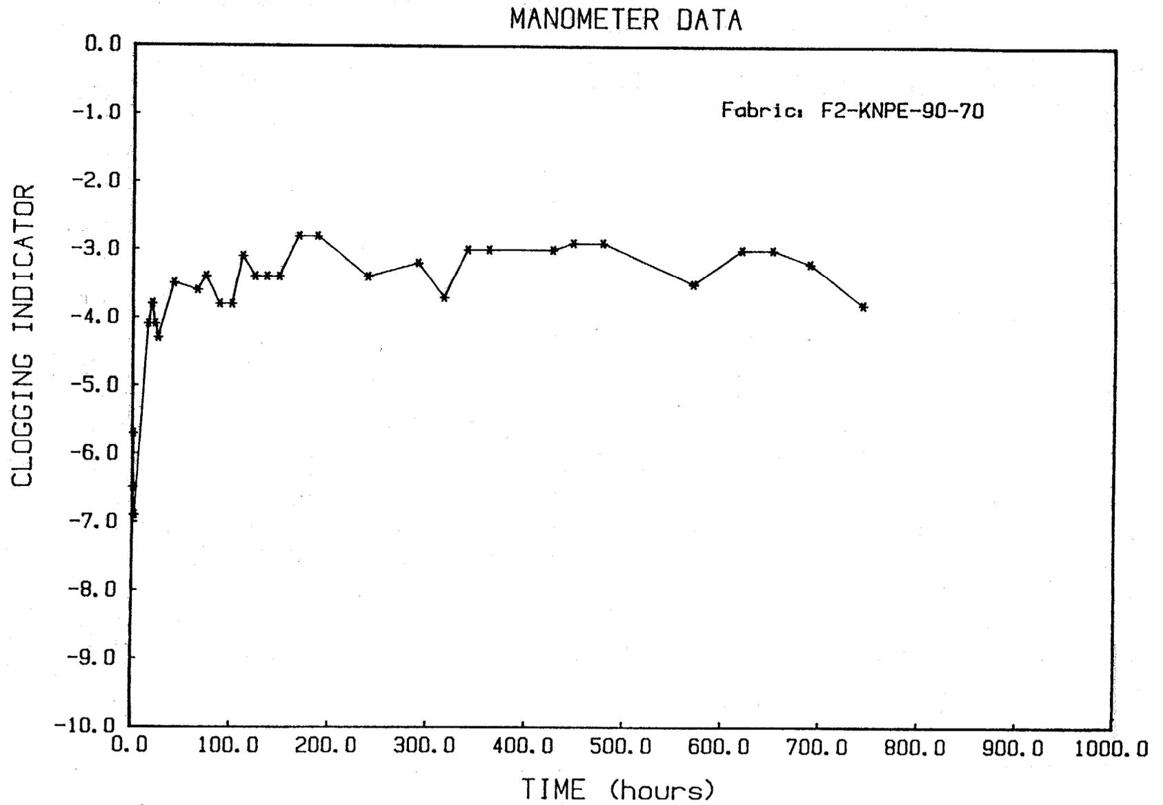
Figure B4: Clogging Indicator Versus Time for Geotextile F2-KNPE-90-70
