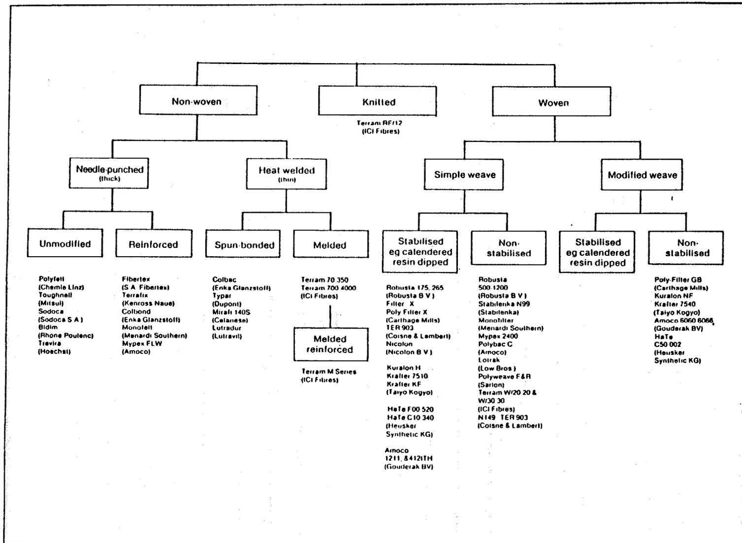
Figure 2: Geotextile Types Based on Manufacturing Process (After Rankilor, 1981)
