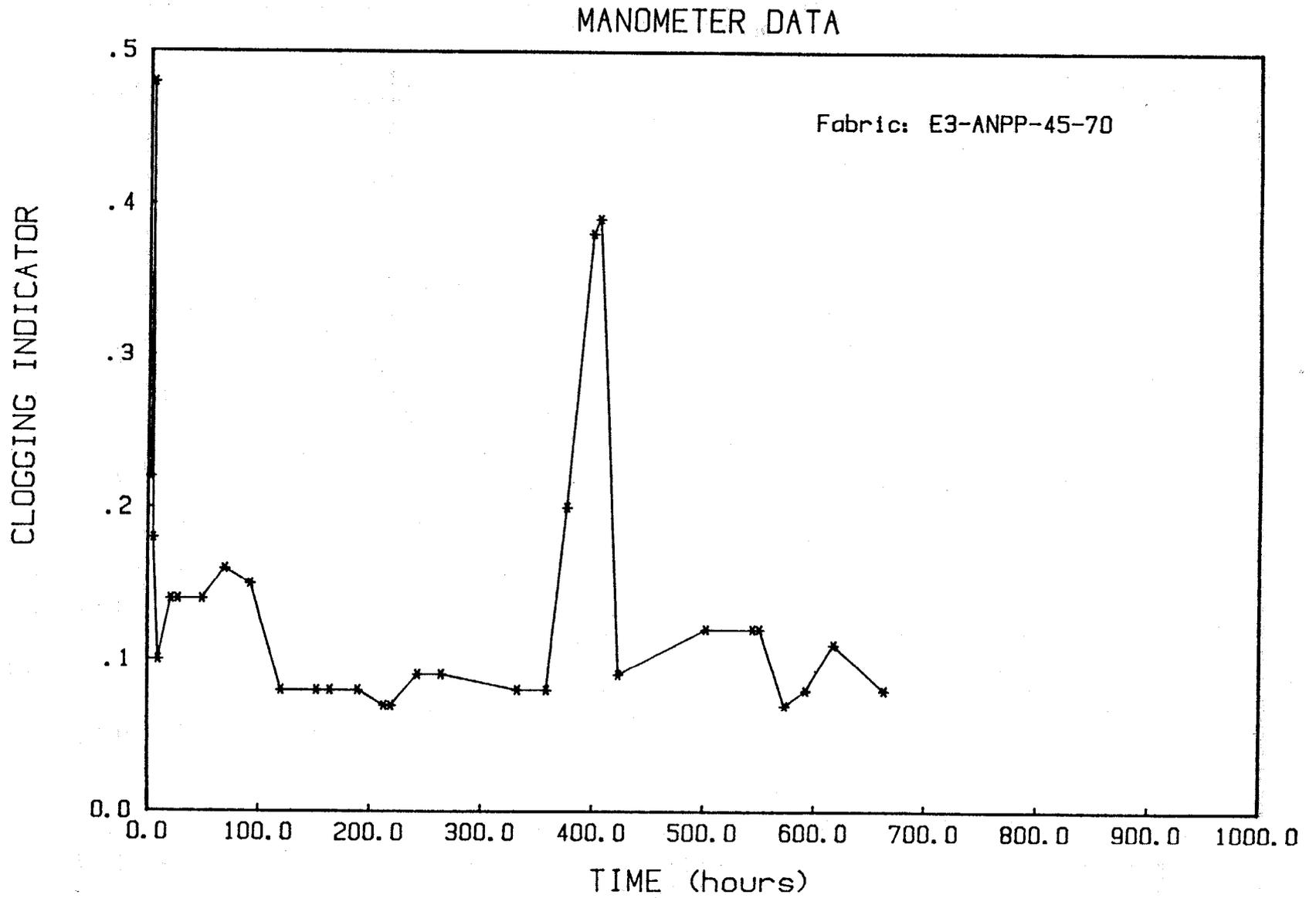
Figure B2: Clogging Indicator Versus Time for Geotextile E3-ANPP-45-70
