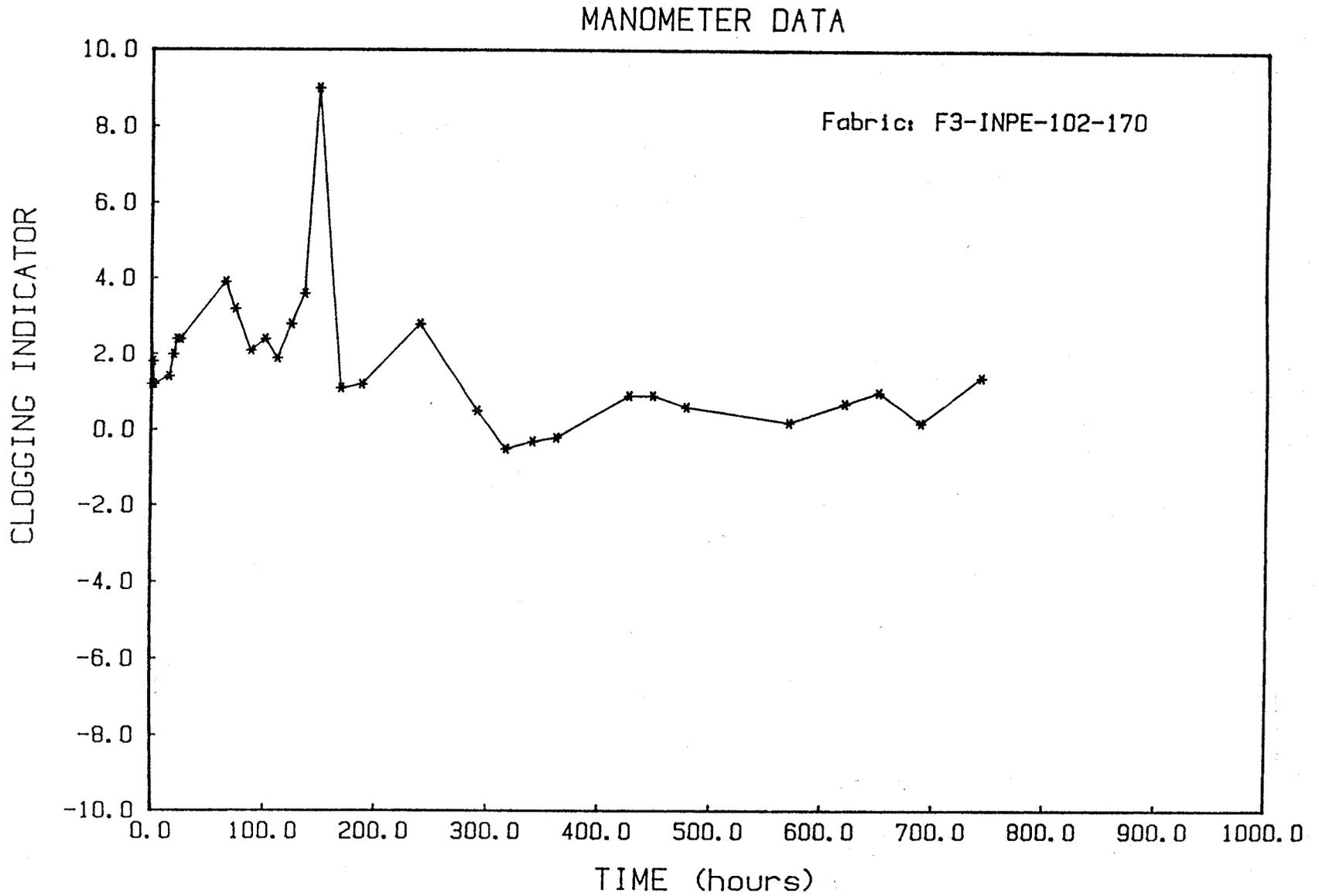
Figure B5: Clogging Indicator Versus Time for Geotextile F3-INPE-102-170
