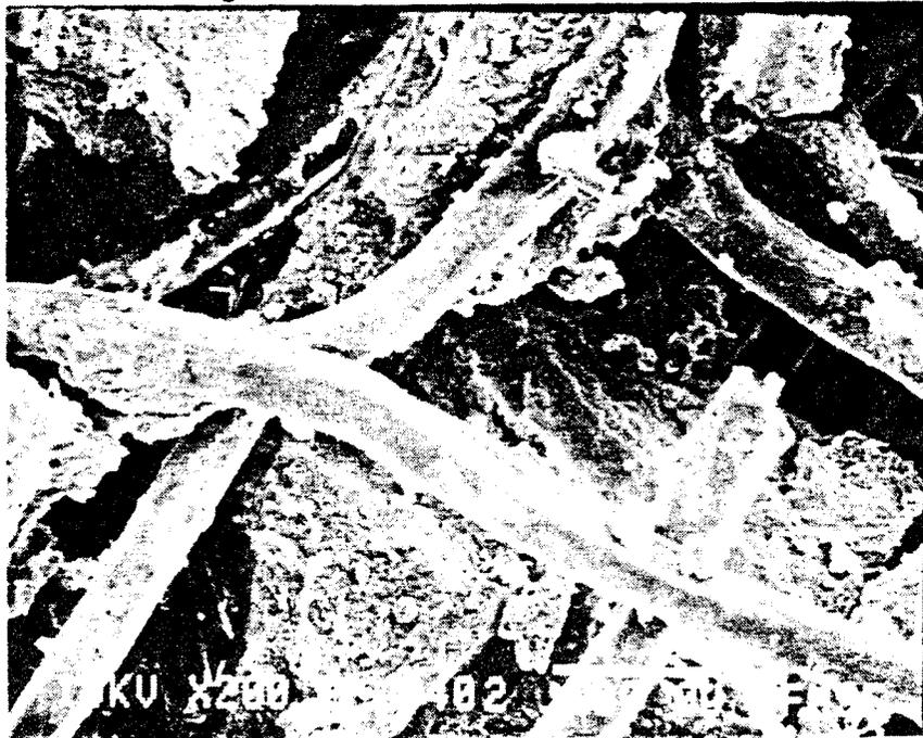
Figure C1: Scanning Electron Microphotographs, Before and After Testing, for Geotextile A4-JNPP-90-60/100.
