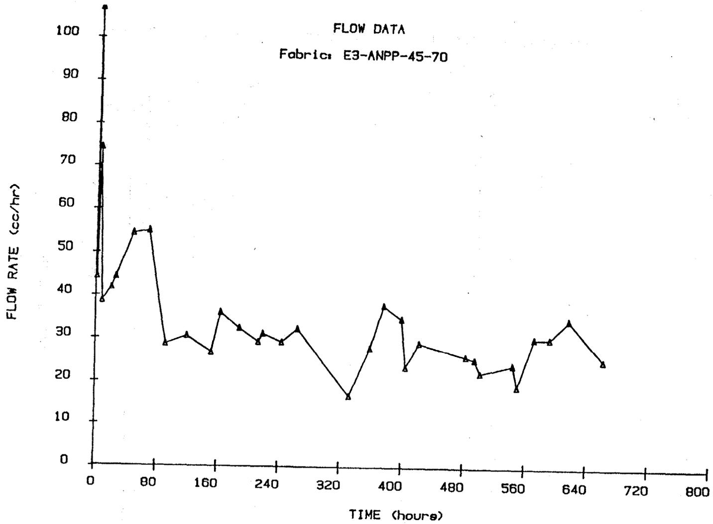
Figure A18: Flow Rate Versus Time for Geotextile E3-ANPP-45-70
