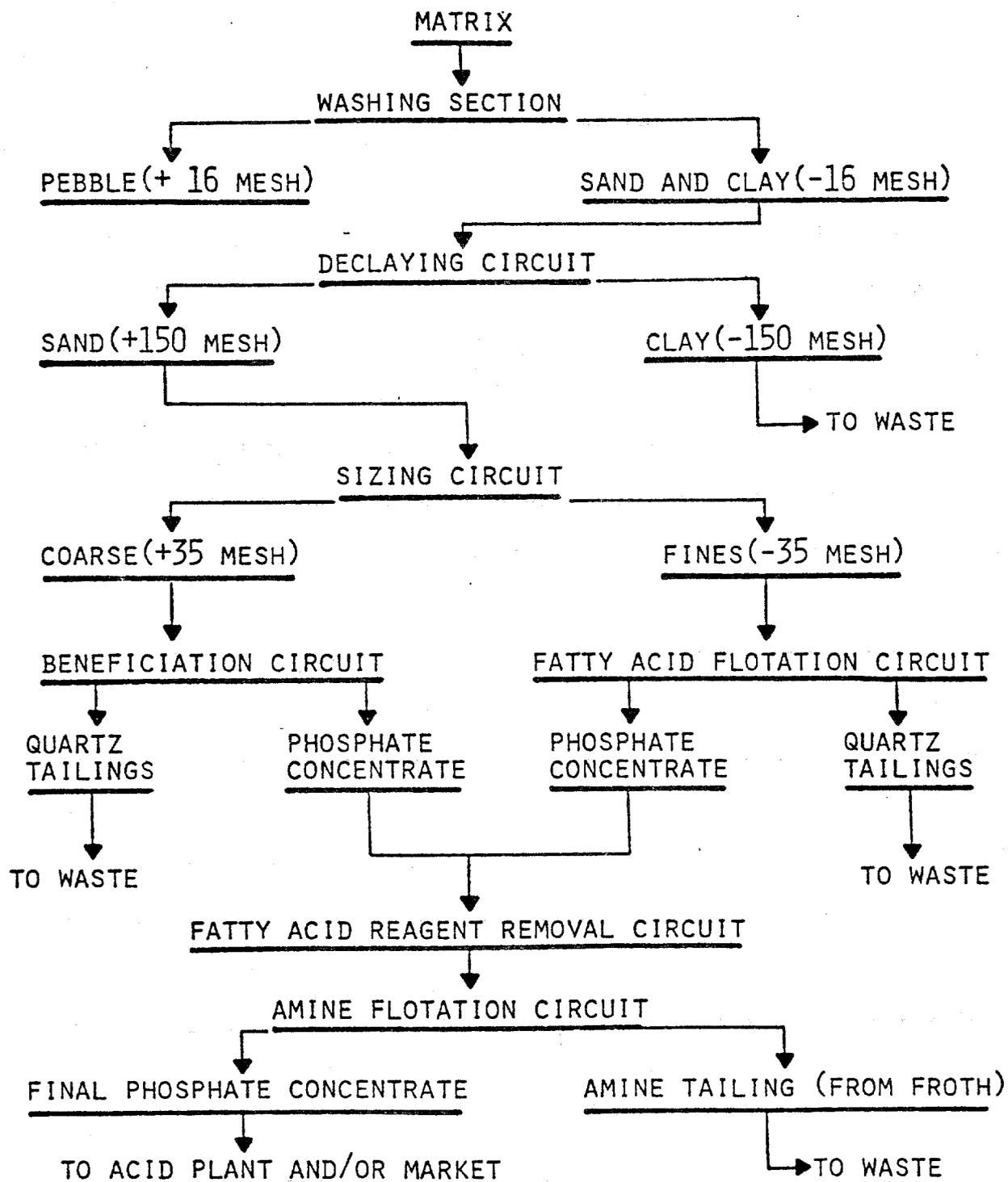
Figure 1: Generalized Phosphate Beneficiation Flow Diagram
