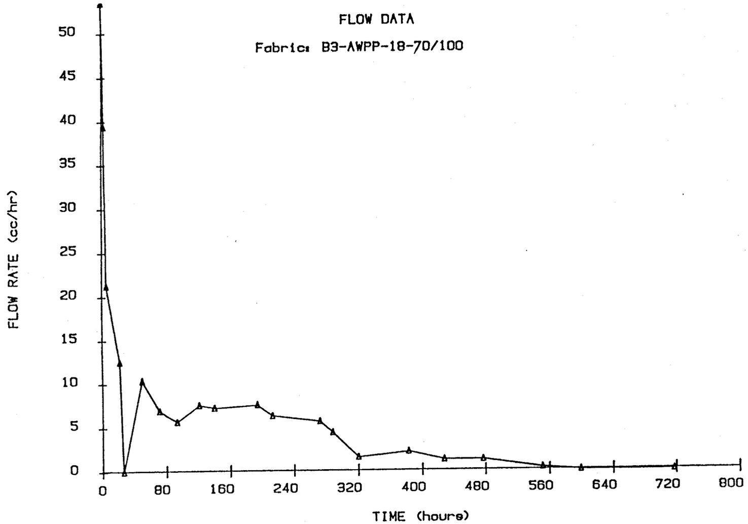
Figure A7: Flow Rate Versus Time for Geotextile B3-AWPP-18-70/100
