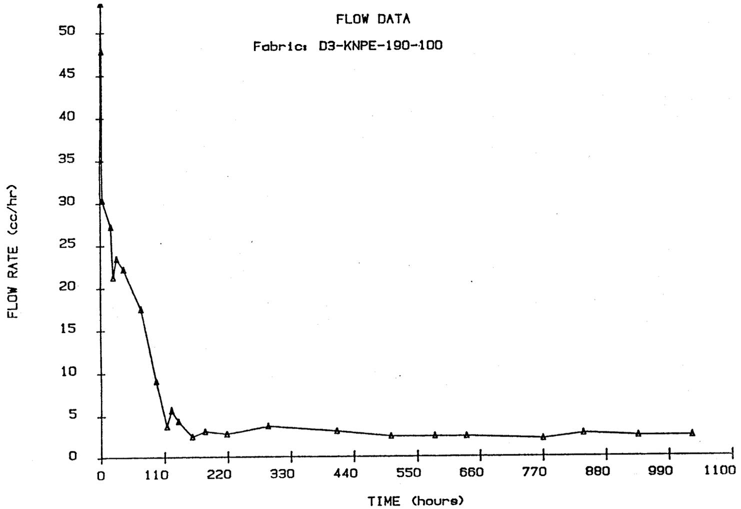
Figure A15: Flow Rate Versus Time for Geotextile D3-KNPE-190-100
