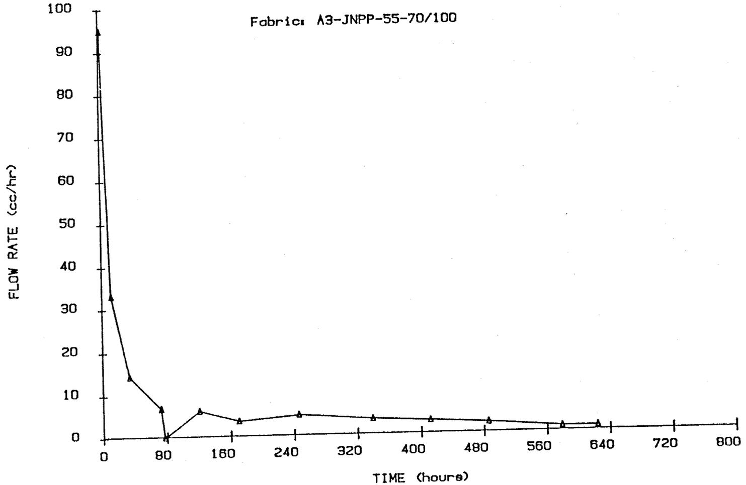
Figure A3: Flow Rate Versus Time for Geotextile A3-JNPP-55-70/100
