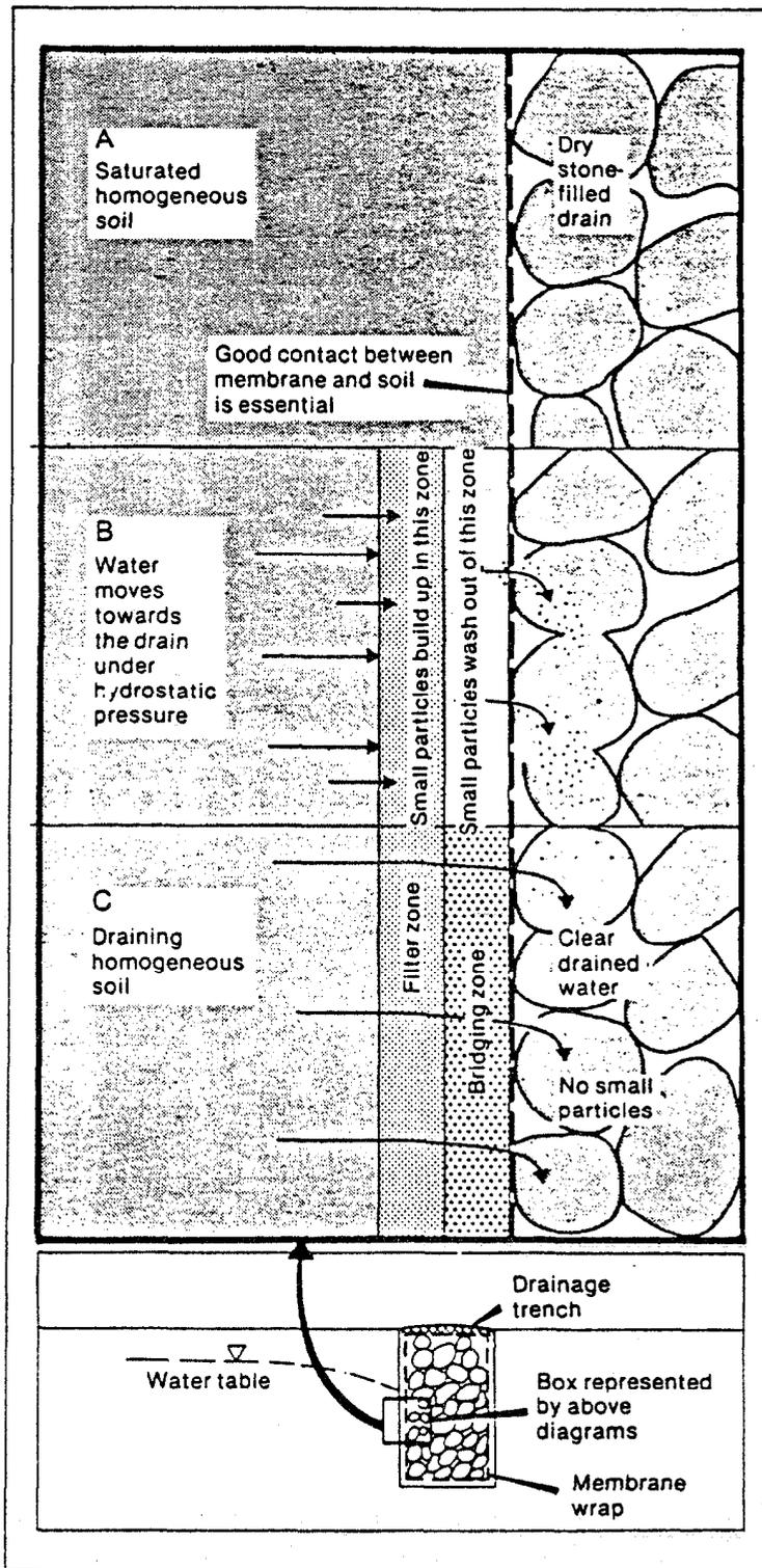
Figure 8: Development of an Internal Soil Filter Behind a Geotextile (After Rankilor, 1981)
