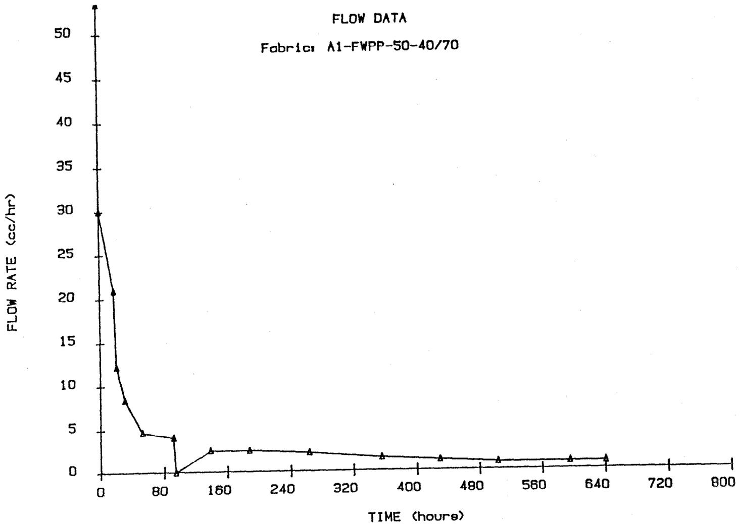
Figure A1: Flow Rate Versus Time for Geotextile A1-FWPP-50-40/70
