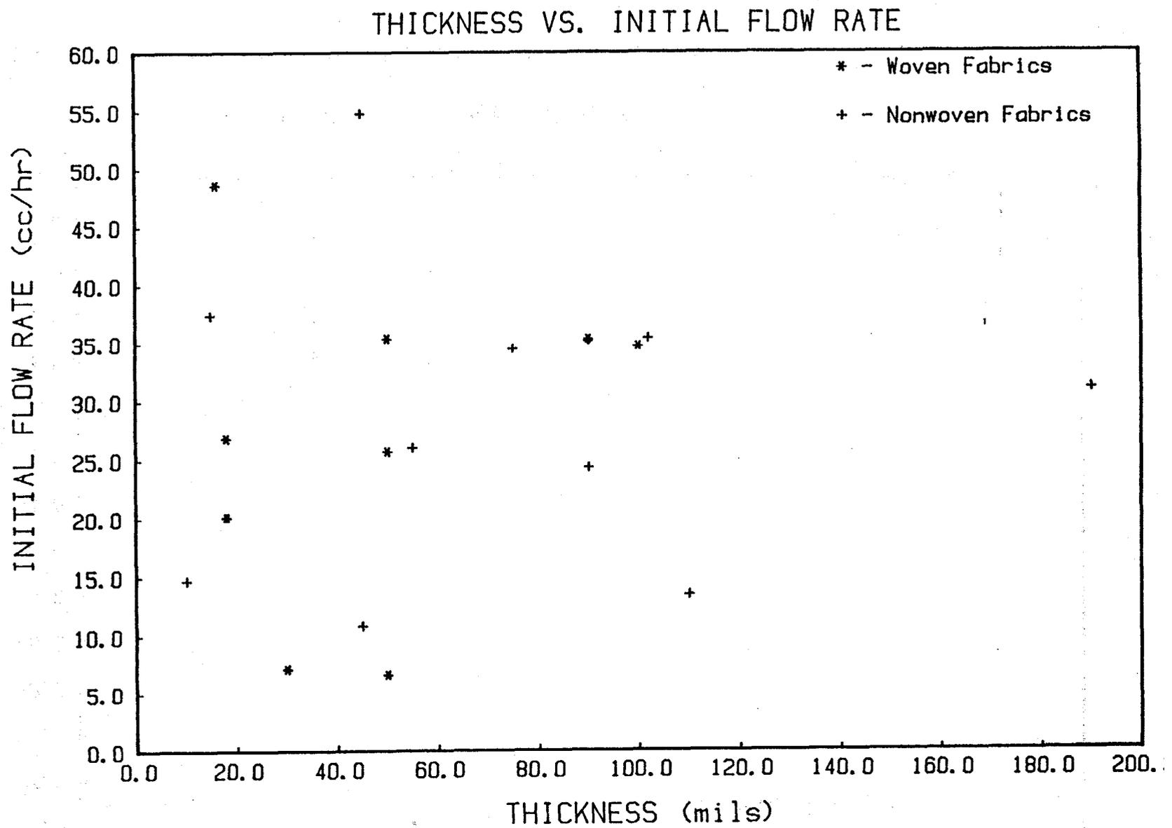
Figure 19: Thickness Versus Initial Flow Rate for Woven and Nonwoven Geotextiles
