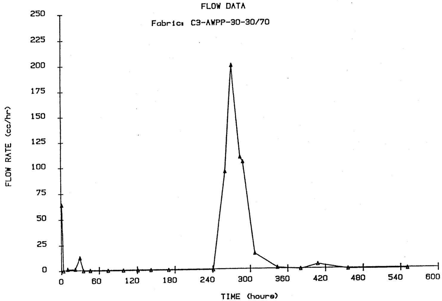
FigureAll: Flow Rate Versus Time for Geotextile C3-AWPP-30-30/70
