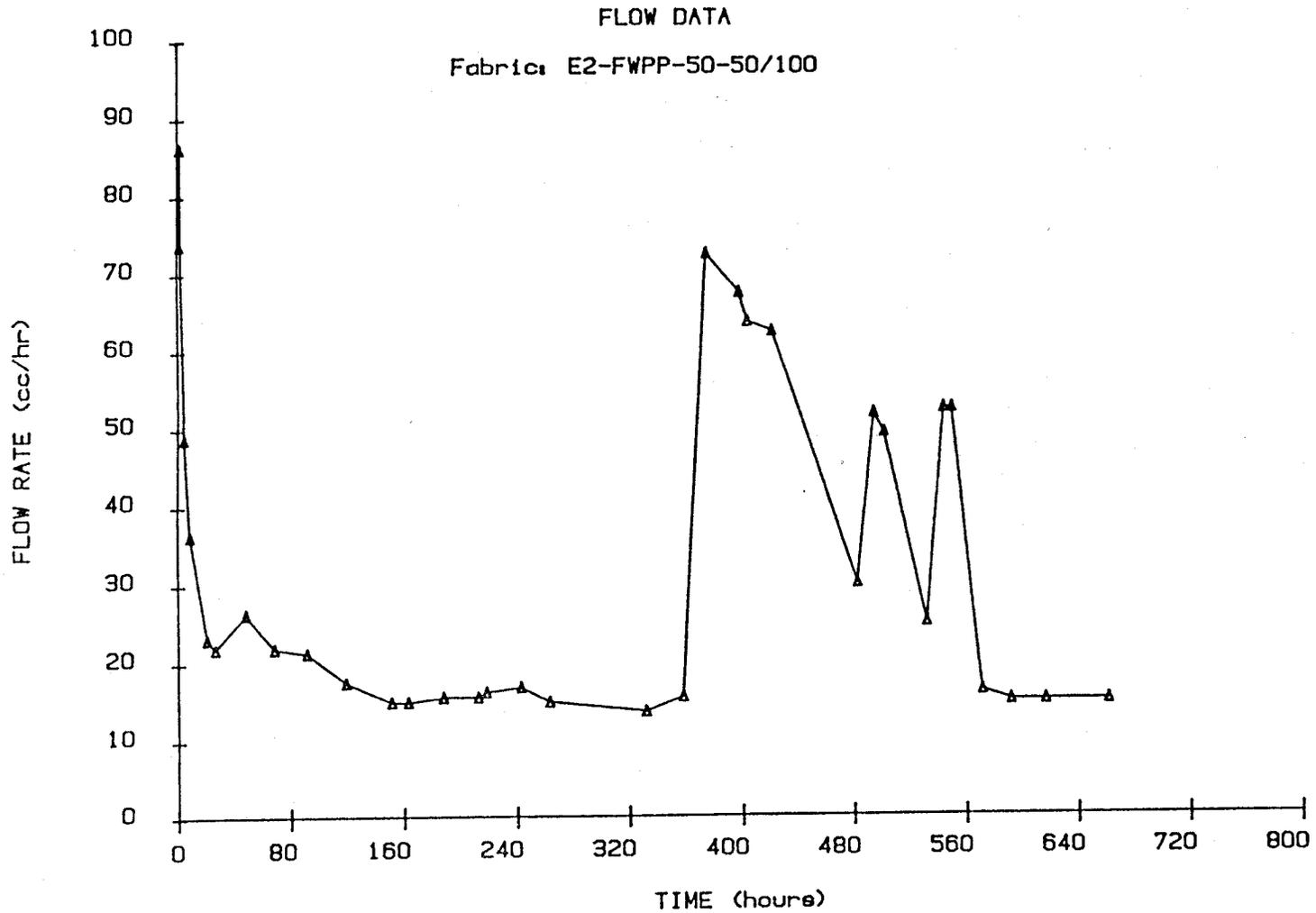
Figure A17: Flow Rate Versus Time for Geotextile E2-FWPP-50-50/100
