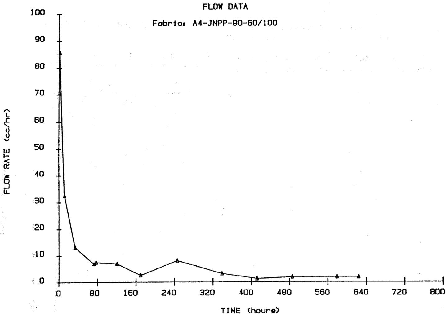
Figure A4: Flow Rate Versus Time for Geotextile A4-JNPP-90-60/100
