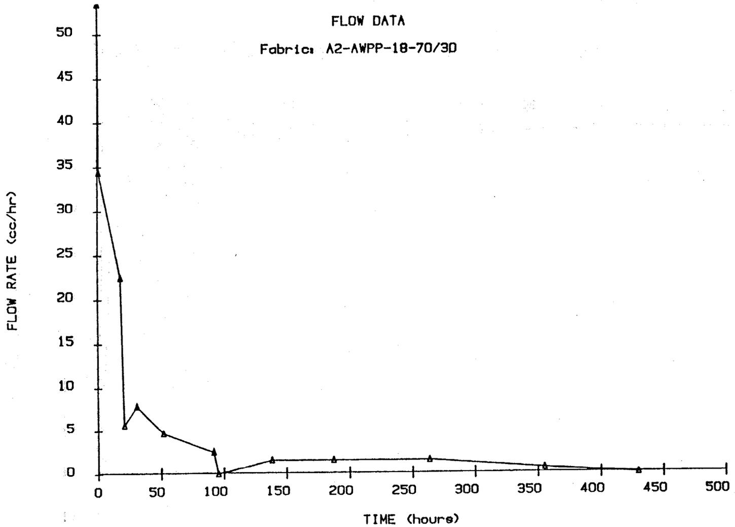
Figure A2: Flow Rate Versus Time for Geotextile A2-AWPP-18-70/30
