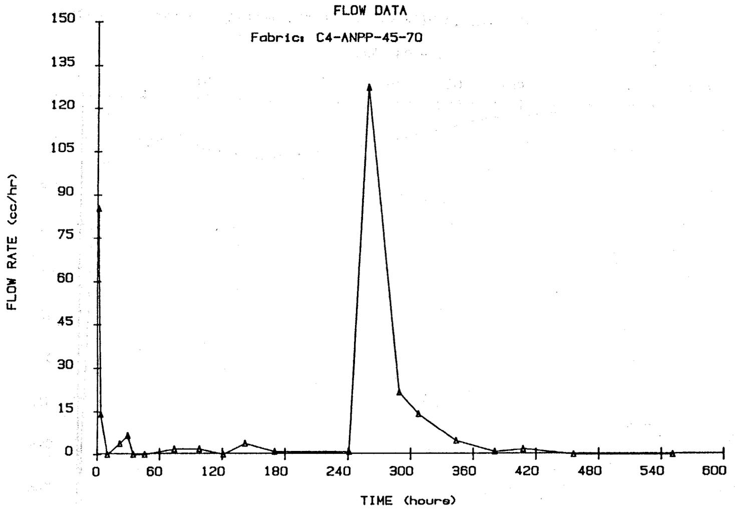
Figure A12: Flow Rate Versus Time for Geotextile C4-ANPP-45-70
