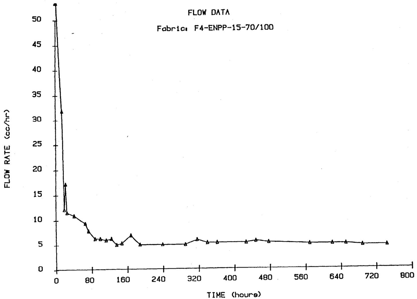
Figure A22: Flow Rate Versus Time for Geotextile F4-ENPP-15-70/100
