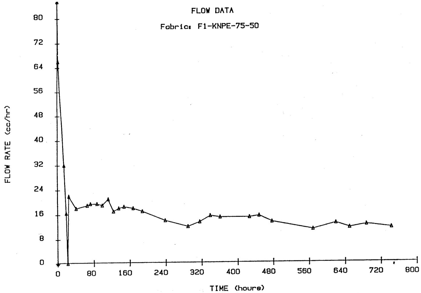
Figure A19: Flow Rate Versus Time for Geotextile F1-KNPE-75-50
