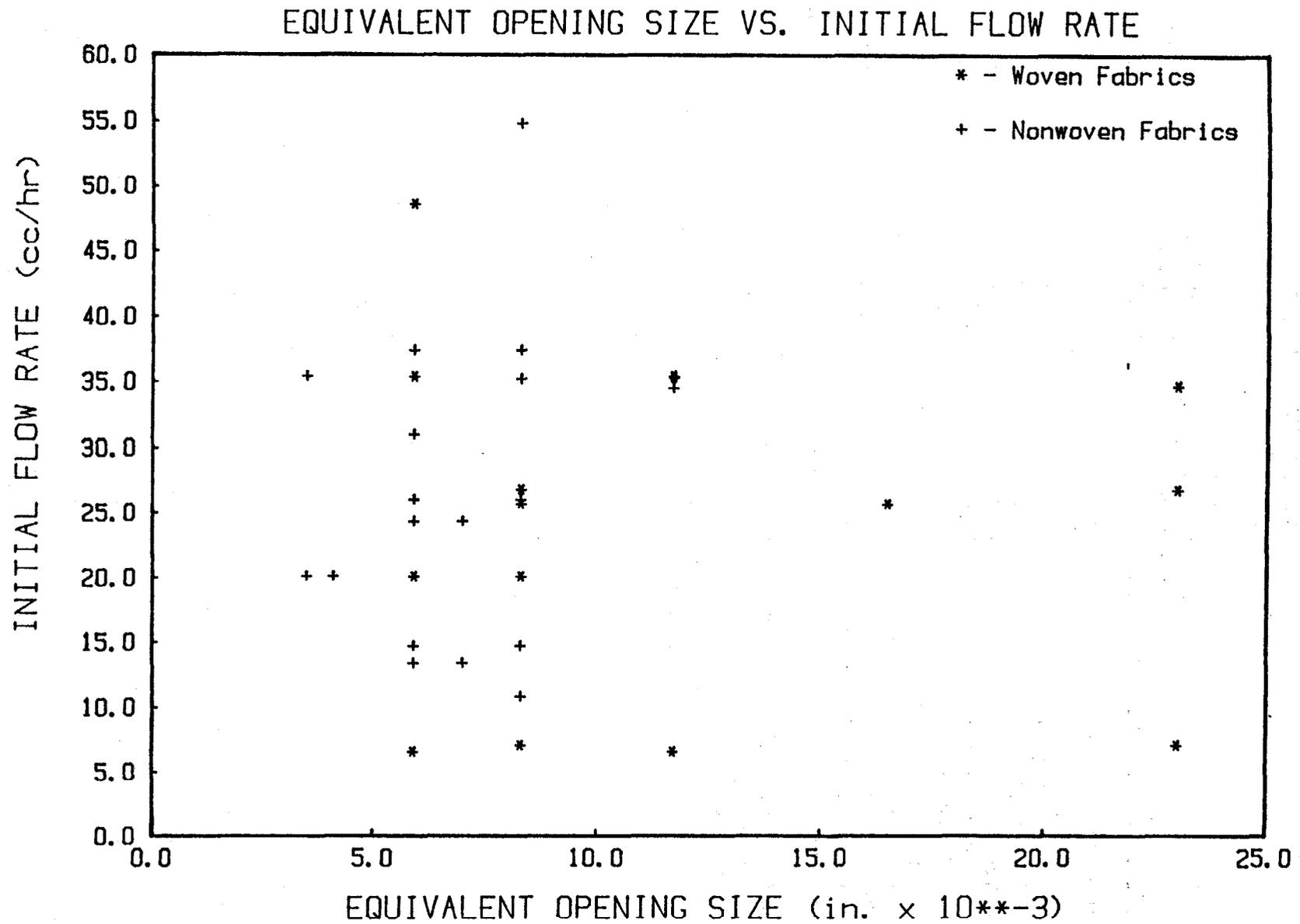
Figure 17: Equivalent Opening Size Versus Initial Flow Rate for Woven and Nonwoven Geotextiles
