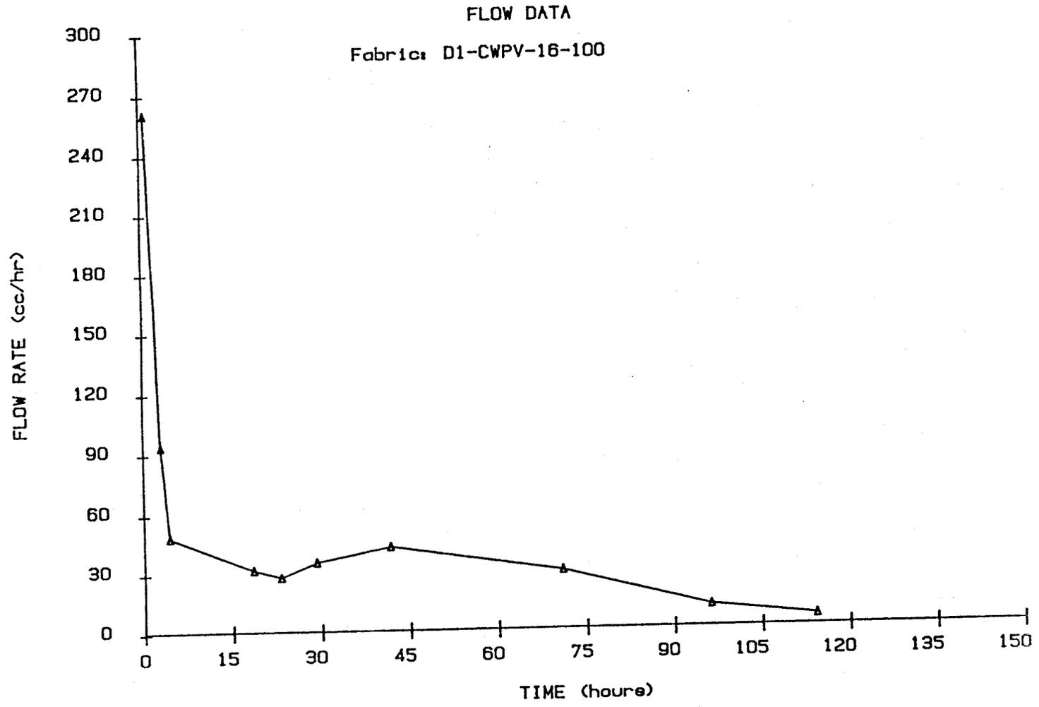
Figure A13: Flow Rate Versus Time for Geotextile D1-CWPV-16-100
