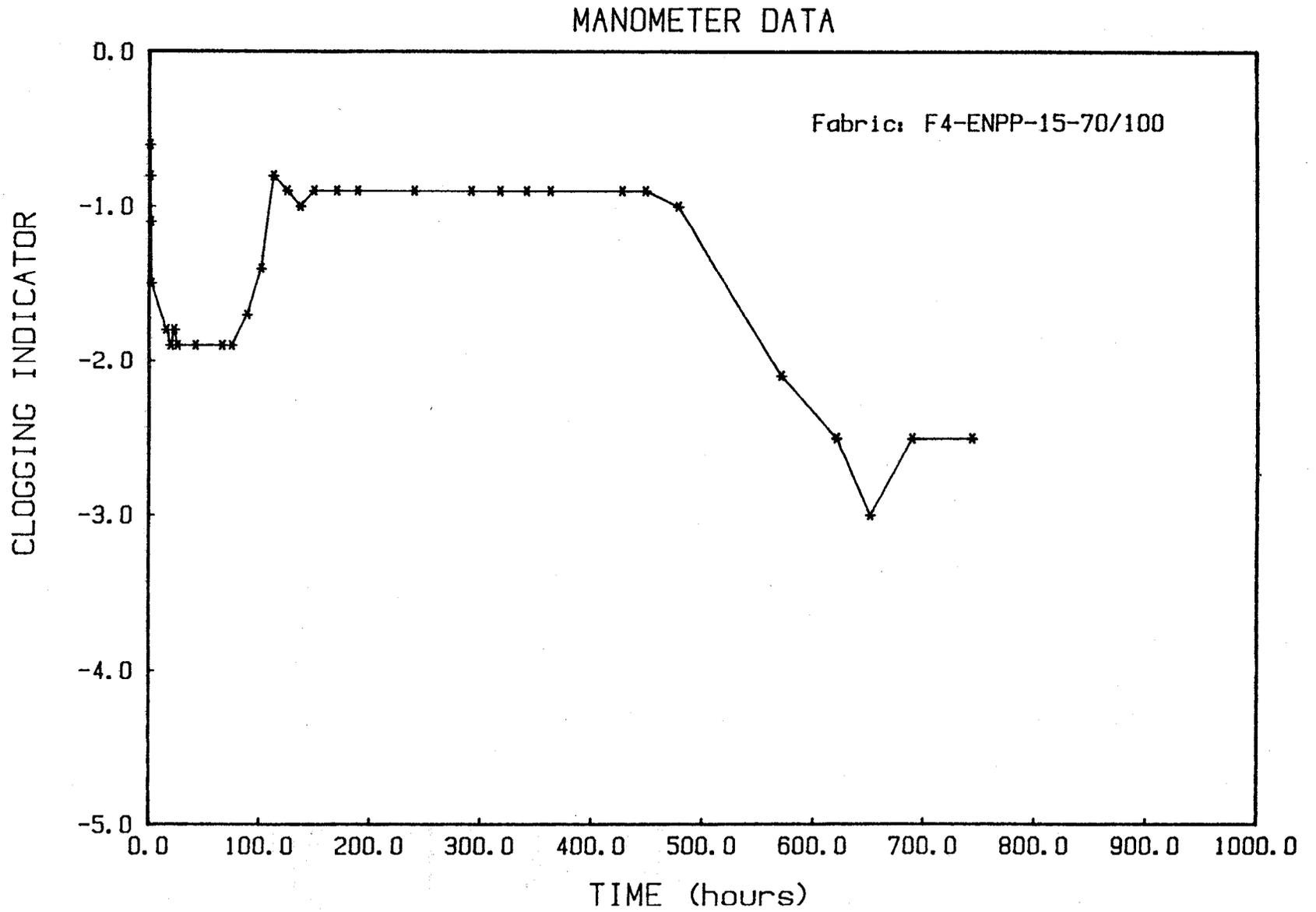
Figure B6: Clogging Indicator Versus Time for Geotextile F4-ENPP-15-70/100
