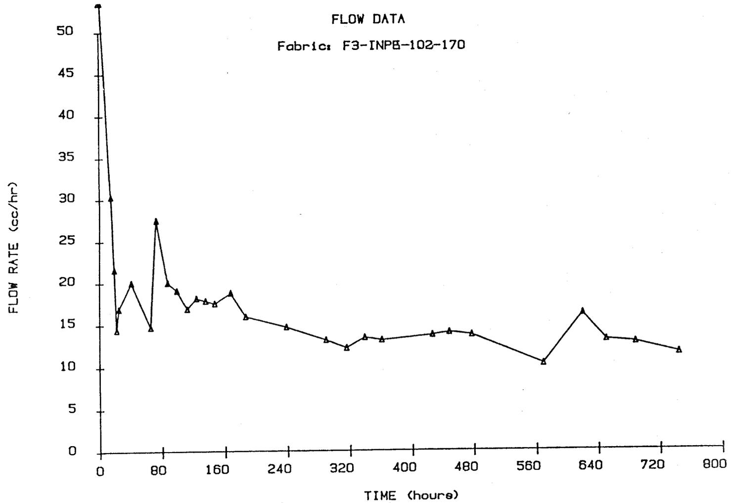
Figure A21: Flow Rate Versus Time for Geotextile F3-INPE-102-170
