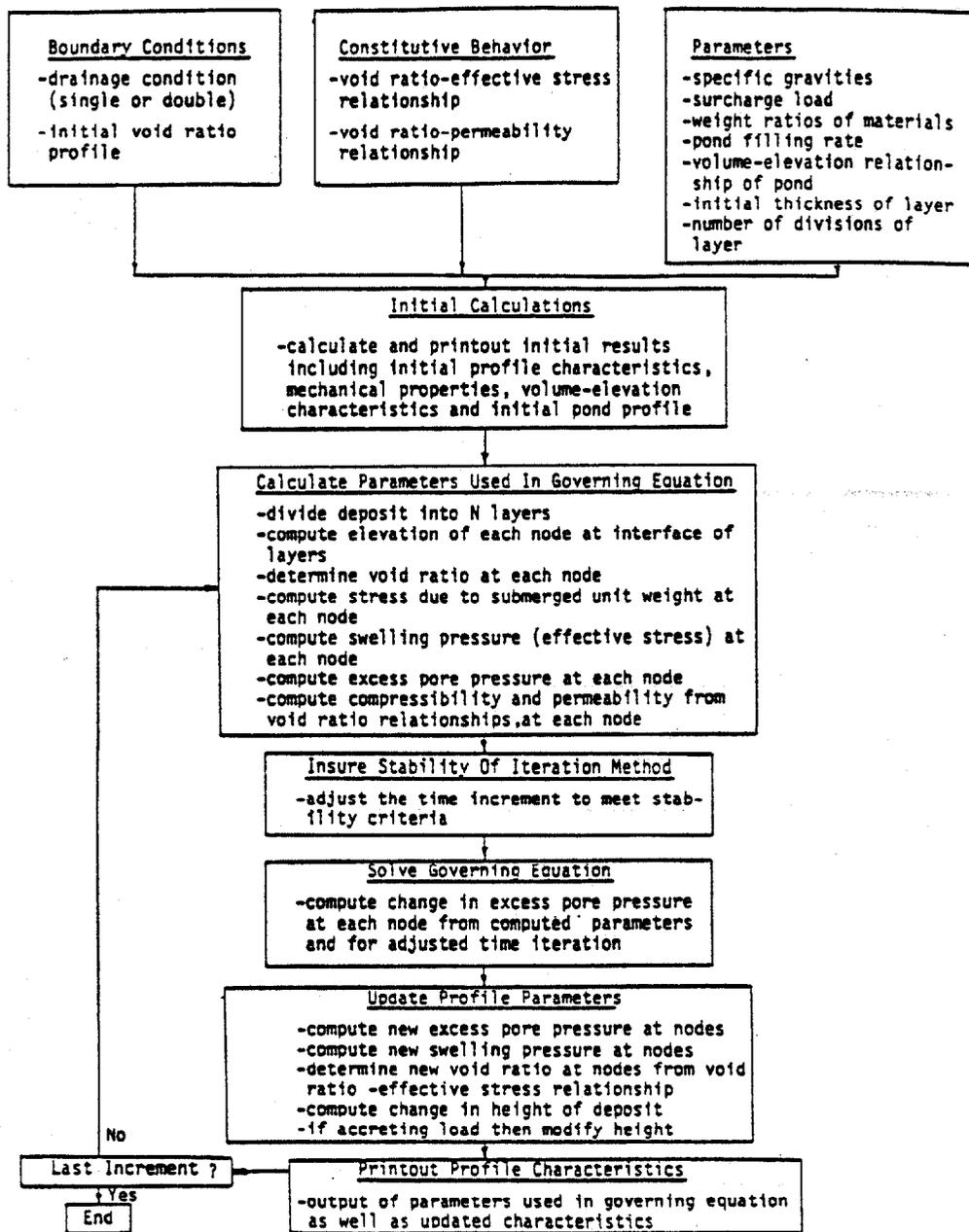
Figure 4.5. Computational Flow Scheme of Yong's Model (Yong and Ludwig, 1984).
