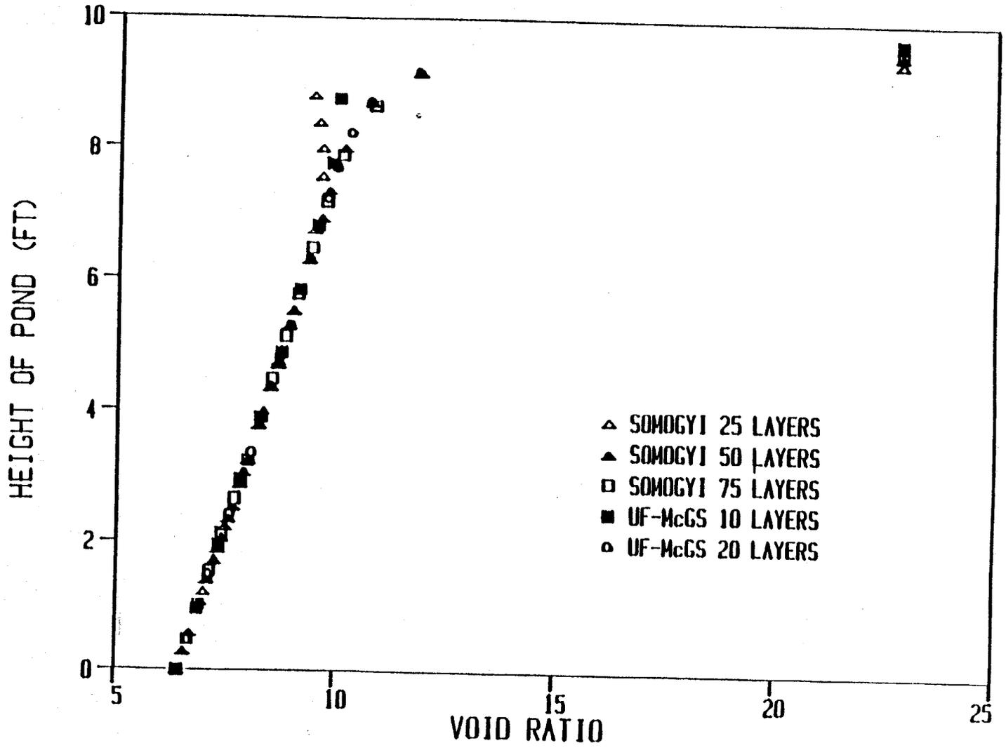
Figure 6.3. Void Ratio Profile after 1 Year for Pond 1a.
