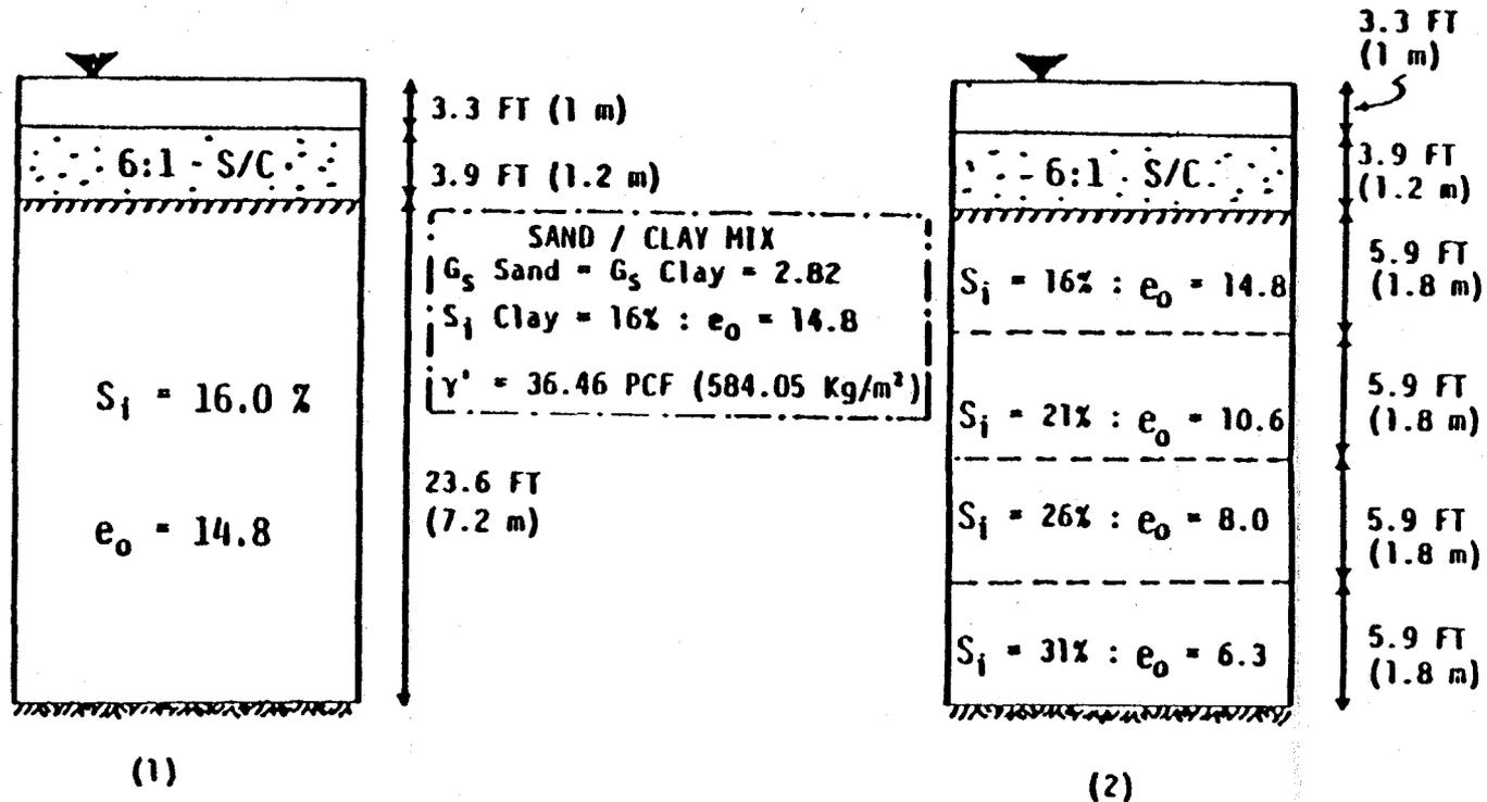
Figure 6.30. Two Layer Quiescent Consolidation: (1) Pond 4a. Uniform Void Ratio (Sand/Clay Cap Surcharge) (2) Pond 4b. Variable Void Ratio
