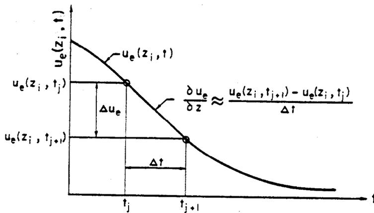
b) - Secant to The Excess Pore Pressure Function at Depth  $z_i$
