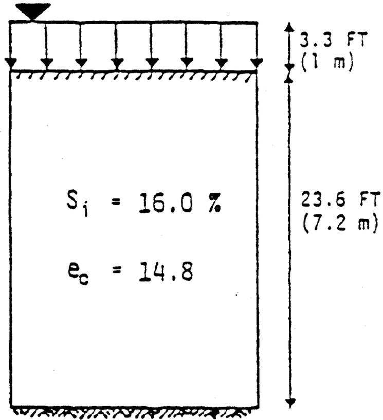
Figure 6.13. Pond 2a: Quiescent Consolidation with Uniform Void Ratio and Surcharge.
