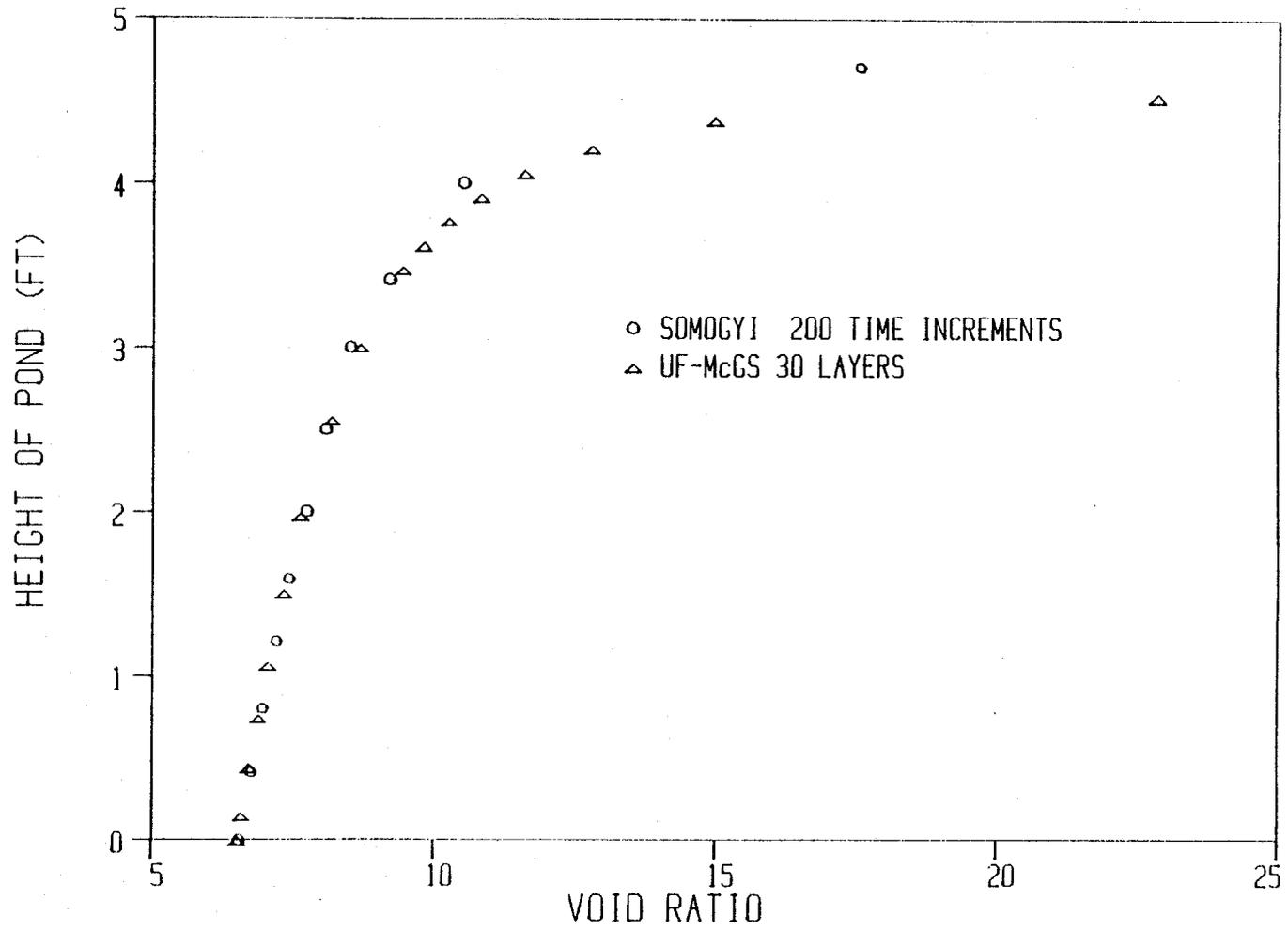
Figure 6.26. One year Void Ratio Profile for Pond 3a.
