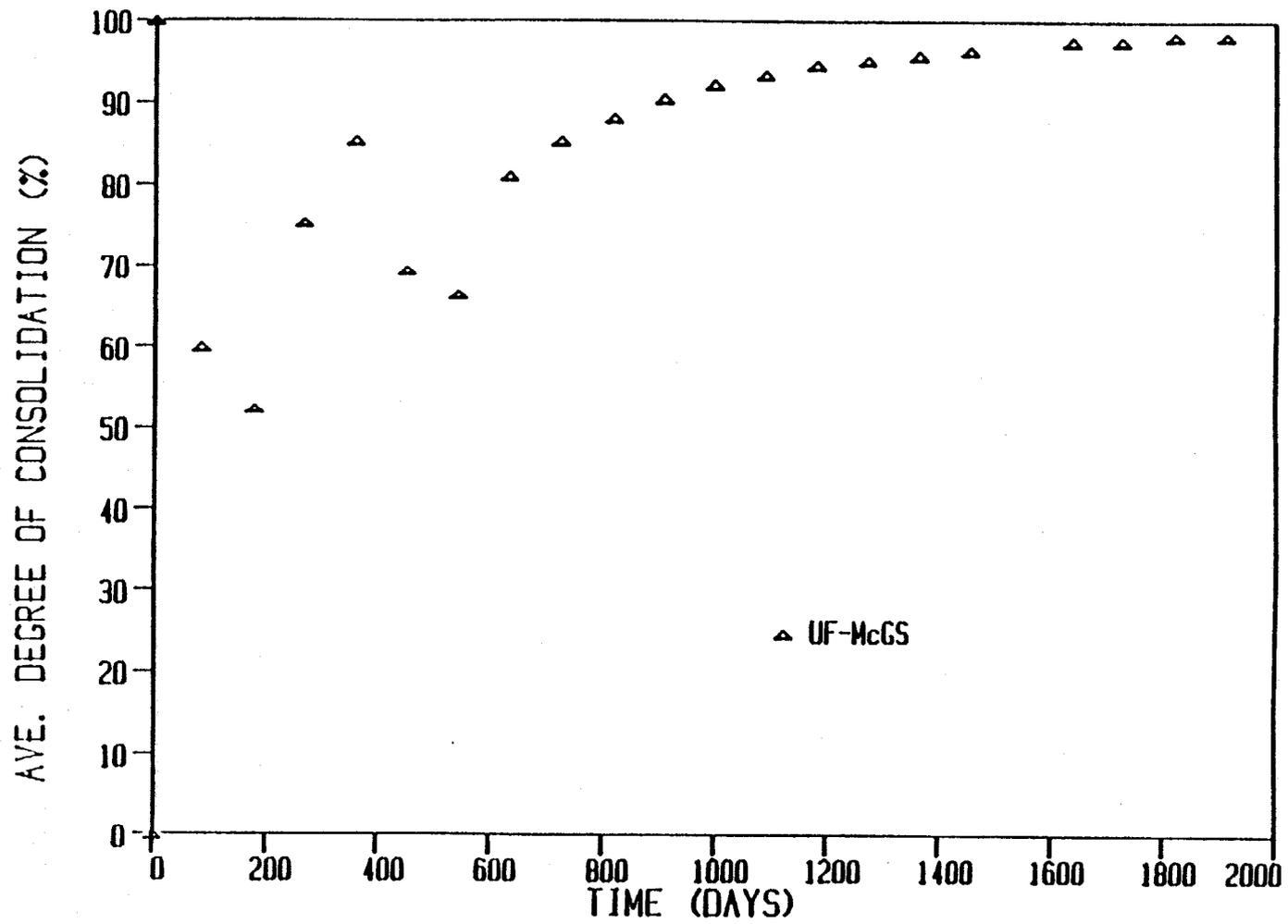
Figure 6.28. Average Degree of Consolidation vs. Time for Pond 3b.
