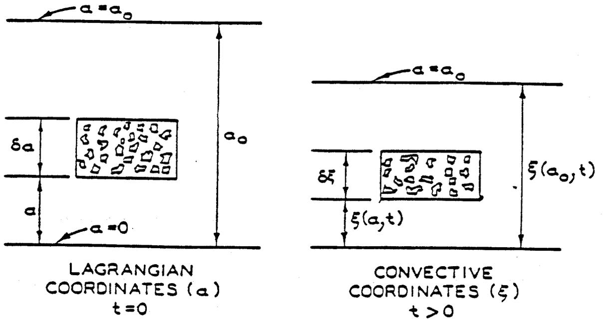
Figure 3.1. Geometrical Description of Soil Elements in Lagrangian and Convective Coordinates (Cargill, 1982).
