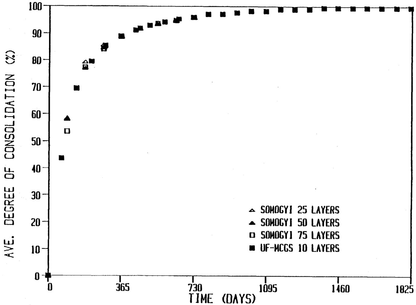
Figure 6.6. Average Degree of Consolidation vs. Time for Pond 1a.
