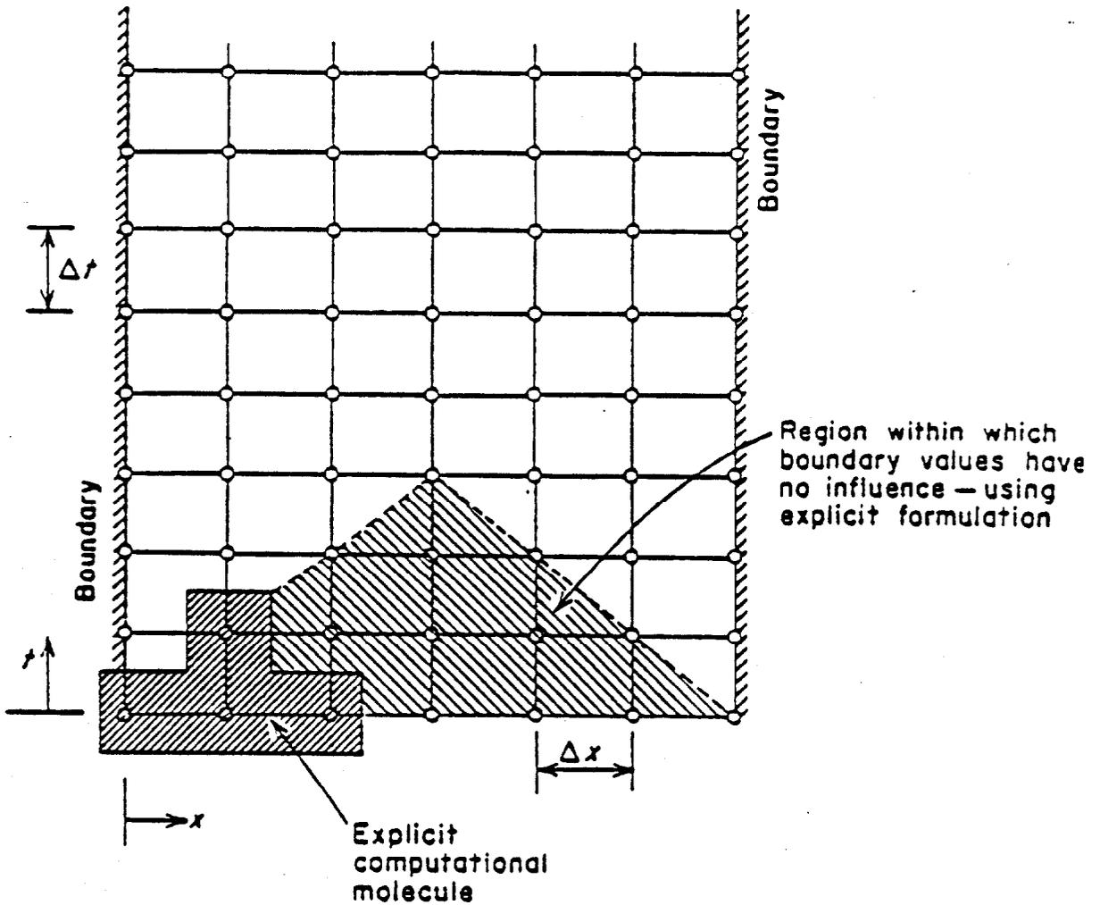
Figure 4.1. Depiction of Major Drawback Inherent with Explicit Finite Difference Schemes (Ketter and Prawel, 1969).
