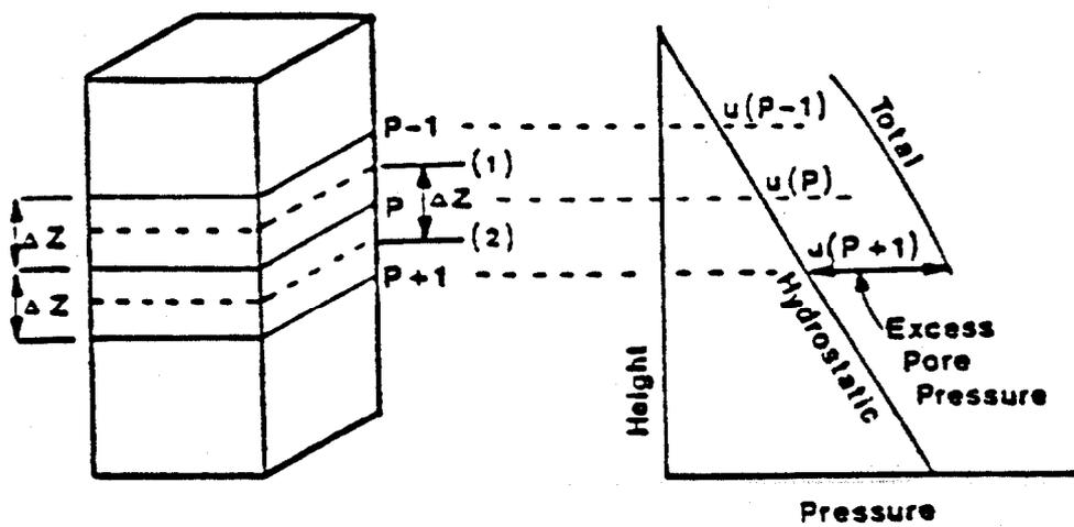
Figure 4.4. Discretization of Elemental Volume Used in the Derivation of the UF-McGS, UF-McGM and Yong Models (Yong et al., 1983).
