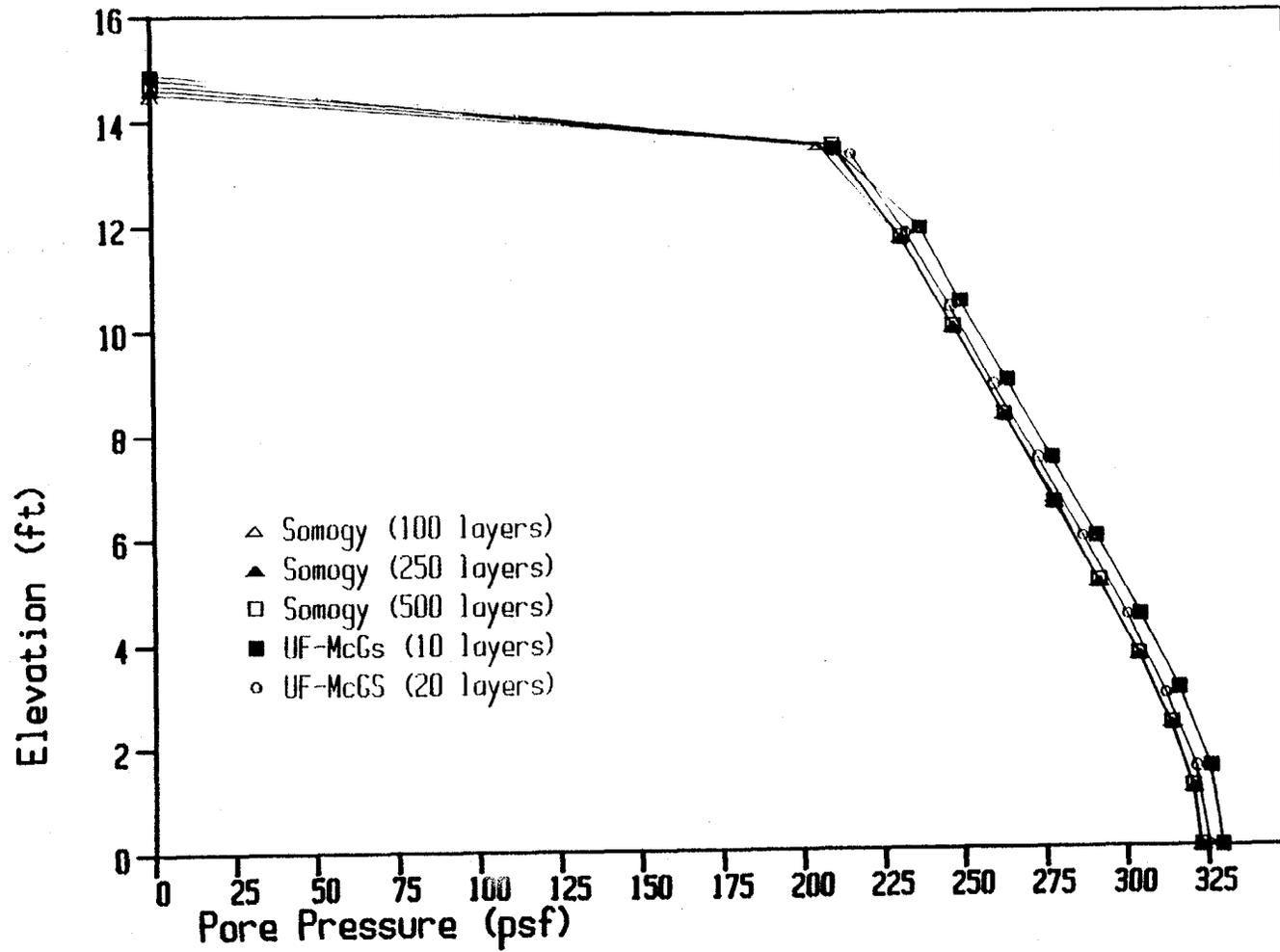
Figure 6.16. Pore Pressure Profile for Pond 2a.
