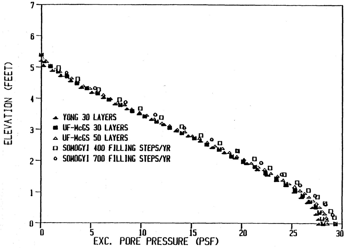
Figure 5.1. Pore Pressure Distribution at Pond 3a at .5 years.
