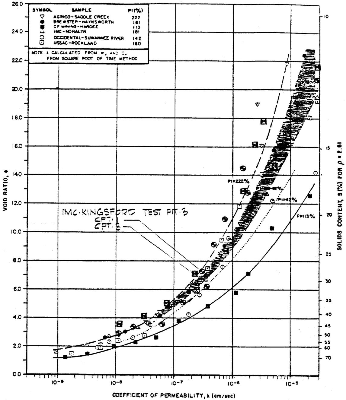
Figure 3.4. Void Ratio vs. Permeability for Phosphatic Clays (Wissa et al., 1983).
