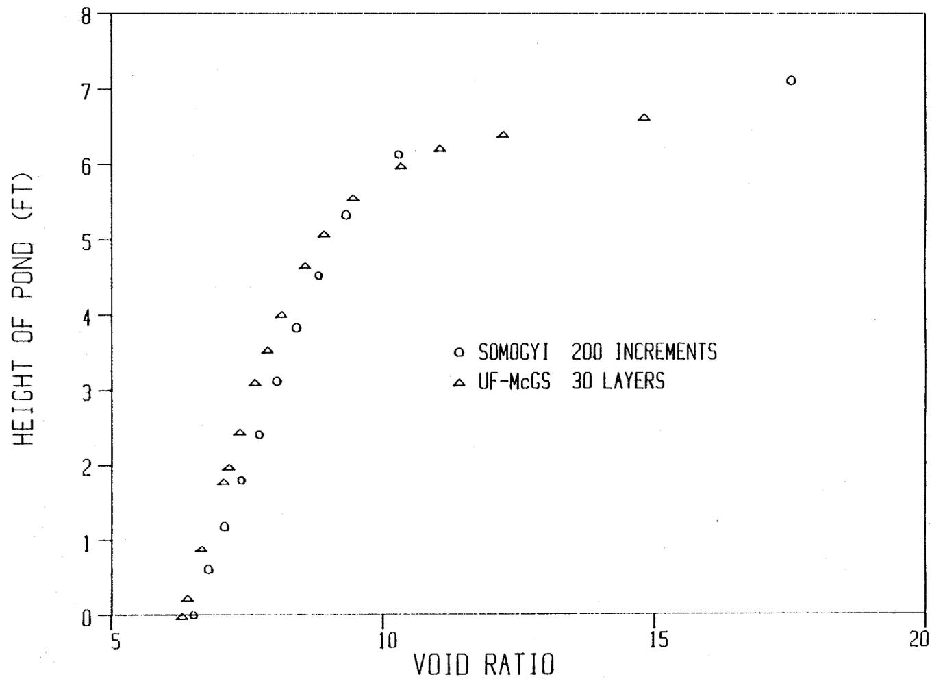
Figure 6.29. One year Void Ratio Profile for Pond 3b.
