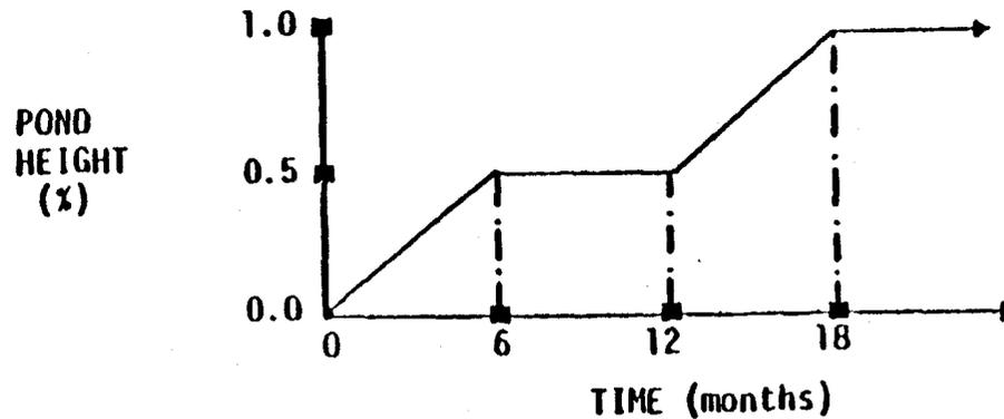
Figure 6.23. Stage Filling: (1) Pond 3a. Uniform Void Ratio.
