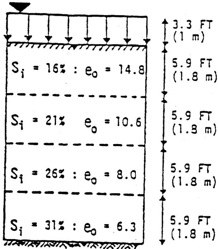
Figure 6. 17. Pond 2b: Quiescent Consolidation with Variable Void Ratio and Surcharge.
