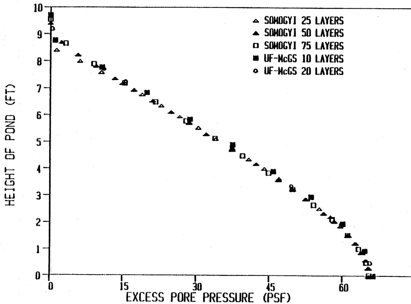
Figure 6.4. Pore Pressure Distribution after 1 Year for Pond 1a.
