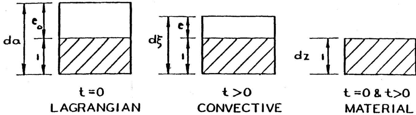
Figure 3.2. Comparison of Differential Soil Elements in Lagrangian, Convective, and Reduced Coordinates (Cargill, 1982).
