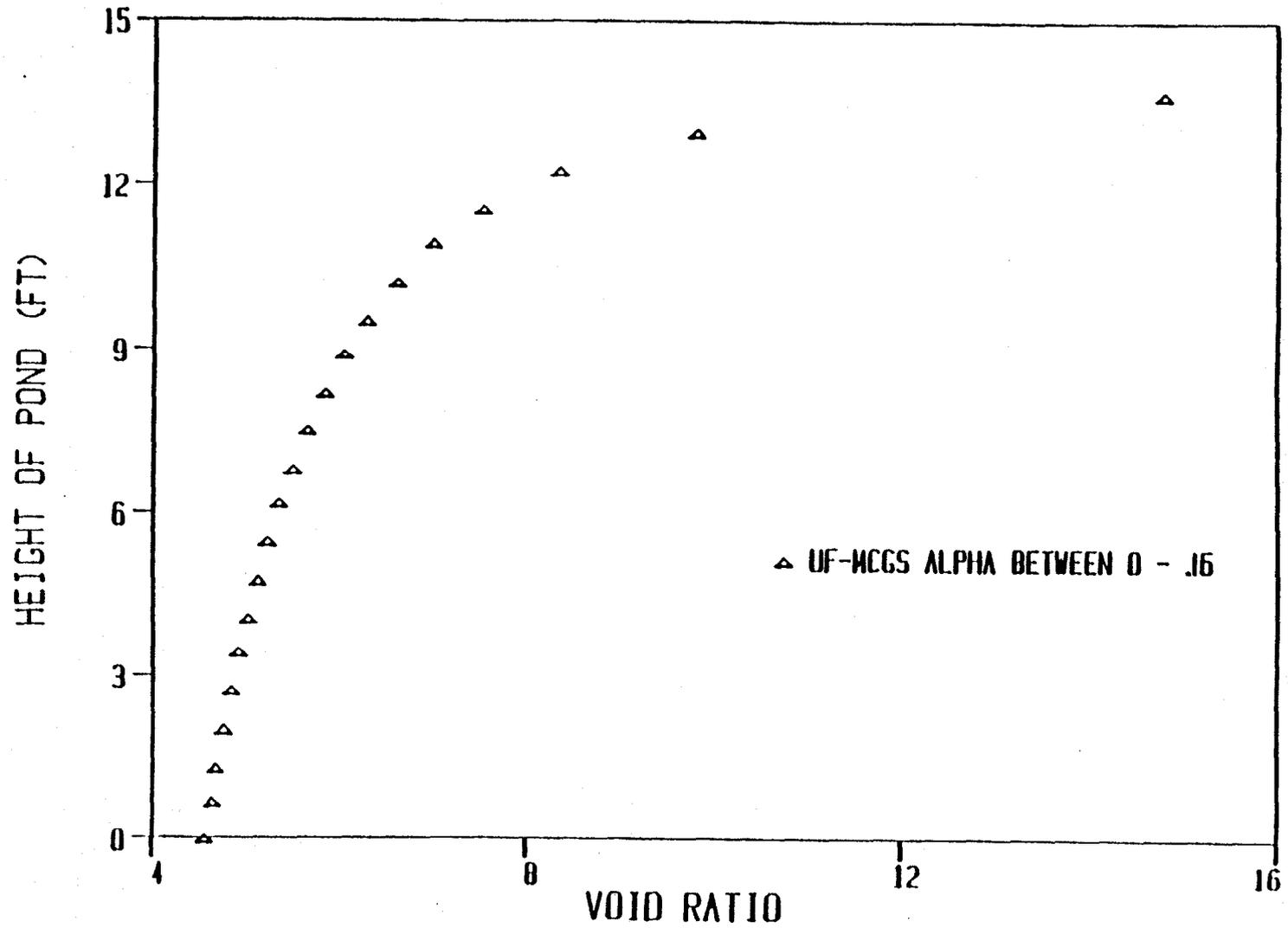
Figure 6.11. Final Void Ratio Distribution for Pond 1b.
