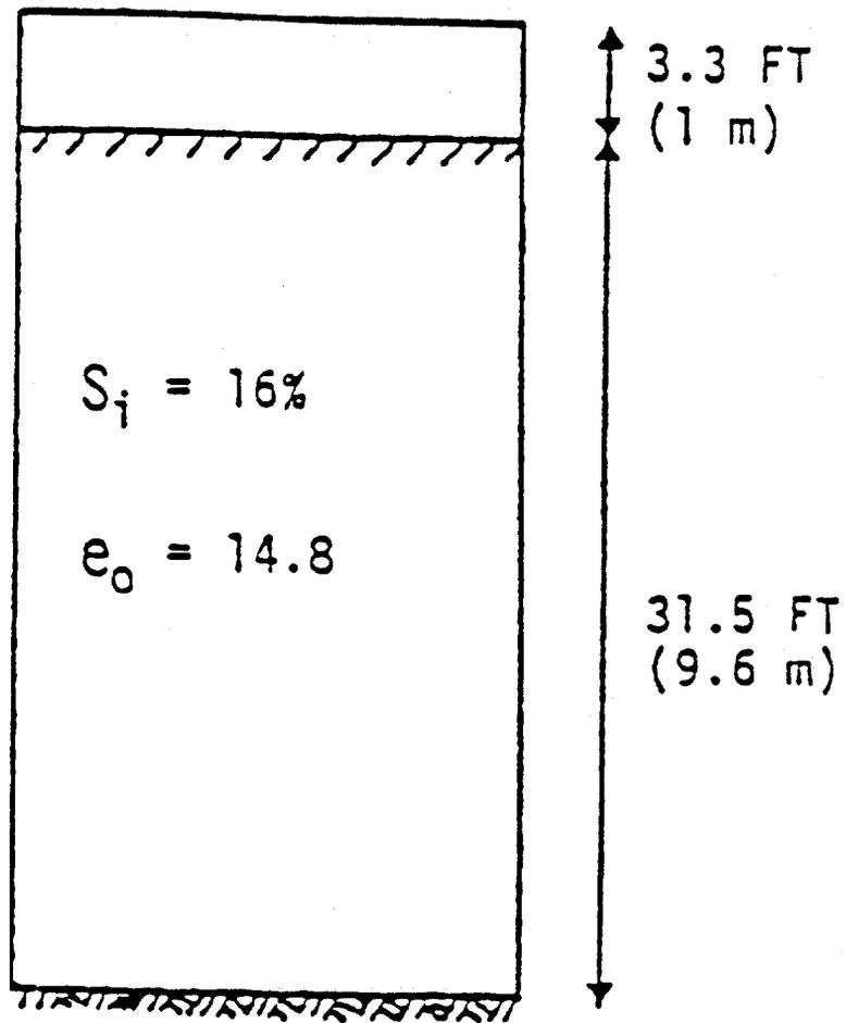
Figure 6.7. Pond 1b: Quiescent Consolidation with Uniform Void Ratio.
