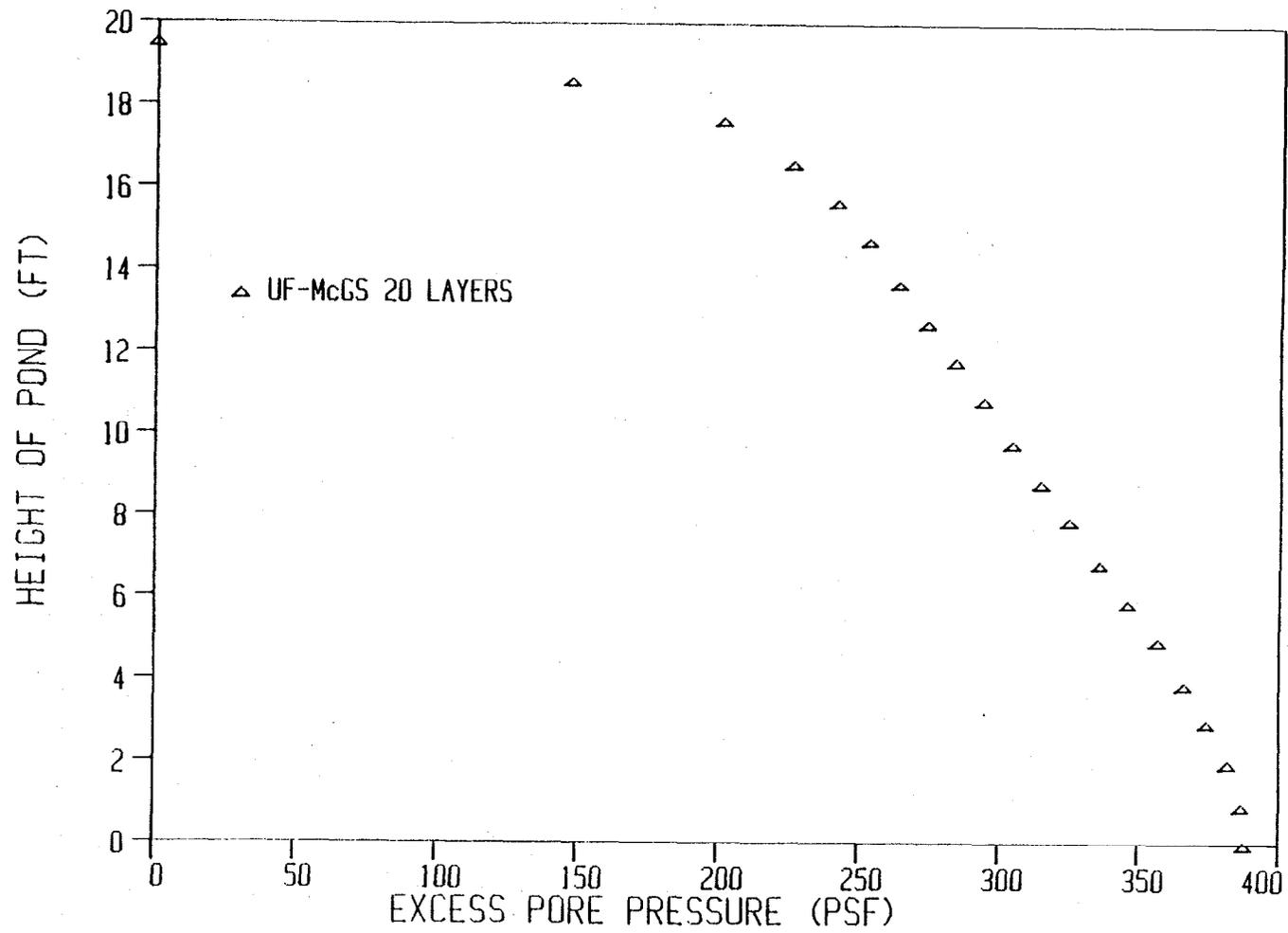
Figure 6.22. Excess Pore Pressure Profile at 1 year for Pond 2b.
