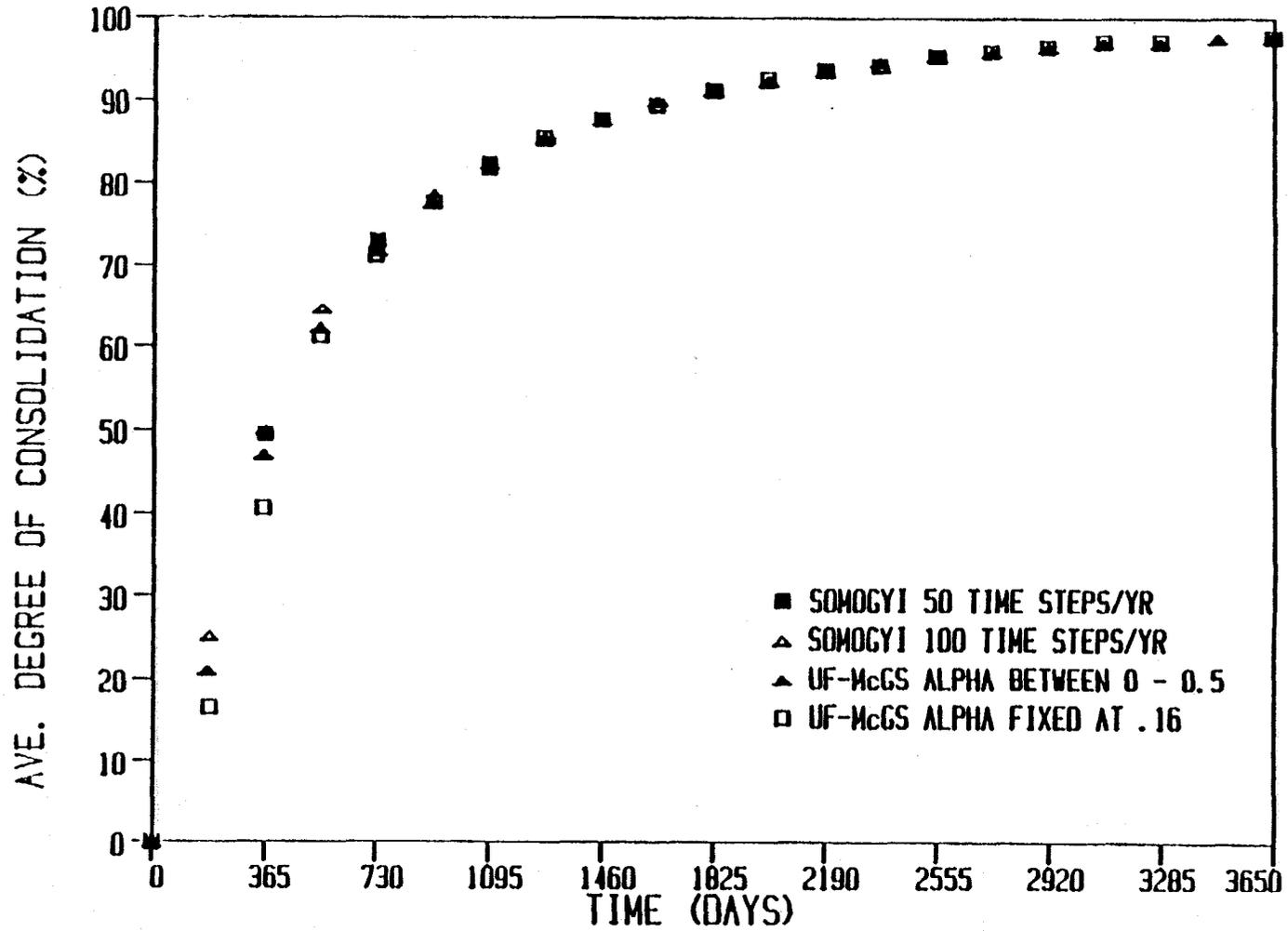
Figure 6.12. Average Degree of Consolidation vs. Time for Pond 1b.
