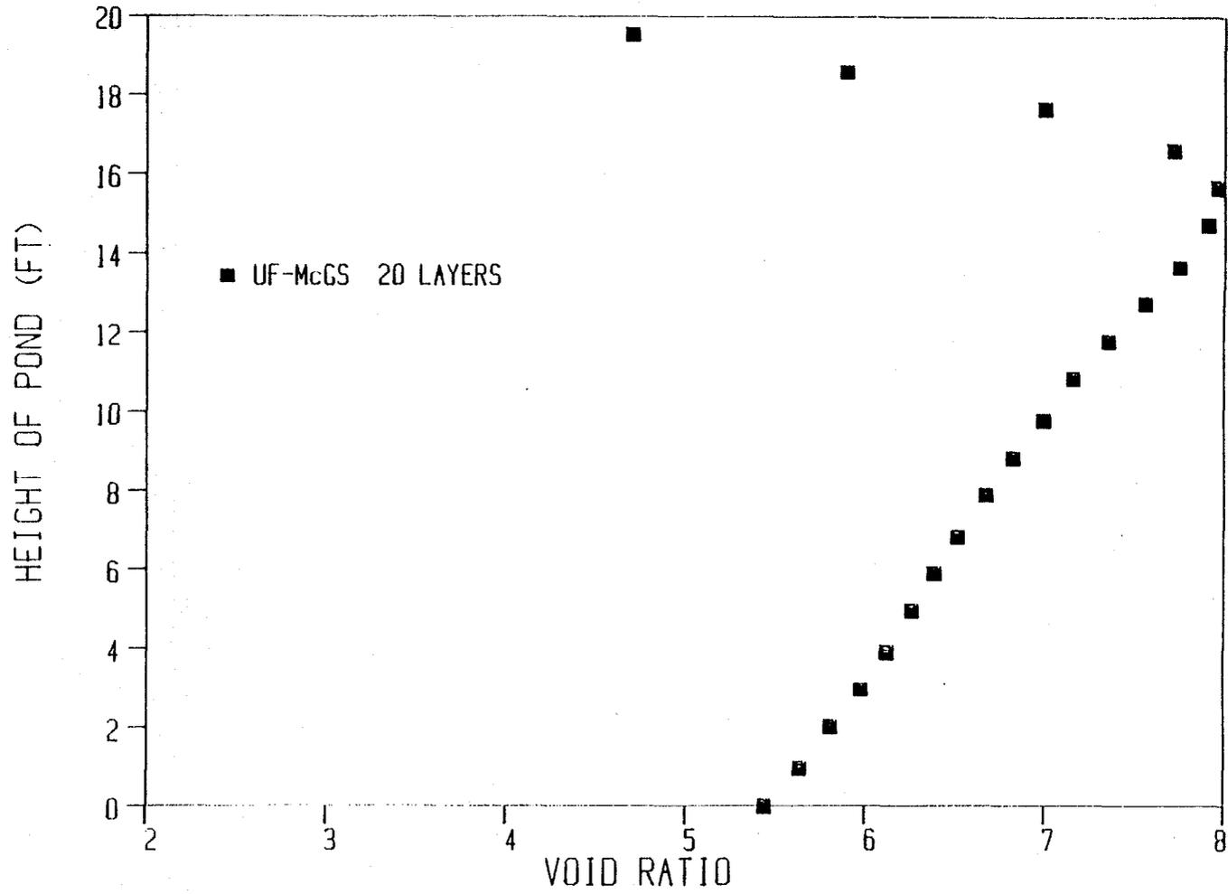
Figure 6.21. Void Ratio Profile at 1 year for Pond 2b.
