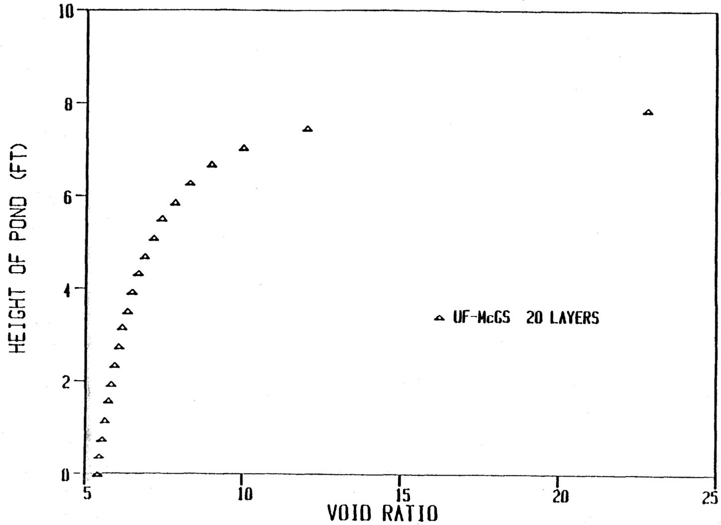
Figure 6.5. Final Void Ratio Distribution for Pond 1a.
