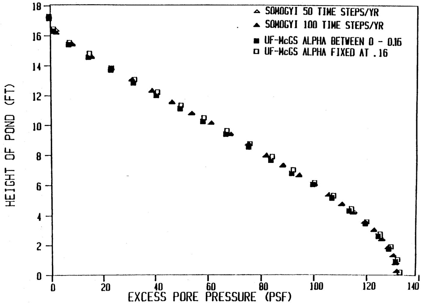
Figure 6.10. Pore Pressure Distribution after 3 Years for Pond 1b.
