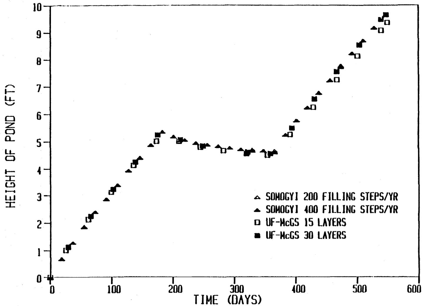
Figure 6.24. Height vs. Time for Pond 3a.
