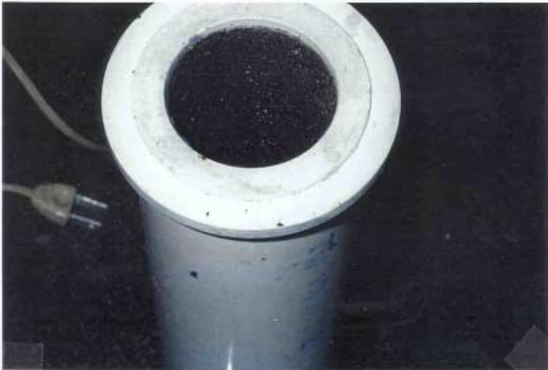
Figure AP-D6. Crud Build-Up at the Wired Steel Porous Tube Surface (Rough) (After 9 Hours' Operation).
