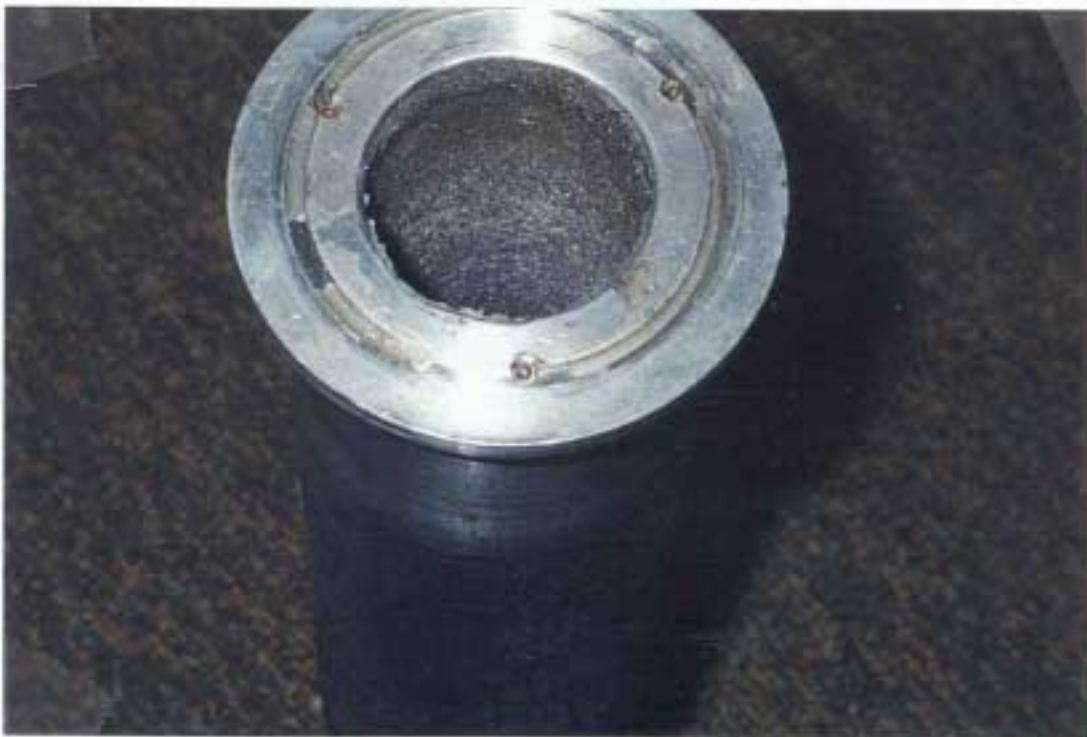
Figure AP-D3. Crud Build-Up at Stainless Steel Porous Tube Surface (After 16 Hours' Operation).
