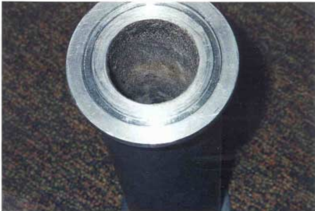
Figure 65. Crud Build-up Was Reduced at Stainless Steel Porous Tube with Electric Field (After 18 Hours' Operation).
