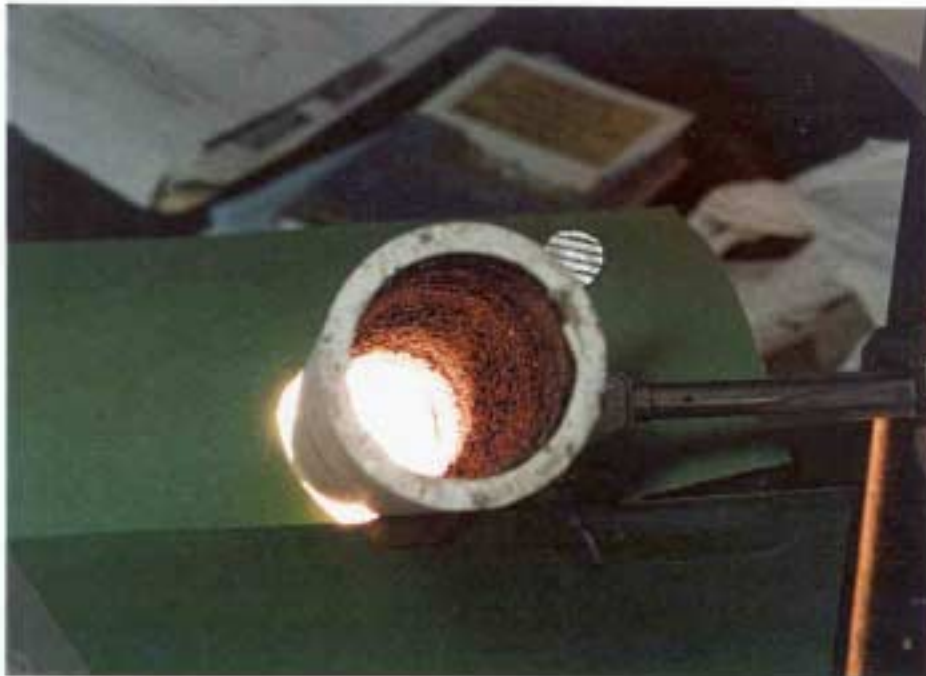
Figure AP-D2. Crud Build-up at the Coarse Plastic Porous Tube Surface (After 18 Hours' Operation).
