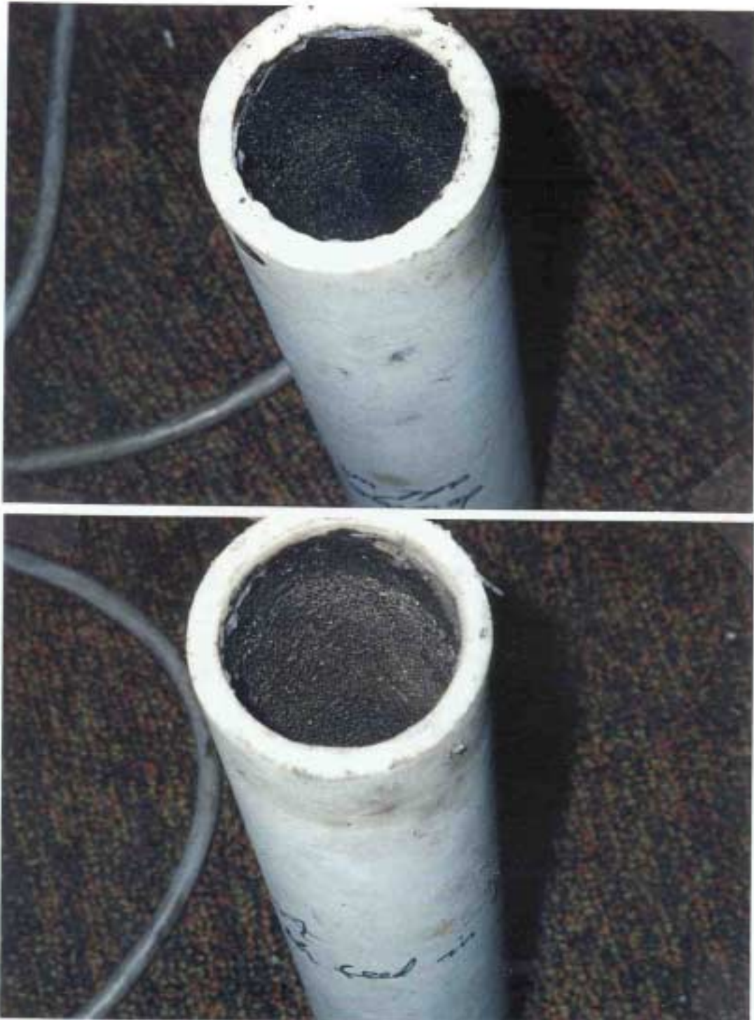
Figure AP-D7. Crud Build-Up at the Plastic Porous Tube When Detergent Was Added with Feed (After 18 Hours' Operation).
