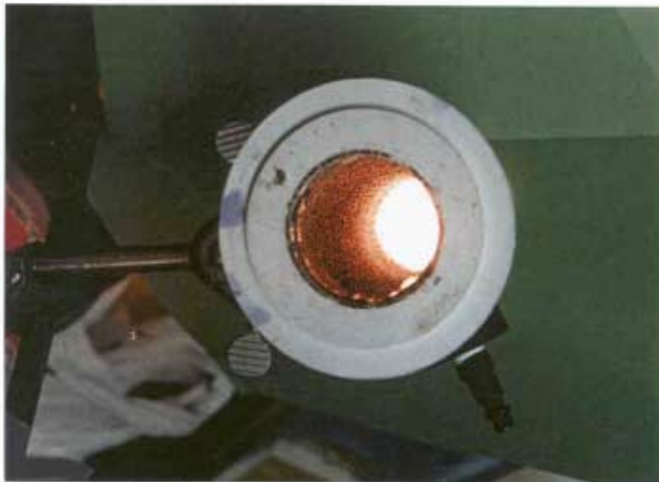
Figure AP-D4. Crud Build-Up at the Ceramic Porous Tube Surface (After 18 Hours' Operation).
