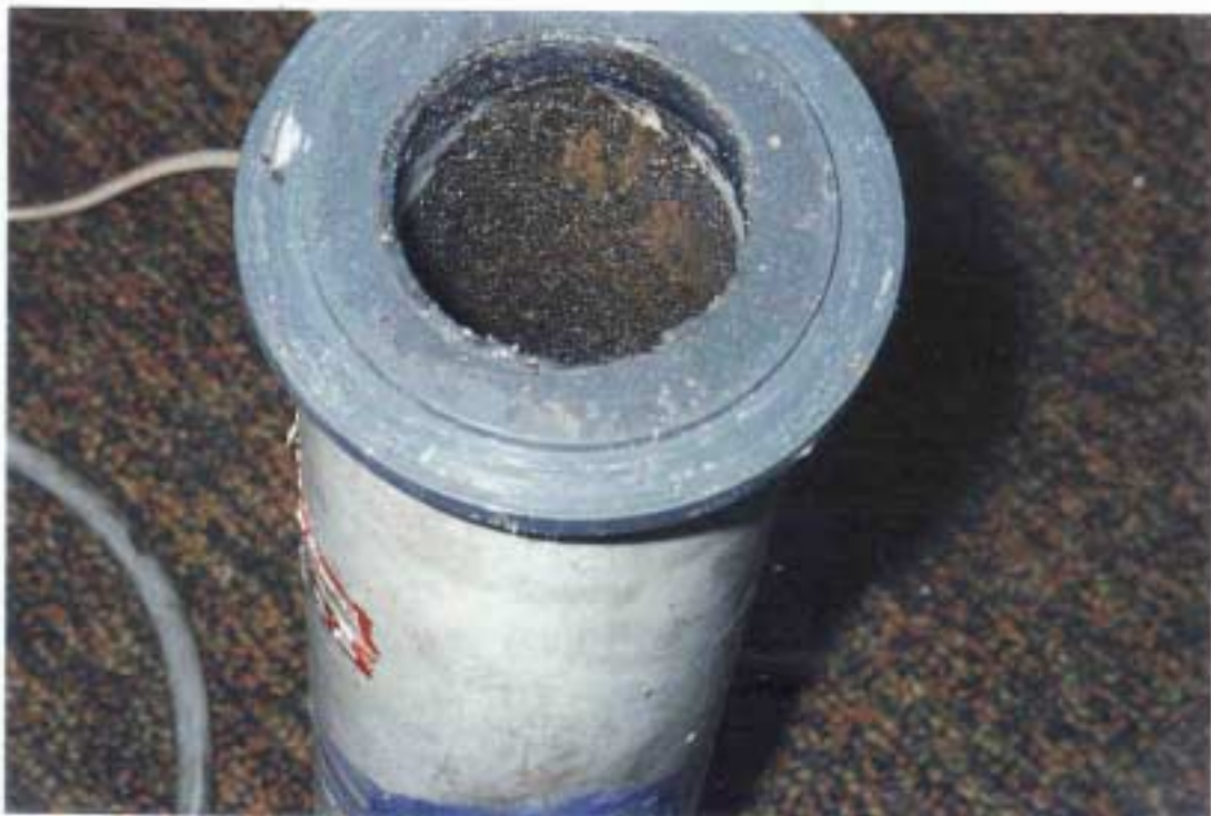
Figure AP-D8. Crud Build-up at Plastic Porous Tube after Cleaning with Detergent (After 12 Hours' Operation).
