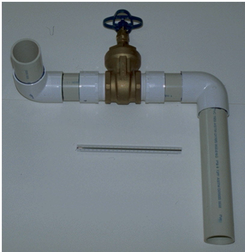
Figure 16. PVC-Brass Valve Assembly for Penetrating Spillway Boards. [04/12/99: 29]
