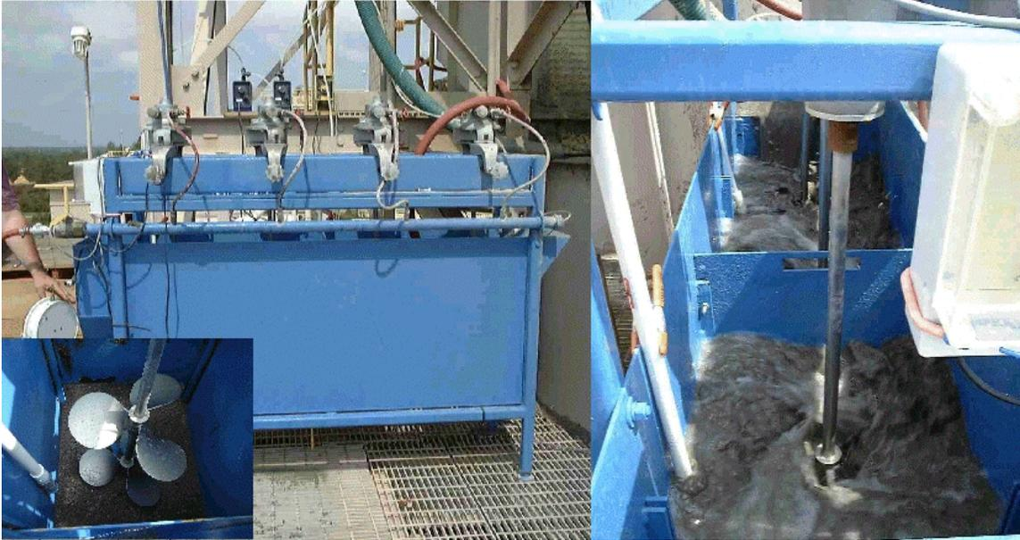
**Figure 7. Photograph of the Stirred-Tank Conditioner.**
