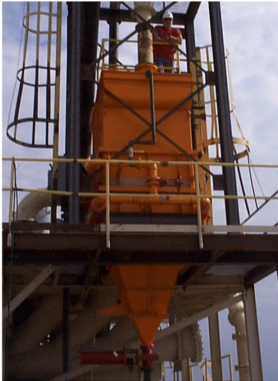
**Figure 5. Photograph of the 5 Ft. x 5 Ft. CrossFlow Classifier.**
