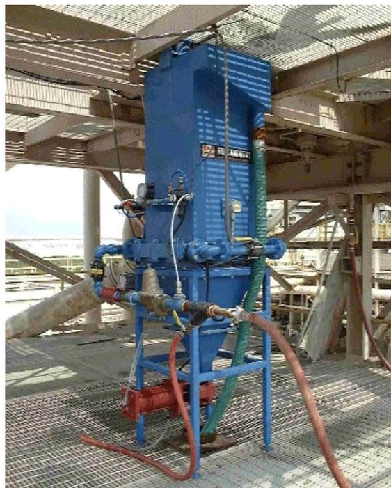
**Figure 6. Photograph of the Pilot-Scale HydroFloat Separator.**
