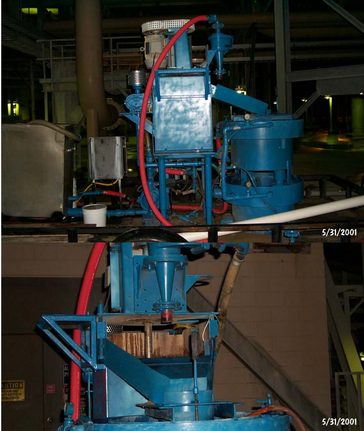
Figure 1. Pilot Plant DEC Set-Up Employed in Rougher Concentrate and IP Flotation Studies.
