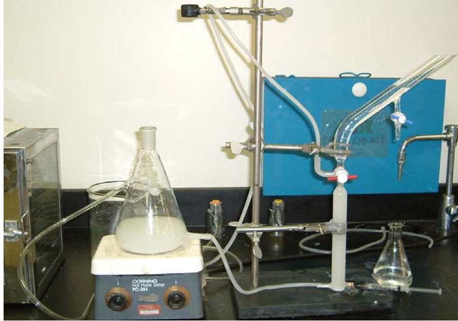
Figure 5. Microflotation Experimental Setup.
