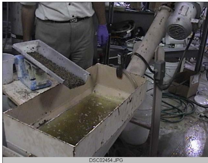
Figure 16. Screw Dewatering Device.
