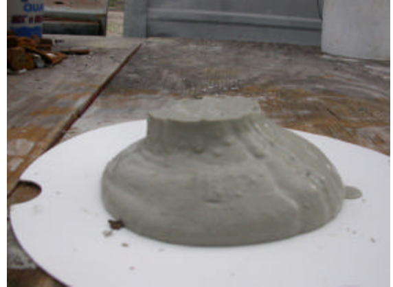
Figure 95. Paste Slump Tests for Determining Yield Stress of Paste.
