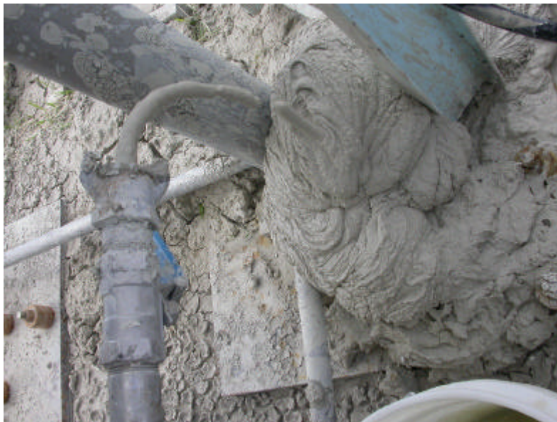
Figure 93. Paste Products with 30.08% Solids (Top) and 35.44% Solids (Bottom).
