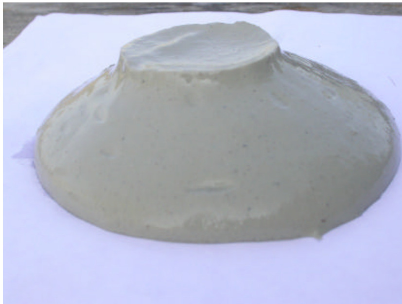
Figure 89. Paste from Test 19 with 19.79% Total Solids and 15.87% Clay Solids.
