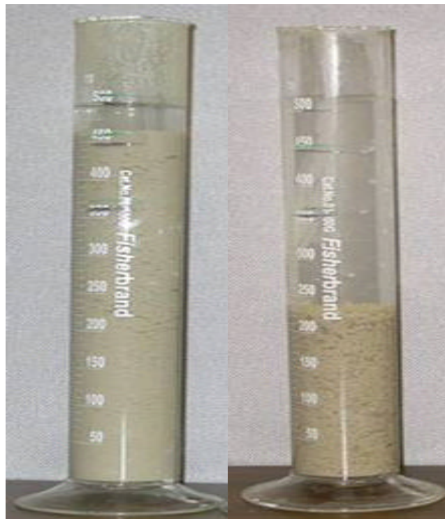
Figure 88. Effects of Sand Addition on Clay Consolidation: No Sand (left); Sand Added (right).
