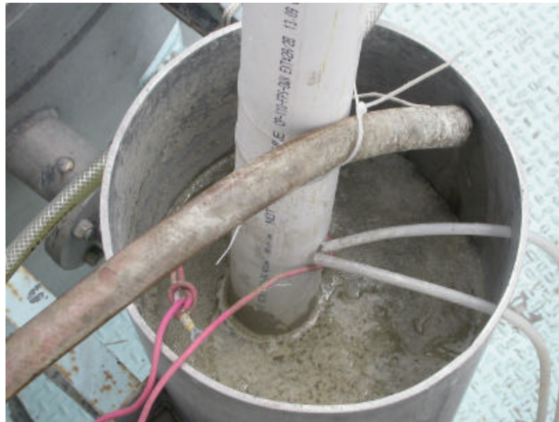
Figure 86. Flocculation Inside Conditioning Tank Beside DCT Where Hengfloc 80607 Was Added.
