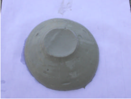
Figure 95. Paste Slump Tests for Determining Yield Stress of Paste.
