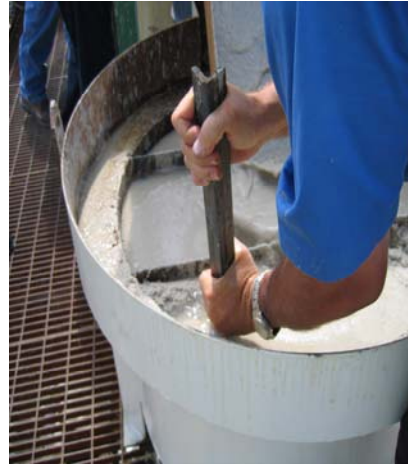
Cyclone Underflow to the Clarifying Cone
