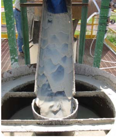
Cyclone Underflow to the Clarifying Cone
