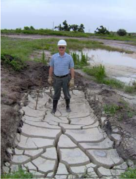
Figure 10. Clay/Sand Mixture in Test Pit after Three Days of Disposal (Dewatered Clays Show Some Load-Bearing Capacity).
