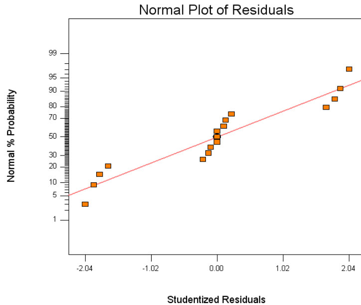
Figure 62. Normal Probability Plot of Residual for Separation Efficiency of Unsized Phosphate Particle Flotation.
