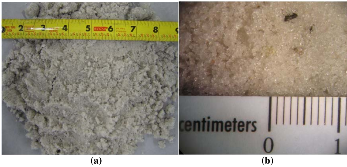
Figure 50. Unsized Phosphate Flotation Tailing in the Presence of Picobubbles: (a) Photographic Image; (b) Optical Microscopic Image.
