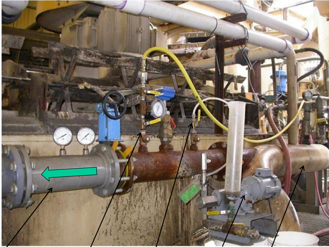
Cavitation tube Compressed air input Frother input Frother pump Process water pipe
