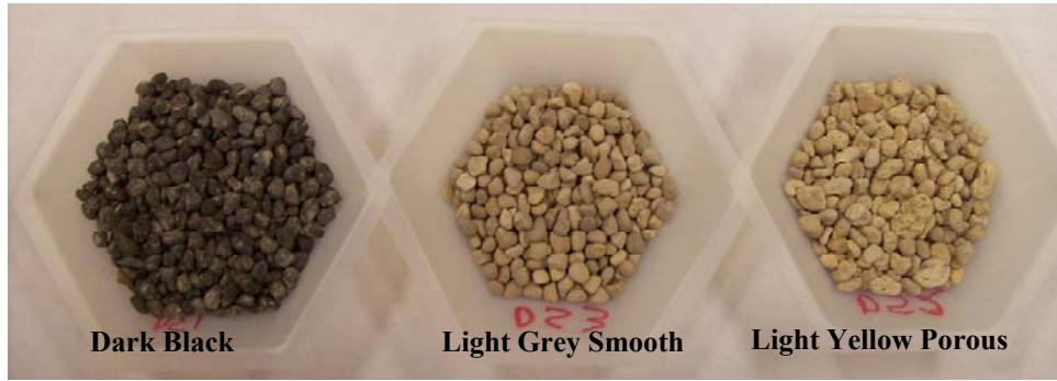
Figure 10. The High-Dolomite Phosphate Ore Was Hand-Separated into Three Main Categories by Color and Texture.
