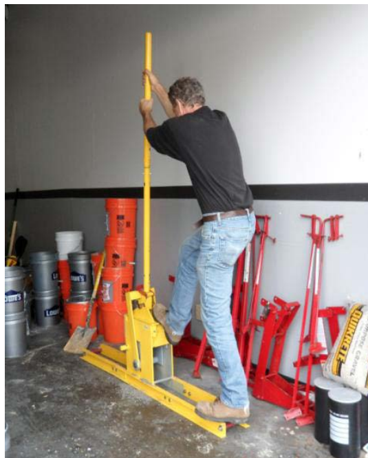
Figure 14. Operating Block Press.
