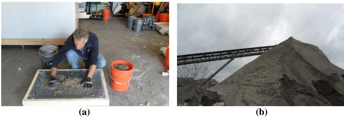
(a) (b) Figure 8. Sifting Crushed Concrete.
