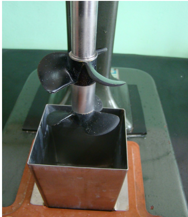
Photo 1. Steel Scrubber with Steel Balls and Double Impellers.
