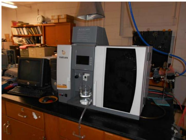
**Figure 6. Varian AA240FS Fast Sequential Spectrometer Used for MgO Analysis.**
