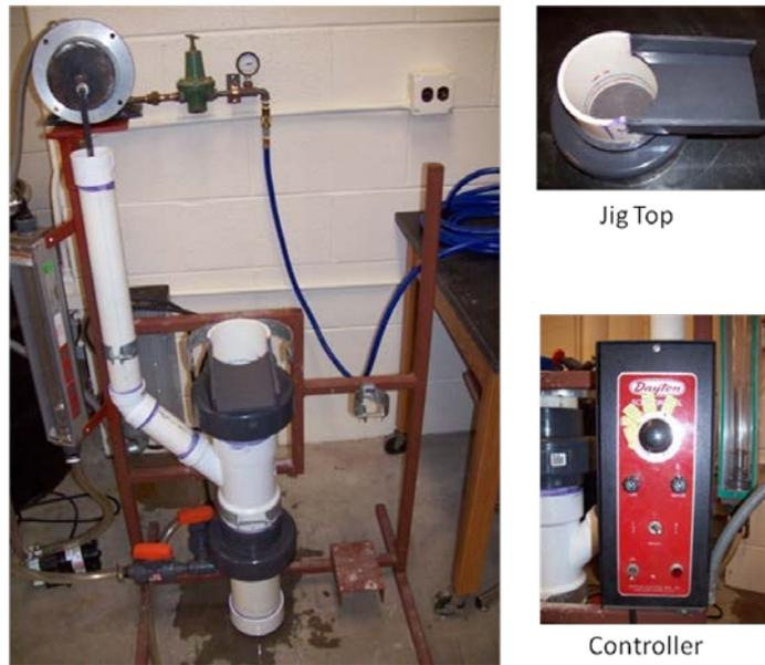
**Figure 22. Photo of Large Laboratory-Scale Jig.**
