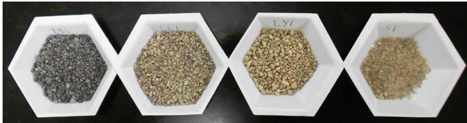
**Figure 36. Sample of High-MgO Mosaic Phosphate Ore (5×20 Mesh) Hand-Separated into Four Different Categories: Dark Black Pebbles, Light Gray Pebbles, Light Yellow Pebbles, and Silica Pebbles.**
