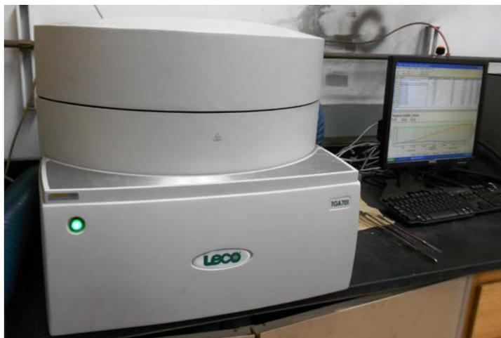
**Figure 12. Leco TGA701 Thermogravimetric Analyzer Used for Carbonate Analysis.**
