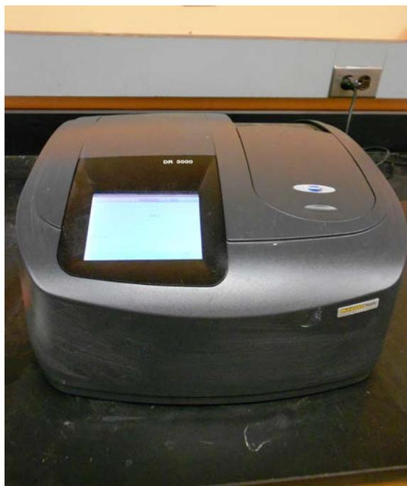
**Figure 9. Hach DR 5000 UV-Vis Spectrophotometer Used for BPL Analysis.**
