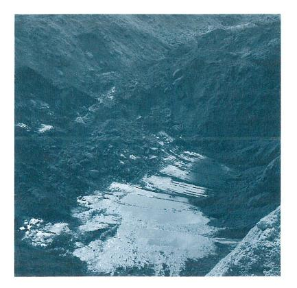
Figure 10. Excavation pit in North Carolina where the phosphatic clay matrix is approximately 30 m deep.
