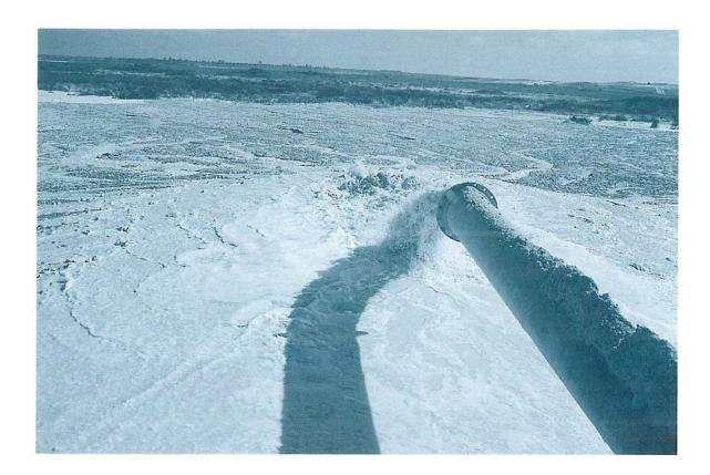
Figure 3. Sand tailings transported by hydraulic pumping.
