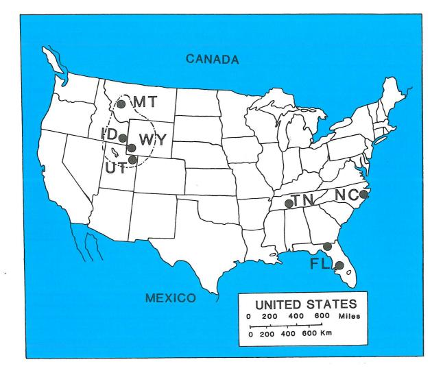
Figure 1. Areas of phosphate rock production in the United States. Note the 4 major areas include Florida, coastal North Carolina, Tennessee, and the western states of Idaho, Montana, Wyoming, and Utah (After Buie et al. 1975).
