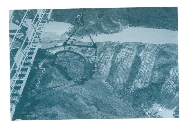
Figure 9. Excavation down to the phosphatic clay matrix (10-15 m) in Florida.
