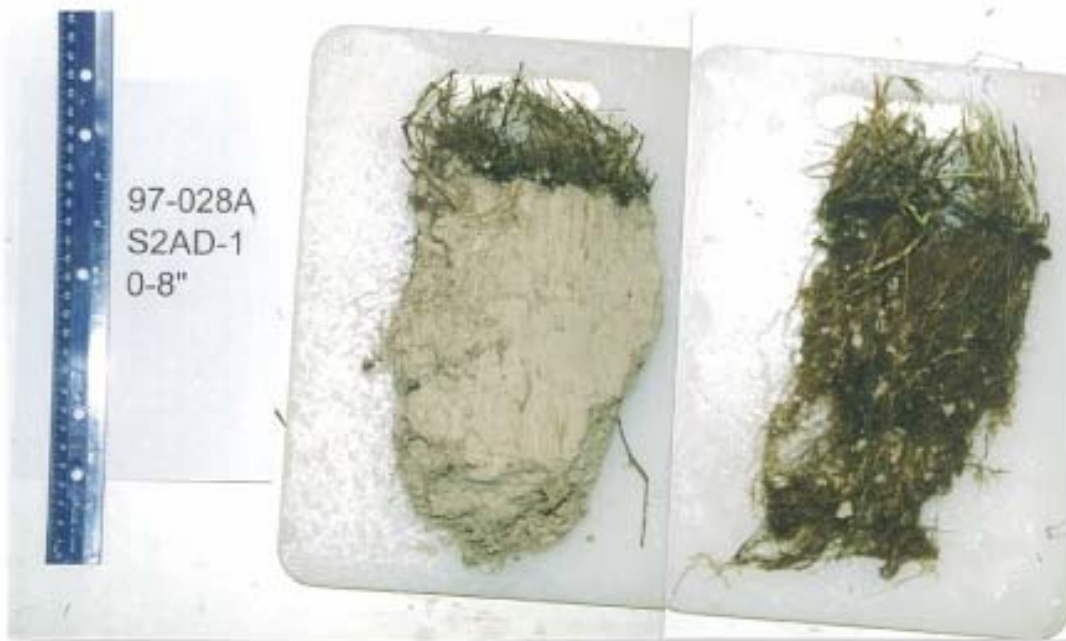
Photograph J-7. Root Growth in Side Slope Test Plot S2A on 09/07/01 (T=1072 Days).
