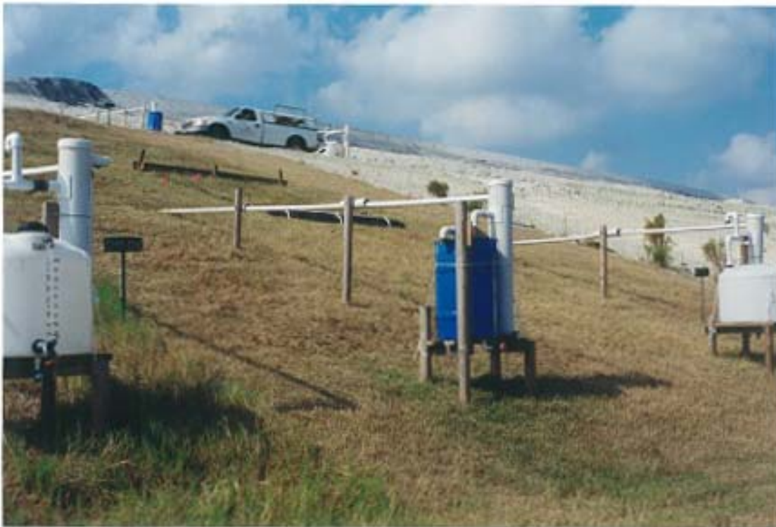
Photograph I-28. Side Slope Test Plot S2G After Mowing on 11/01/99 (T = 396 Days).
