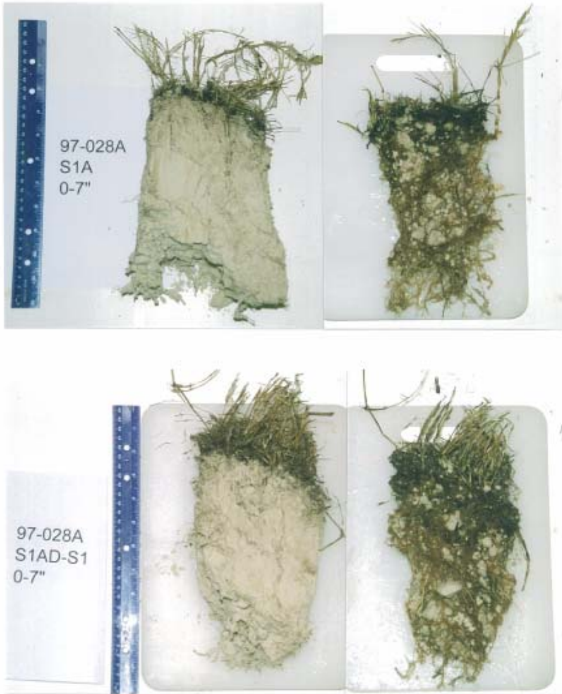
Photograph J-5. Root Growth in Side Slope Test Plot S1A on 09/07/01 (T=1072 Days).
