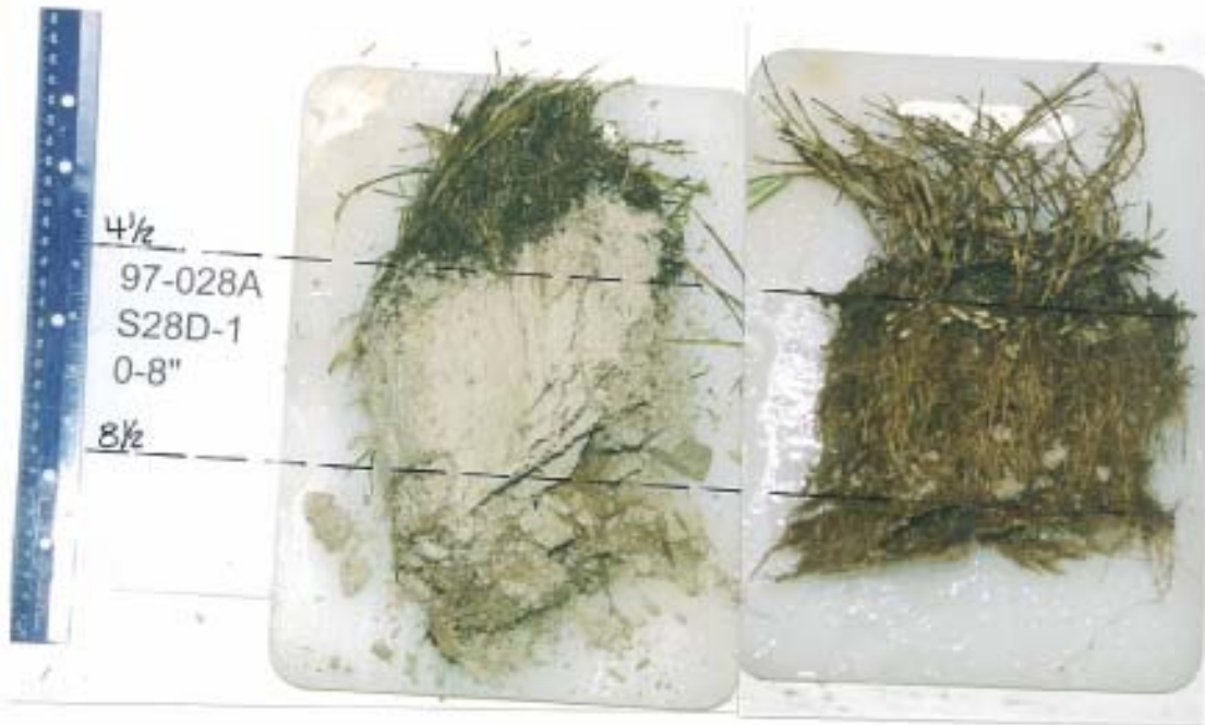
Photograph J-8. Root Growth in Side Slope Test Plot S2B on 09/07/01 (T=1072 Days).
