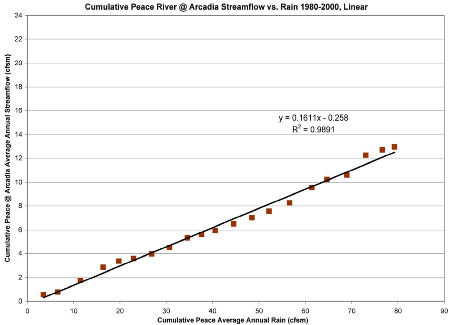
Figure H-8. Peace River @ Arcadia Cumulative Rain Versus Streamflow (Linear).
