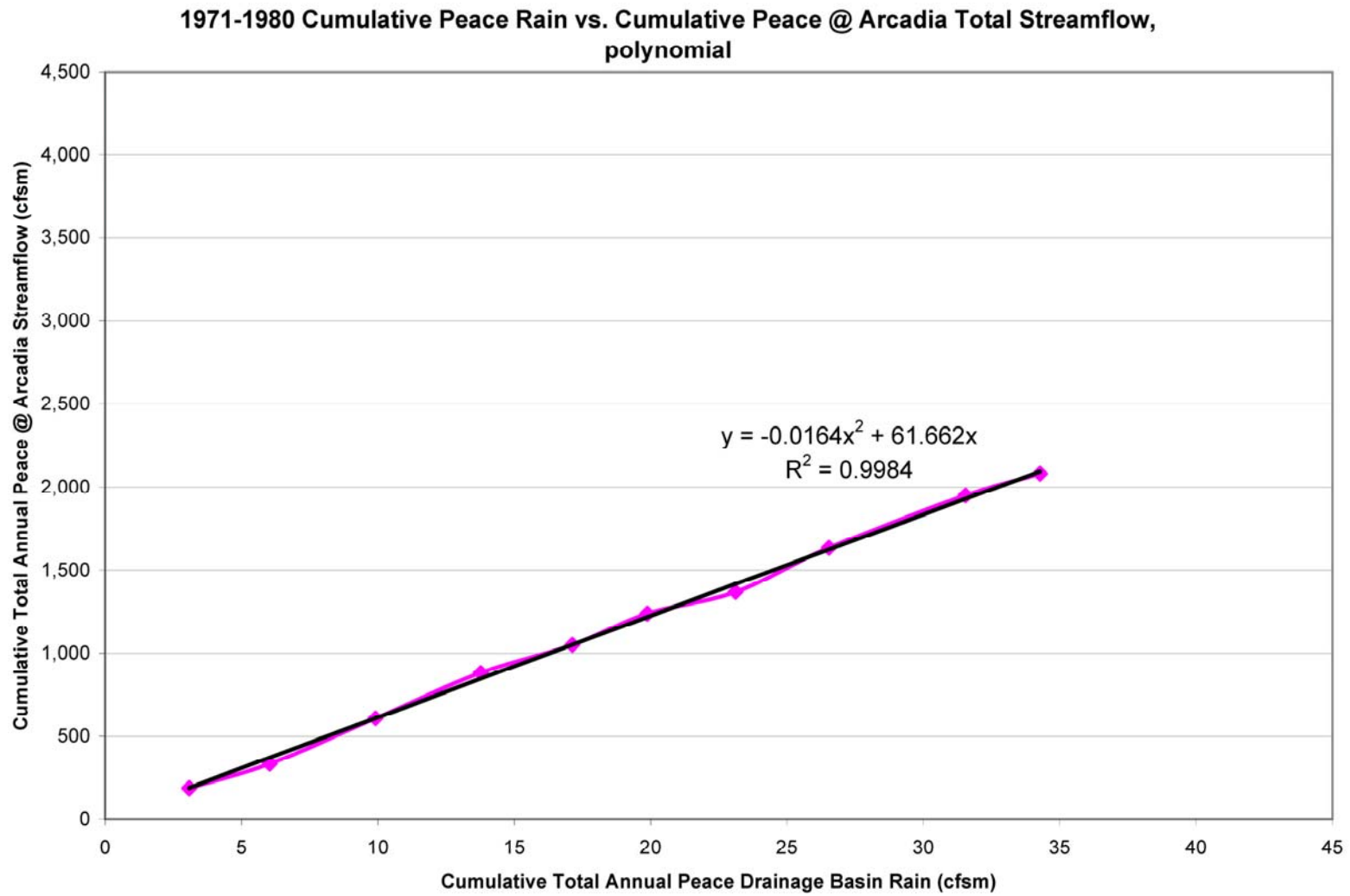
Figure G-5. Cumulative Peace Streamflow Versus Rain (cfsm), 1971-1980 (Polynomial).
