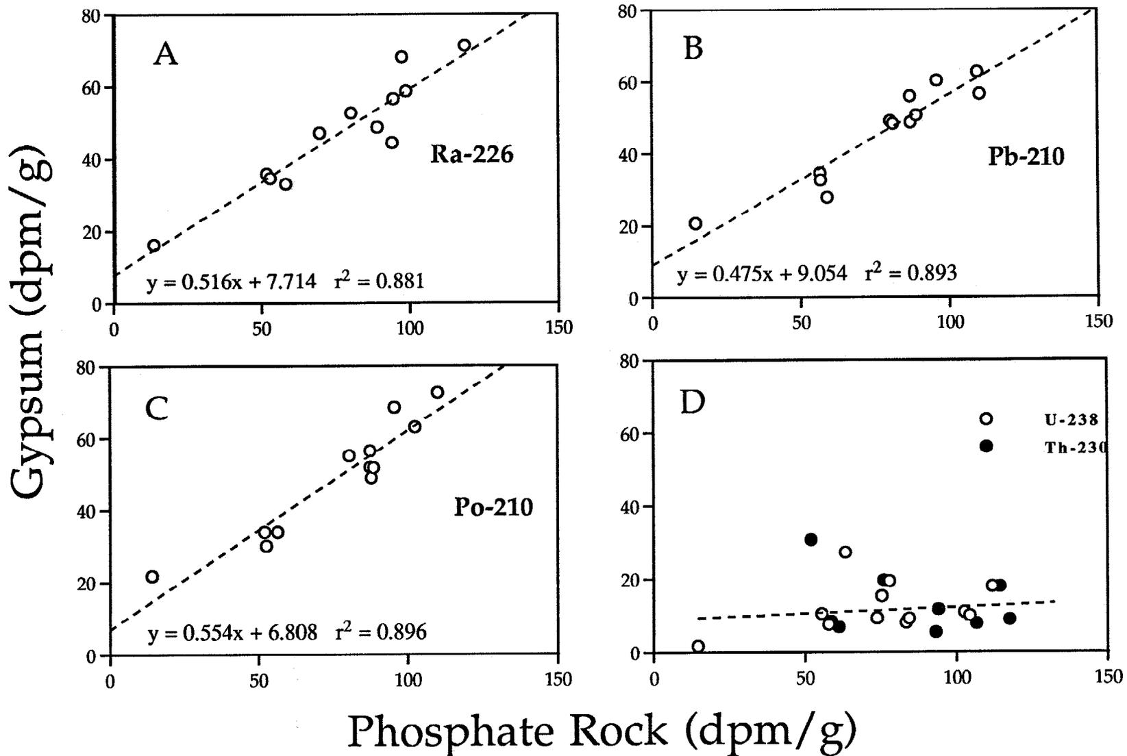
Fig. 1-9 Relationships of activities of uranium-series radionuclides in gypsum *versus* phosphate rock for (A)  $^{226}\text{Ra}$ ; (B)  $^{210}\text{Pb}$ ; (C)  $^{210}\text{Po}$ ; and (D)  $^{238}\text{U}$  and  $^{230}\text{Th}$ . Least squares regression lines shown for  $^{226}\text{Ra}$ ,  $^{210}\text{Pb}$ , and  $^{210}\text{Po}$ .
