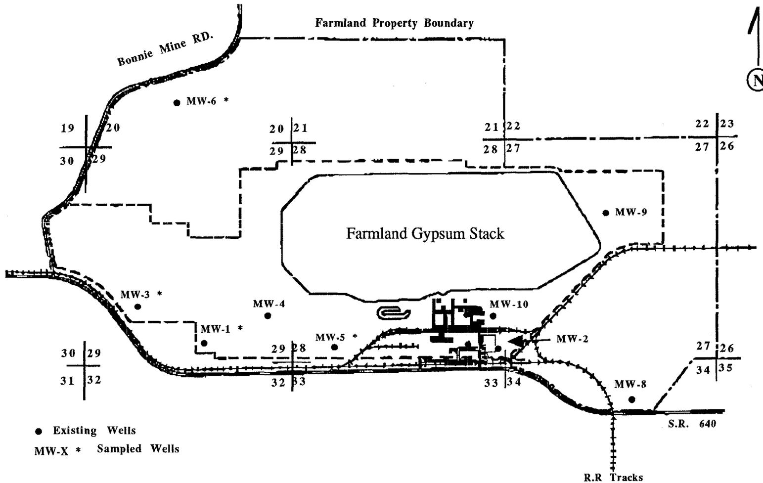
Fig. 1-2 Monitor wells sampled around the phosphogypsum stack at Farland Industries, Bartow, Florida. Samples were collected from wells 1, 3, 5, and 6.
