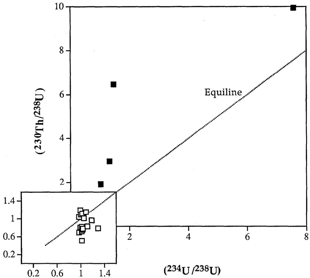
Fig. 1-10 Plot of activity ratios ( $^{230}\text{Th}/^{238}\text{U}$ ) versus ( $^{234}\text{U}/^{238}\text{U}$ ) for 17 samples of phosphogypsum. Replicate analyses have been produced and are plotted for most samples. Error bars are smaller than plotting symbols.
