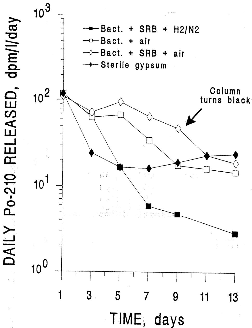
Fig. 4.7. The daily Po release under air and N<sub>2</sub>-H<sub>2</sub> purging. Symbols and treatments are the same as in Fig. 6.
