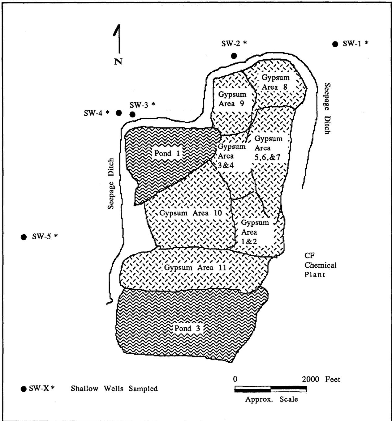
Fig. 1-5 Monitor wells sampled around the gypsum stack at C.F. Industries, Bartow, Florida. Water samples were collected from wells SW-1, 2, 3, and 5.
