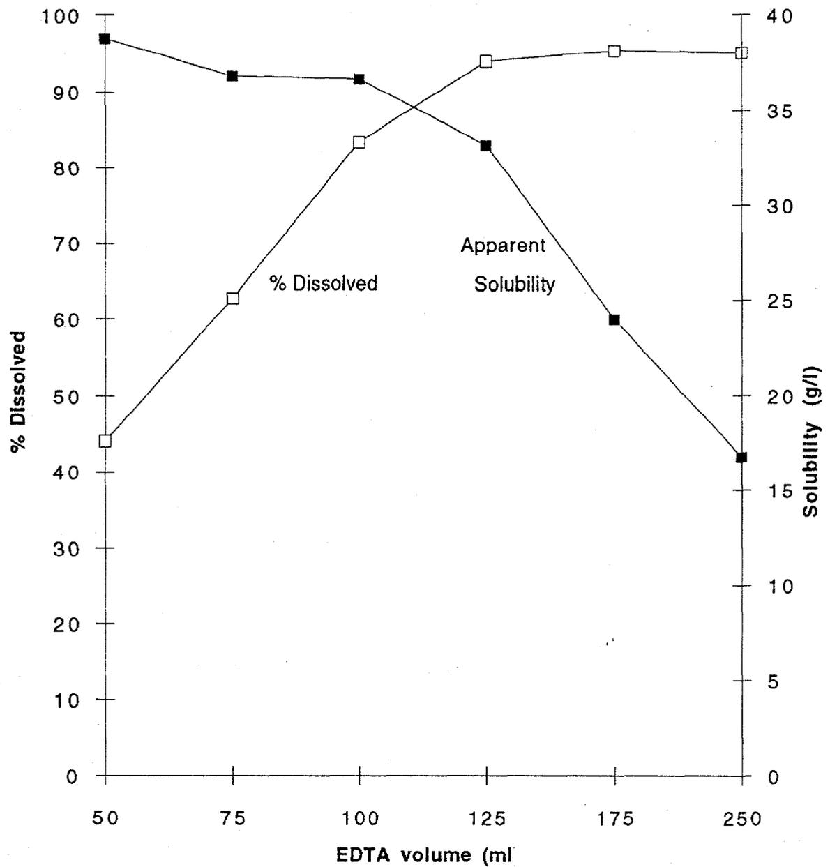
**Figure 2-1.** Fraction of constant weight (4.4 grams) of phosphogypsum sample Gyp-6 dissolved *versus* volume of 0.25 M EDTA at pH=10 added (left-hand scale). The apparent solubility of the phosphogypsum (right-hand scale) appears to decrease with increasing volume because the EDTA dissolves the more soluble fraction ( $\text{CaSO}_4 \cdot n \text{H}_2\text{O}$ ) until totally depleted and then attacks the less soluble fractions of the solid which may contain other sulfate mineral phases.
