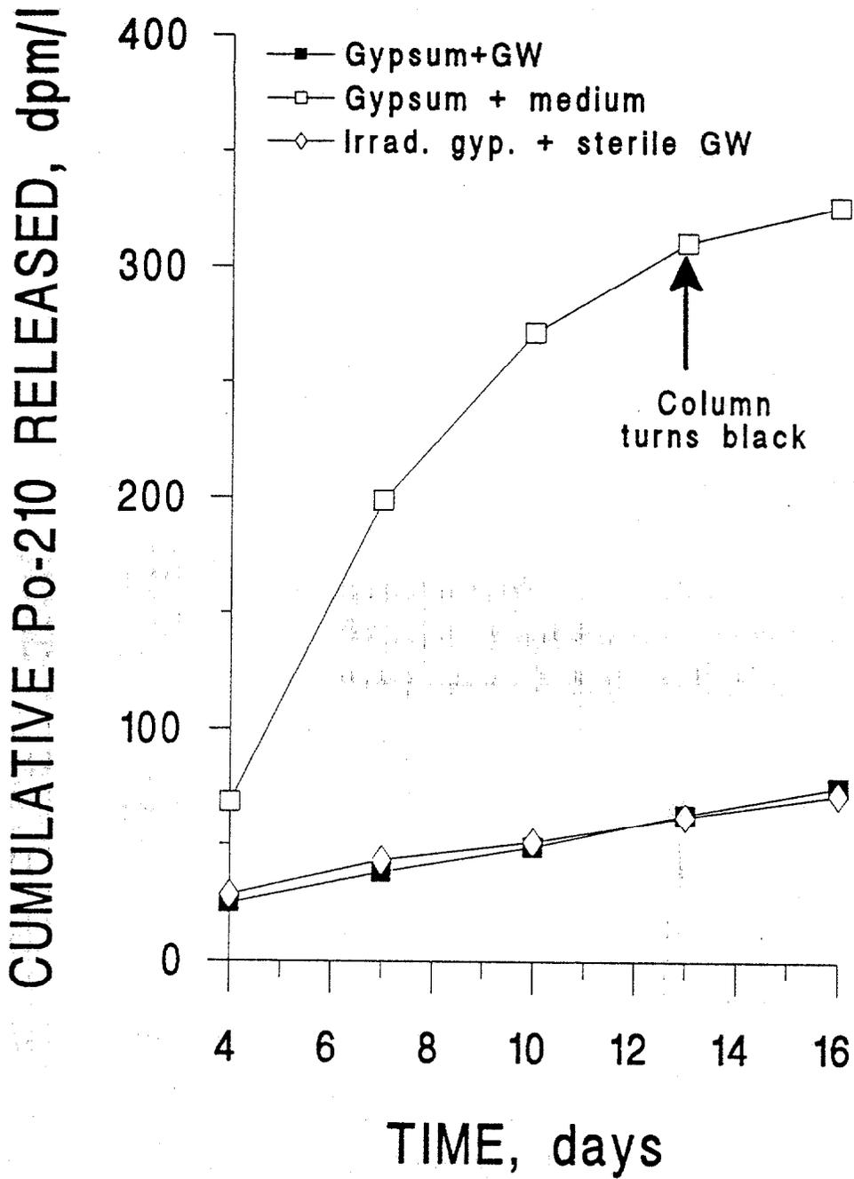
Fig. 4.8. Polonium release by naturally occurring gypsum microflora under varying nutrient conditions. Symbols: gypsum fed ground water (solid squares), sterile gypsum fed sterile ground water (open diamonds), gypsum fed PYE medium (open squares).
