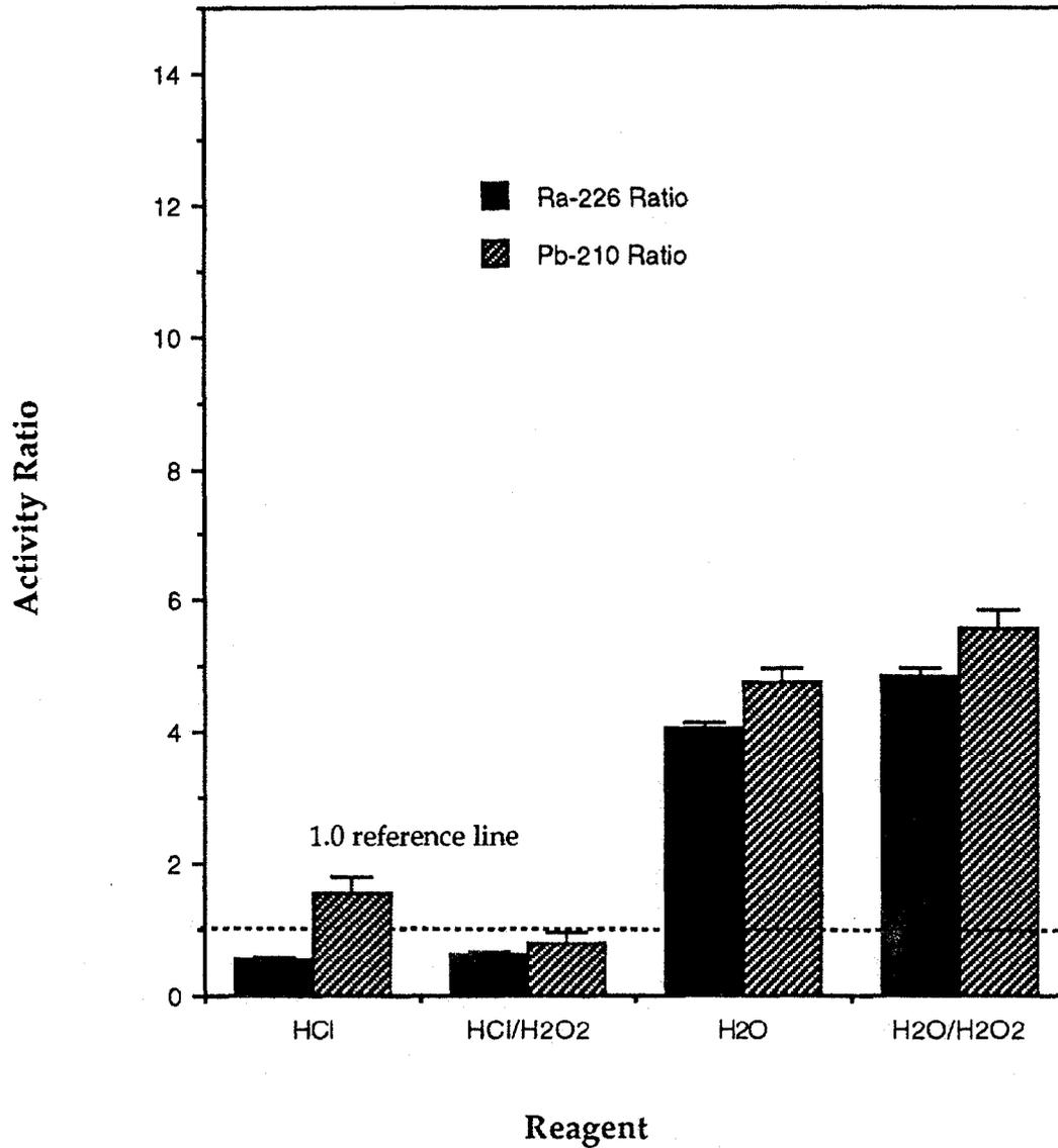
**Figure 2-5.** Selective leaching results with various reagents for phosphogypsum sample Gyp-6. The enrichment or depletion of  $^{226}\text{Ra}$ , expressed as an activity ratio in the residue to that originally present is shown for each of the reagents tested by the black bars. The  $^{210}\text{Pb}$  enrichment/depletion is shown by the striped bars. Solutions were unfiltered in these experiments.
