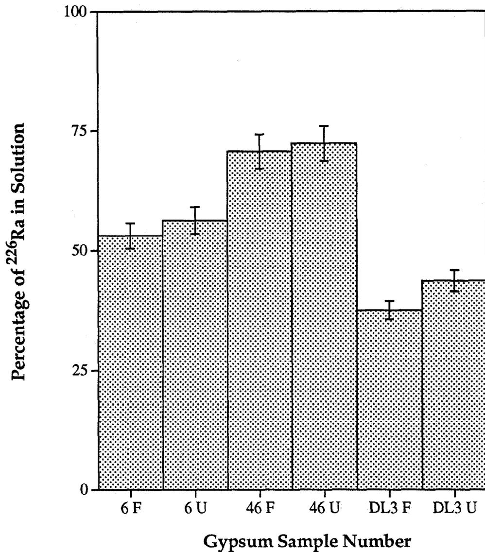
**Figure 2-9.** Plots of the percentages of  $^{226}\text{Ra}$  in solution in "D" series dissolution experiments. Data for both filtered (F) and unfiltered (U) solutions are shown. The percentages plotted are mean values of  $^{226}\text{Ra}$  in solution in 2 dissolutions of Gyp-6, 4 dissolutions of Gyp-46, and 5 dissolutions of Gyp DL3. Error bars represent  $1\sigma$  of the mean values. Activities of  $^{226}\text{Ra}$  in solution were measured by Rn emanation.
