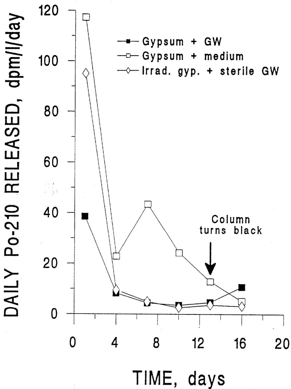
Fig. 4.9. Daily Po release by naturally occurring gypsum microflora under varying nutrient conditions. Symbols and treatments are the same as in Fig. 8.
