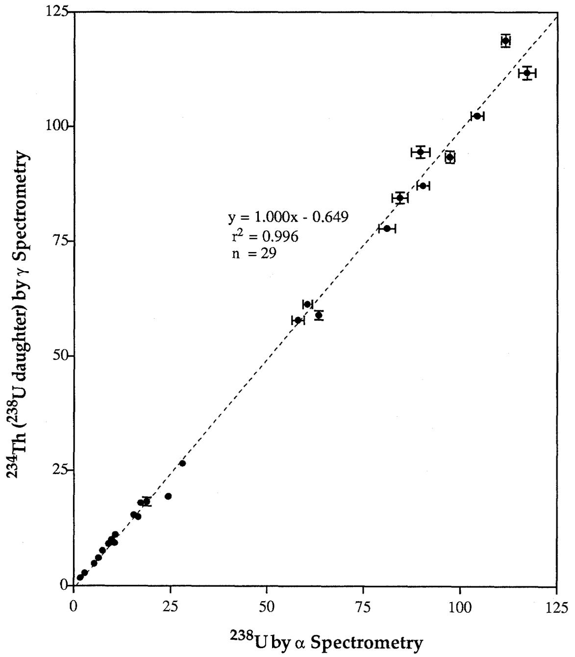
Fig. 1-8 Plot of  $^{238}\text{U}$  activities measured by  $\gamma$ -ray spectrometry *versus*  $^{238}\text{U}$  activities determined by isotope dilution  $\alpha$ -spectrometry. All activities are in dpm/g.
