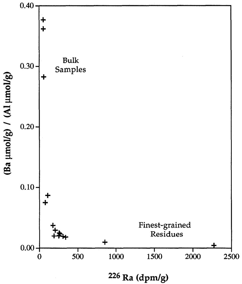
Figure 2-15. Plot of  $(Ba \mu\text{mol/g}) / (Al \text{ mmol/g})$  versus  $^{226}\text{Ra}$  (dpm/g).
