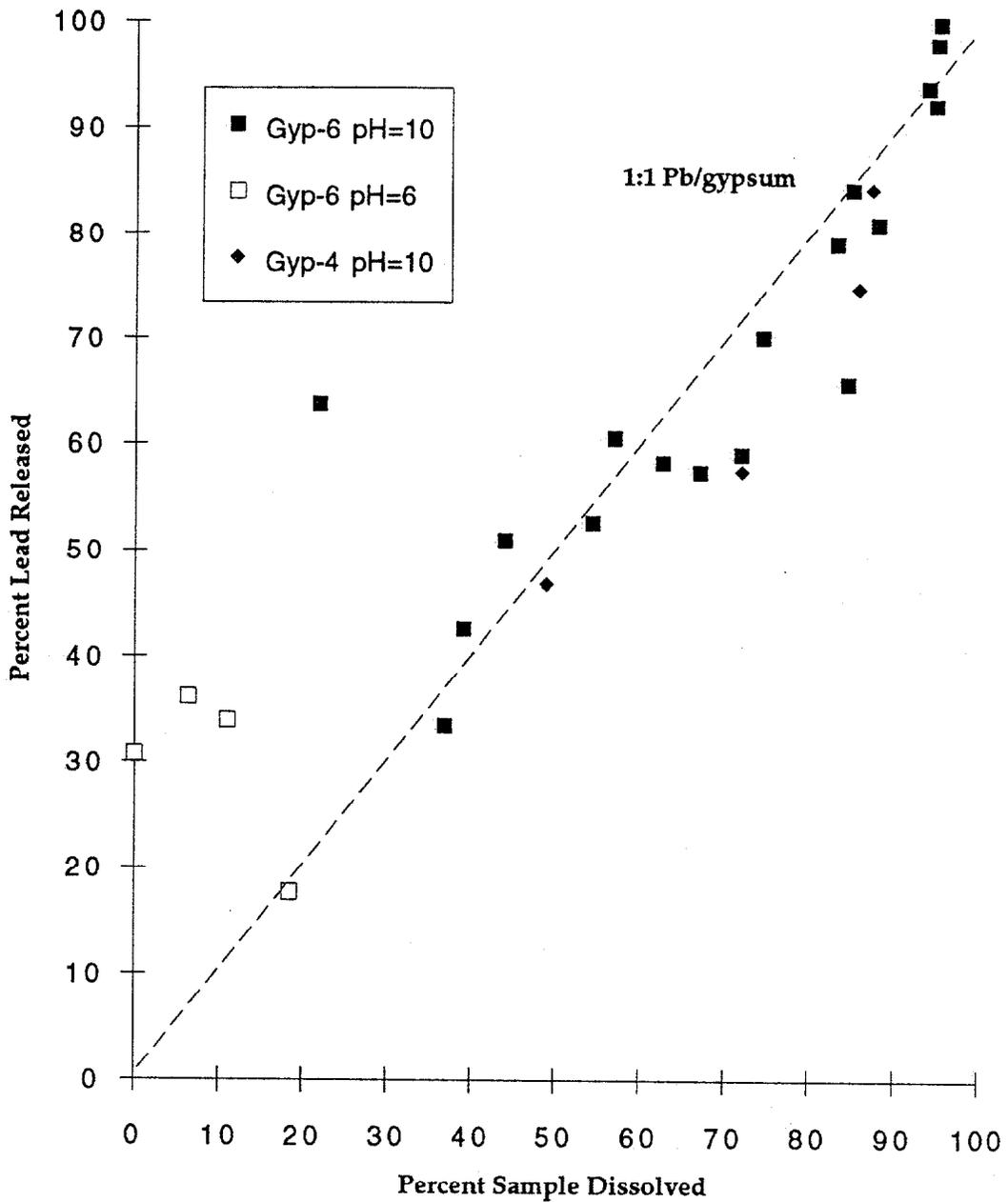
**Figure 2-4.** Percent  $^{210}\text{Pb}$  released into EDTA *versus* percent sample dissolved from two phosphogypsum samples, Gyp-4 and Gyp-6 at pH=10 (solid symbols) and Gyp-6 at pH=6 (open squares). The 1:1 reference line shows where the data would plot if  $^{210}\text{Pb}$  was congruently released during the dissolution of  $\text{CaSO}_4 \cdot n \text{H}_2\text{O}$ . This plot is based on radiochemical analysis of  $^{210}\text{Pb}$  in the residues remaining after leaching.
