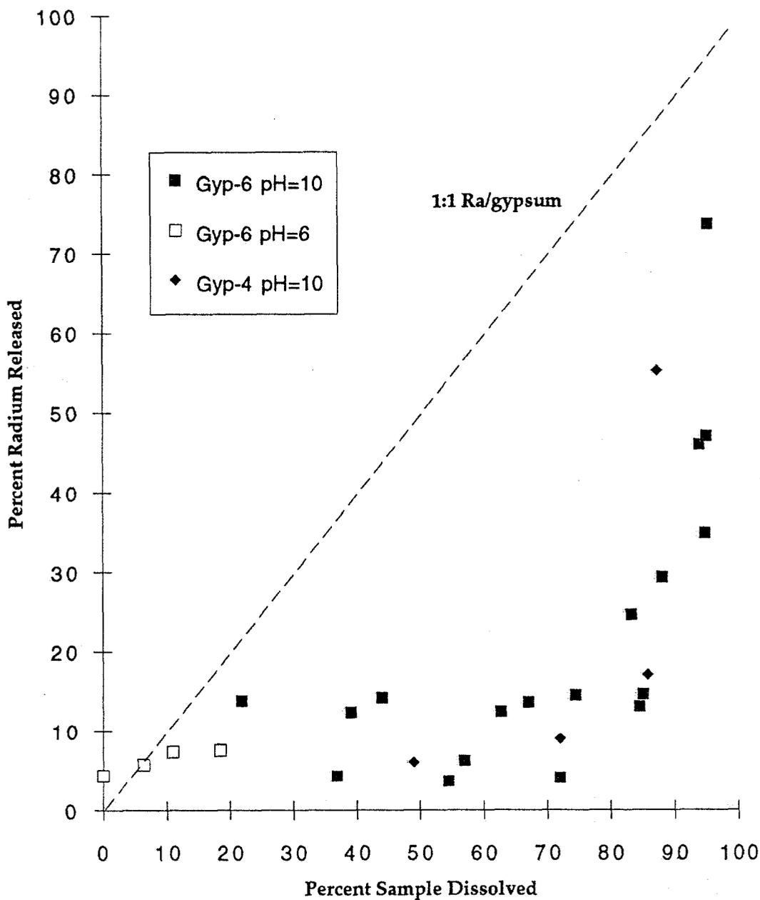
**Figure 2-3.** Percent  $^{226}\text{Ra}$  released into EDTA *versus* percent sample dissolved from phosphogypsum samples Gyp-6 at pH=10 (solid symbols) and Gyp-6 at pH=6 (open squares). The 1:1 reference line shows where the data would plot if  $^{226}\text{Ra}$  was uniformly distributed as a lattice constituent of  $\text{CaSO}_4 \cdot n \text{H}_2\text{O}$  and was released during dissolution without any subsequent adsorption.
