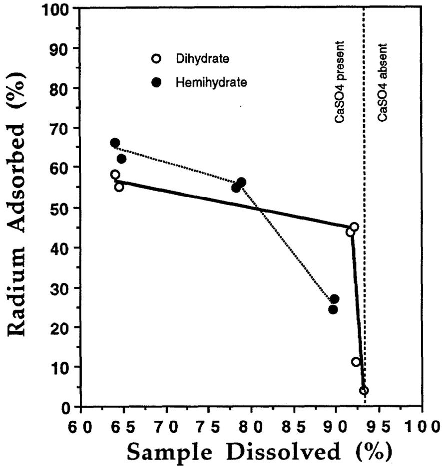
**Figure 2-8.** Radium adsorption experiment results for the dissolution of two crystalline forms of Gyp-6 in DDW. The proportional decrease in radium adsorption with the amount of undissolved  $\text{CaSO}_4 \cdot n \text{H}_2\text{O}$  implies that  $\text{CaSO}_4 \cdot n \text{H}_2\text{O}$  is the primary phase which adsorbs radium. Very little adsorption onto the insoluble residue is indicated.
