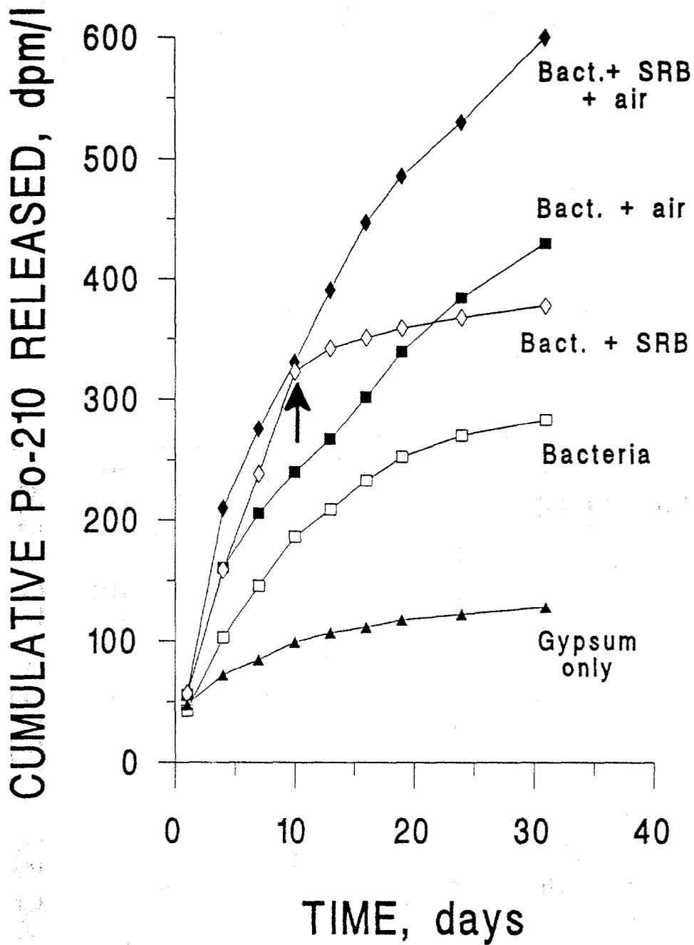
Fig. 4.3. The effect of purging the columns with air to control redox conditions. Sterilized gypsum columns were treated as follows: BACT addition (open squares), Bact+SRB addition (open diamonds), BACT plus air purging (solid squares), BACT+SRB plus air purging (solid diamonds), gypsum alone (solid triangles). The arrow indicates when the unpurged BACT+SRB column turned black indicating the formation of FeS.
