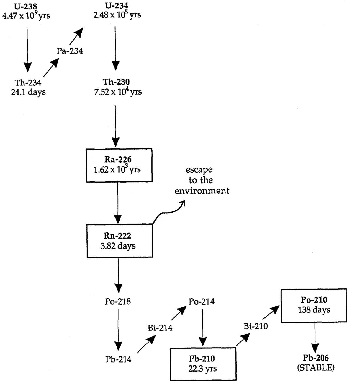
Fig. 1-1 Natural  $^{238}\text{U}$  decay chain with nuclides of interest to this study enclosed in boxes. Downward arrows indicate alpha particle decay and diagonal arrows represent beta decay.
