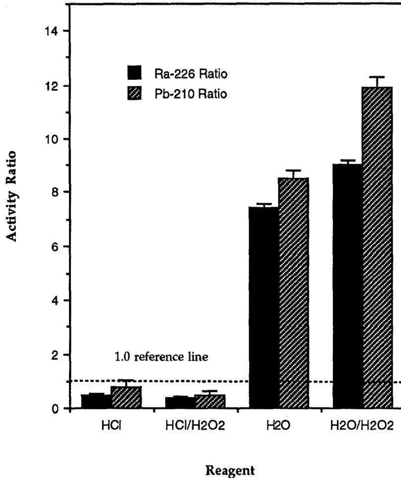
**Figure 2-7.** Results from a second replicate selective leaching experiment with various reagents for phosphogypsum sample Gyp-6. The enrichment or depletion of  $^{226}\text{Ra}$ , expressed as an activity ratio in the residue to that originally present is shown for each of the reagents tested by the black bars. The  $^{210}\text{Pb}$  enrichment/depletion is shown by the striped bars. Solutions were again filtered in these experiments.
