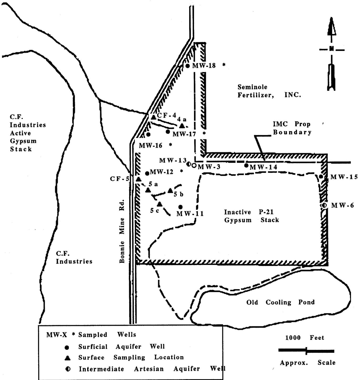
Fig. 1-3 Monitor wells sampled around the IMC P-21 gypsum stack, Bartow, Florida. Samples have been collected from wells 11, 12, 16, 17, and 18.
