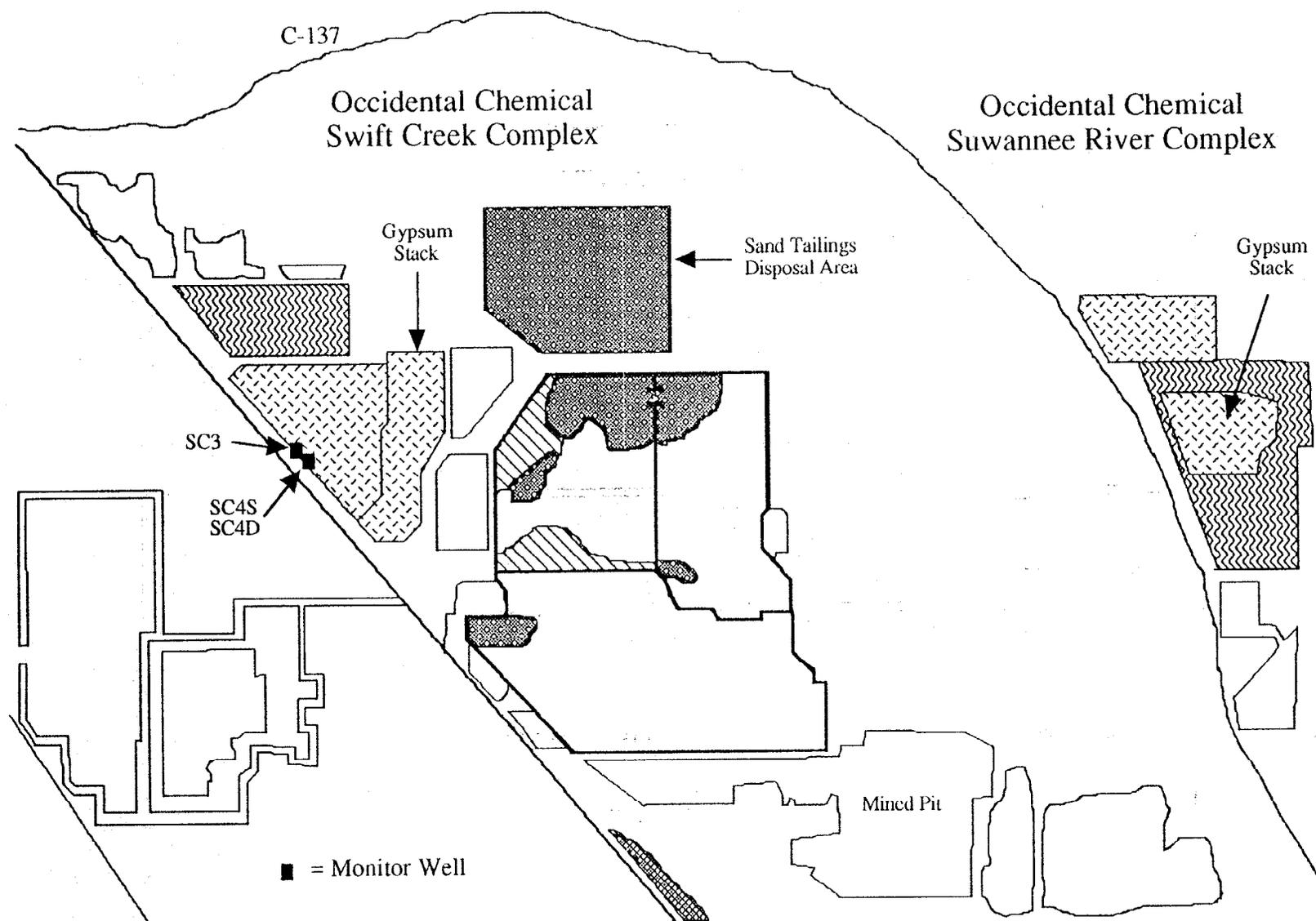
Fig. 1-6 Monitor wells sampled around a gypsum stack at Occidental Chemical, White Springs, Florida. Water samples were collected from wells 3S, 4D, and 4S.
