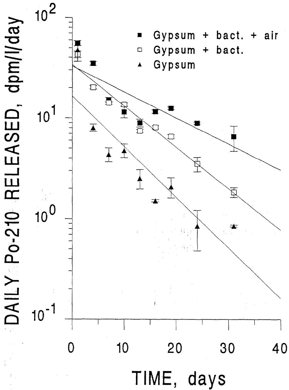
Fig. 4.5. Polonium release by the BACT mixture alone with and without air purging. The treatments were: BACT plus air (solid squares), BACT without air (open squares), and gypsum alone (solid triangles).
