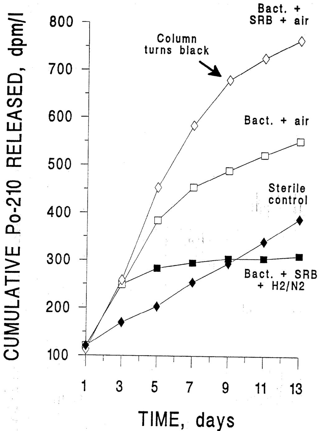
Fig. 4.6. The effect of initiating anaerobiosis by purging with either H<sub>2</sub> or N<sub>2</sub> gas. Air purging enhanced Po release while inducing anaerobiosis and SRB activity reduced Po release. The treatments were: BACT+SRB plus H<sub>2</sub>-N<sub>2</sub> (solid squares), BACT+SRB plus air (open diamonds), BACT plus air (open squares), gypsum alone (solid diamonds).
