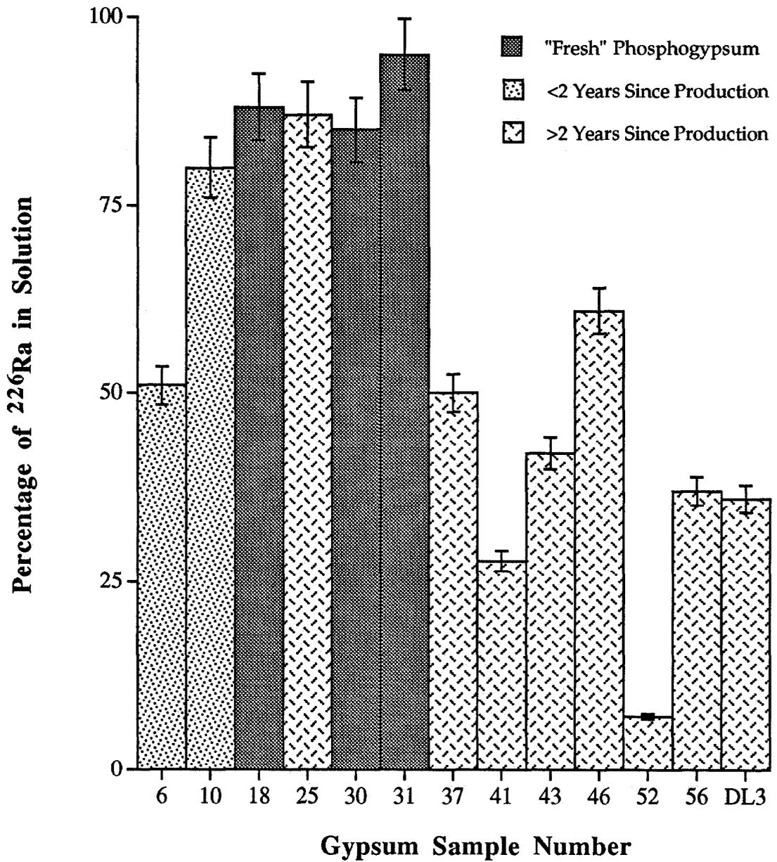
**Figure 2-10.** Plots of the percentages of  $^{226}\text{Ra}$  in solution for "SD" series samples. Solutions were filtered to  $0.45\ \mu\text{m}$  and  $^{226}\text{Ra}$  in solution was measured by Rn emanation. Percentages are a mean of 3 analyses for each solution and the error bars represent standard deviations at the  $1\sigma$  level.
