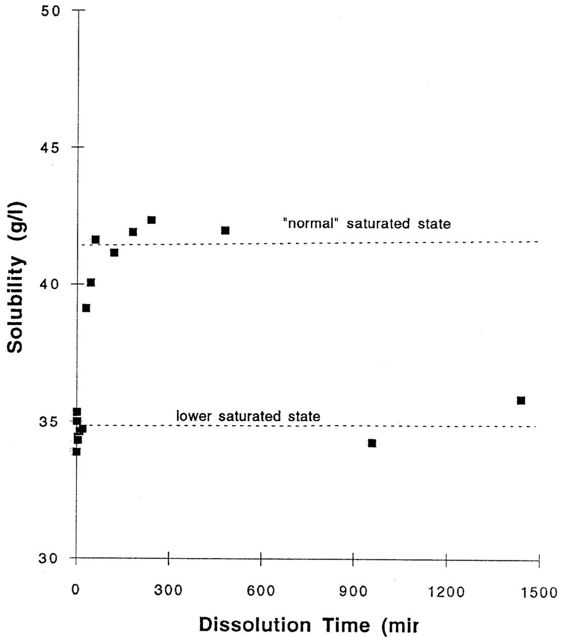
**Figure 2-2.** Solubility of phosphogypsum sample Gyp-4 *versus* time of dissolution. This curve shows that gypsum dissolves very quickly in EDTA. The solution reaches the theoretical saturated state within the first hour and returns to a lower apparent solubility after about 8 hours.
