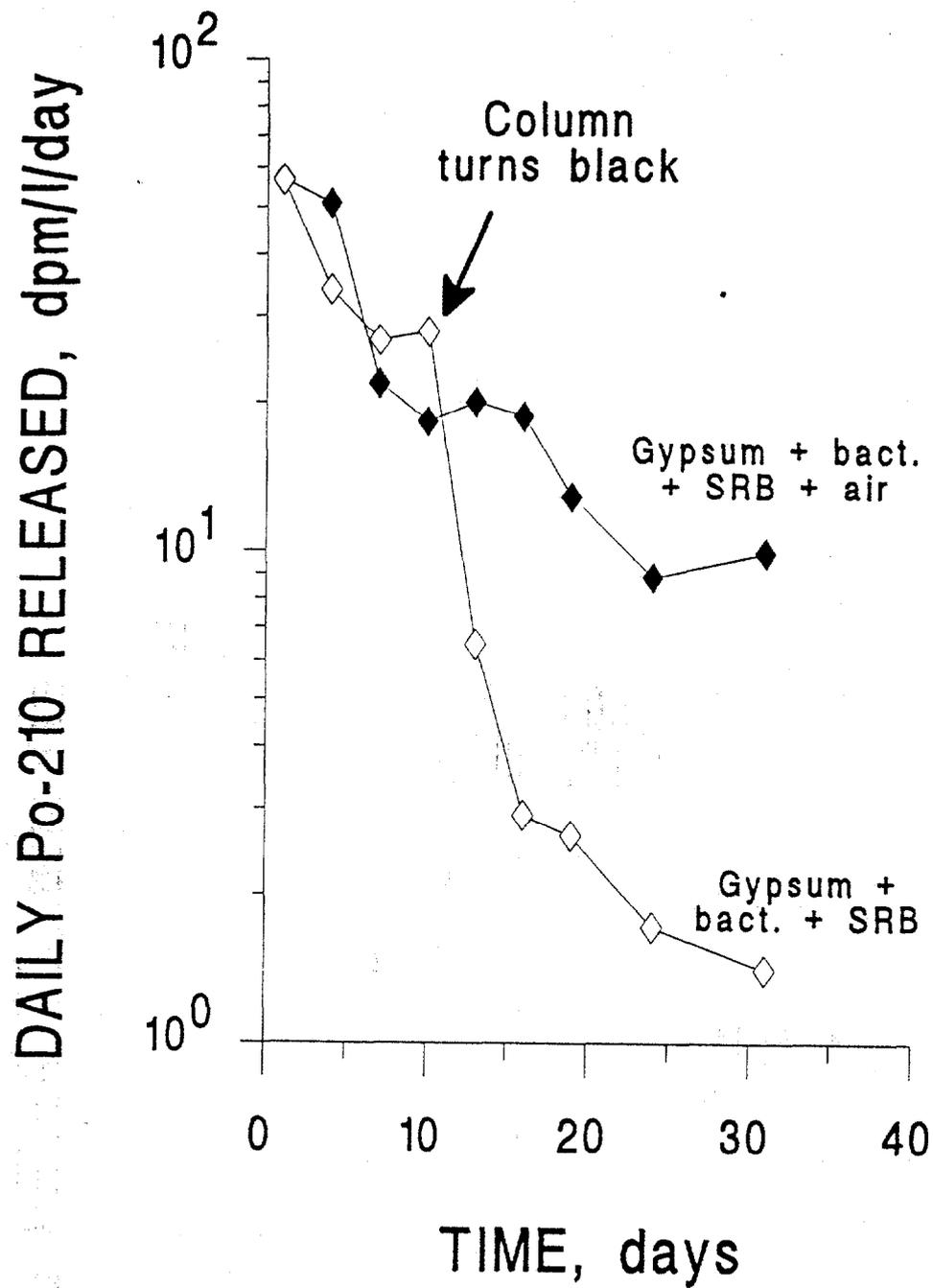
Fig. 4.4. A comparison of the air purged and unpurged columns containing SRB. Once FeS forms in the unventilated column Po release ceases dramatically. Symbols: Solid diamonds, BACT+SRB plus air; open diamonds, BACT+SRB only.
