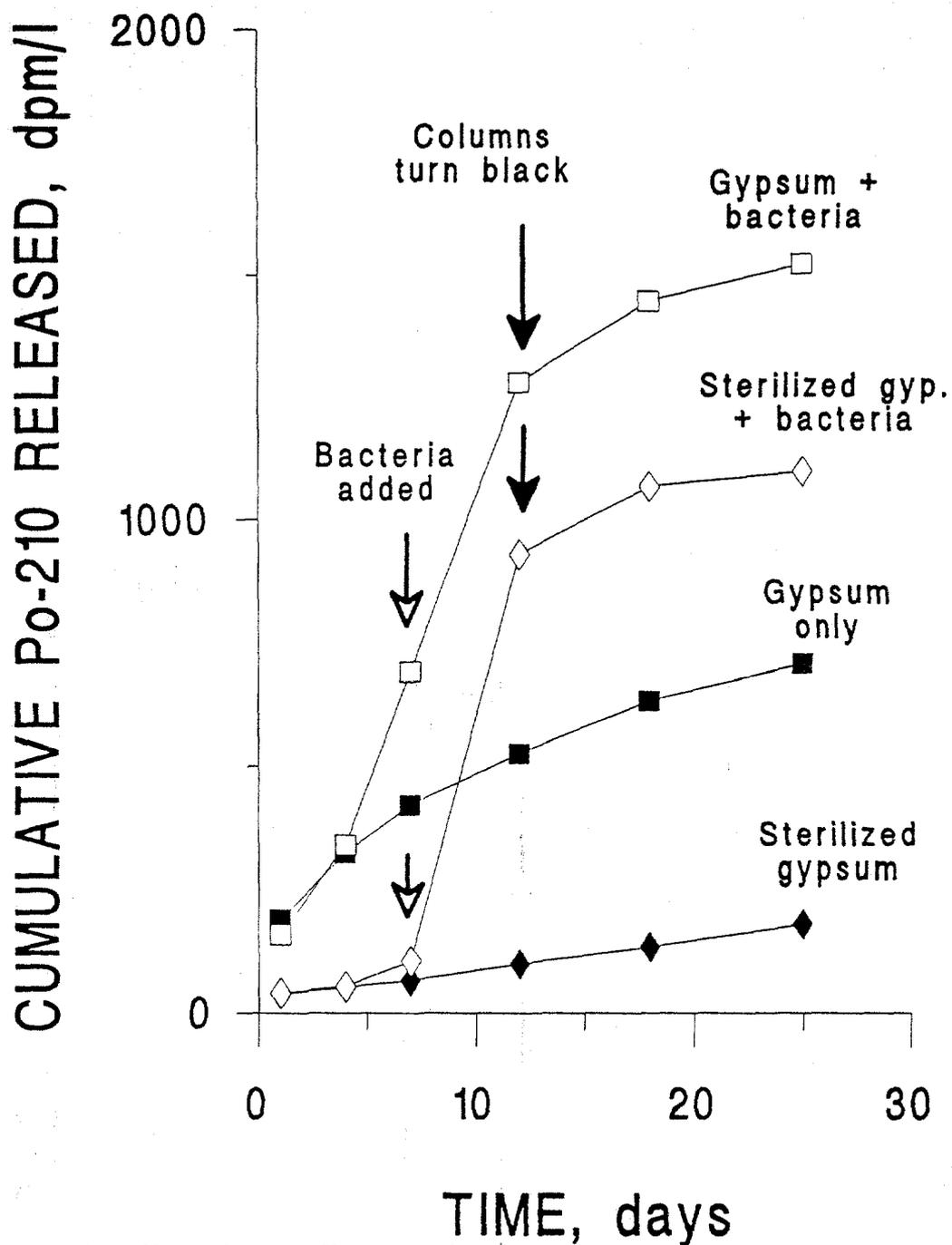
Fig. 4.1. The effect of naturally occurring and cultured bacteria on the cumulative release of Po from gypsum. Columns received the following treatments: the natural gypsum microflora alone (solid squares), the natural gypsum microflora plus the BACT-SRB mixture (open squares), sterilized gypsum plus the BACT-SRB mixture (open diamonds) and sterilized gypsum alone (solid diamonds). The arrows indicate when BACT-SRB were added or when the columns turned black indicating FeS formation.
