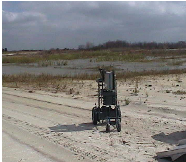
Figure 21. Spectrometer Measuring the Gamma Energy Spectra at the Sand Tailings Area.
