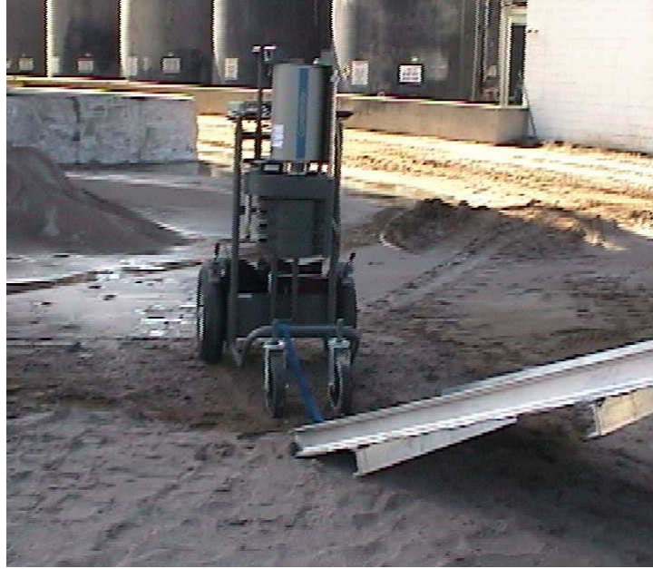
Figure 20. Spectrometer Measuring Gamma Radiation Emitted by the Pile of Spilled Concentrated Phosphate at a Mining Site.
