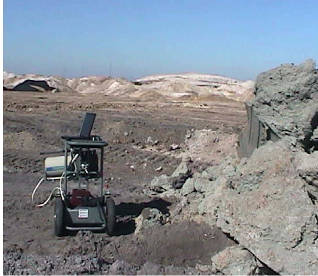
Figure 19. Gamma Spectrometer Measuring the Radiation Field of Freshly Dumped Phosphate Ore Matrix.
