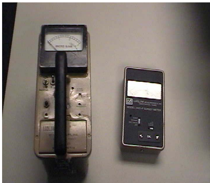
Figure 1. The Ludlum 12-S and 2401-P Survey Meters (from Left to Right) Used in This Study.
