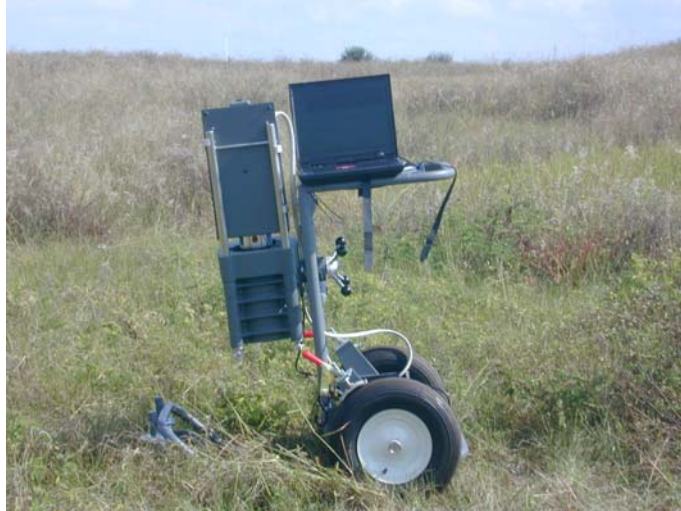
Figure 7. The BEGe Detector, Pointed Downwards, with Laptop Computer at the Sand Tailings Area of Tenoroc State Park.
