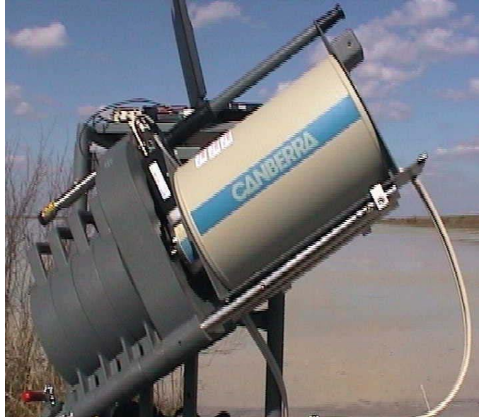
Figure 8. Side View of the BEGe Detector to Allow Viewing the Shield Configuration.
