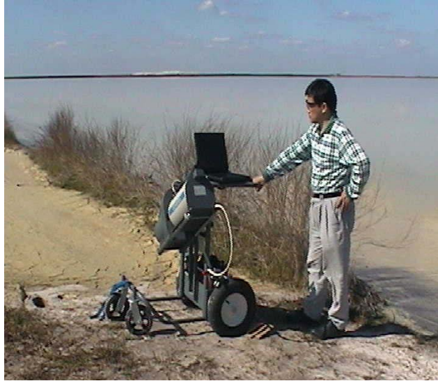
Figure 22. Spectrometer Measuring the Gamma Radiation Field at the Clay Settling Pond at Mine Site B.
