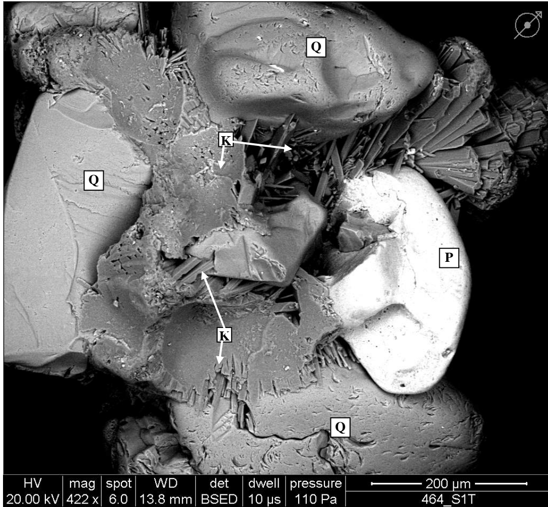
Figure 66. SEM Micrograph of Hole 464 Split 1 Tailings in Which the Phosphate Particle Is Attached to Quartz Particles by Crystalline and Noncrystalline Kaolinite Mineral.
