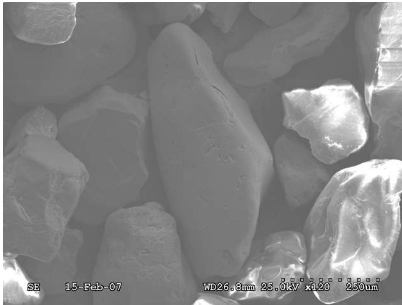
Figure 15. SEM Image of EDS Particle 3 from CF Industries Bad Feed Sample.
