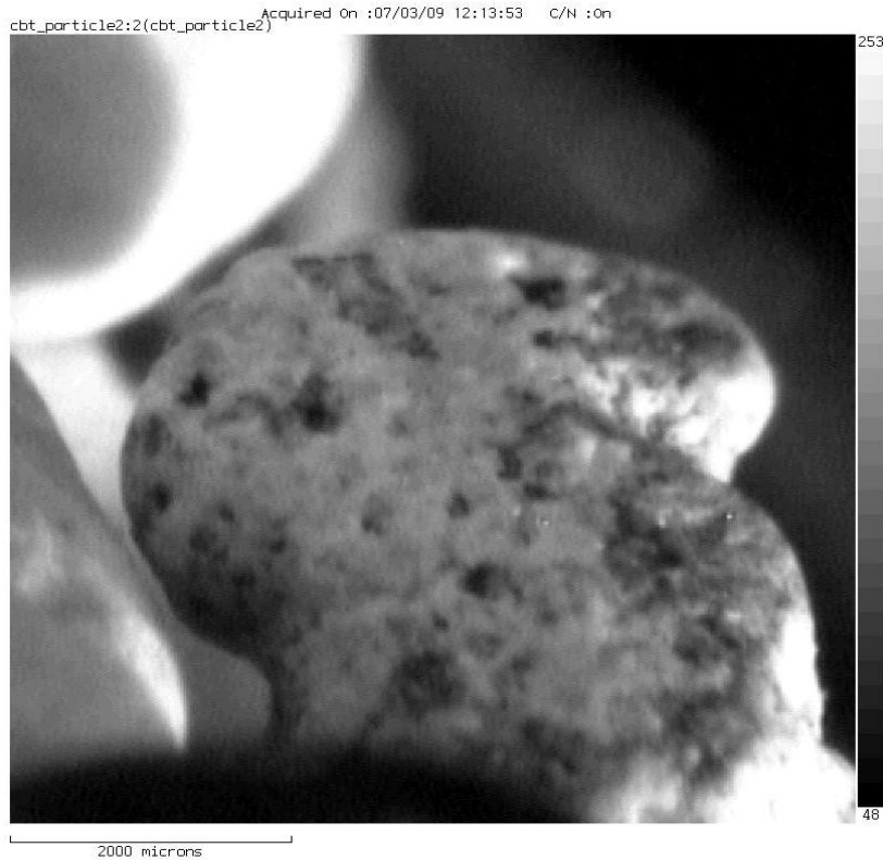
Figure 19. Electron Image of XPS Particle 2 from CF Industries Bad Tailings Sample.
