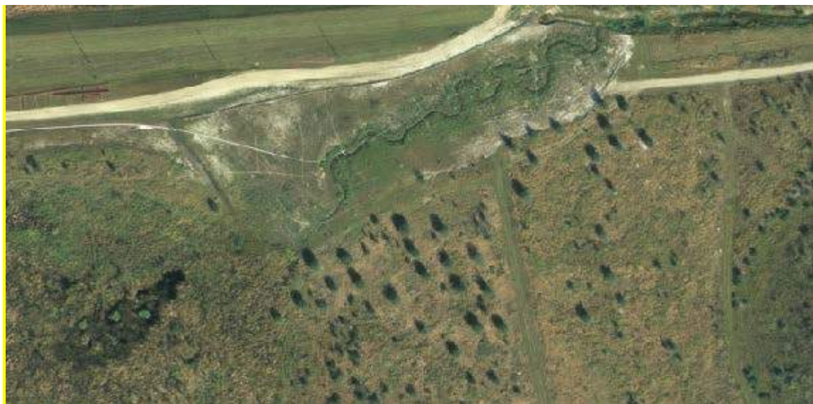
Image flown 2010, post-construction, DB-5 stream reclamation site. Meander pattern copied from a natural site and applied to restoration design.
