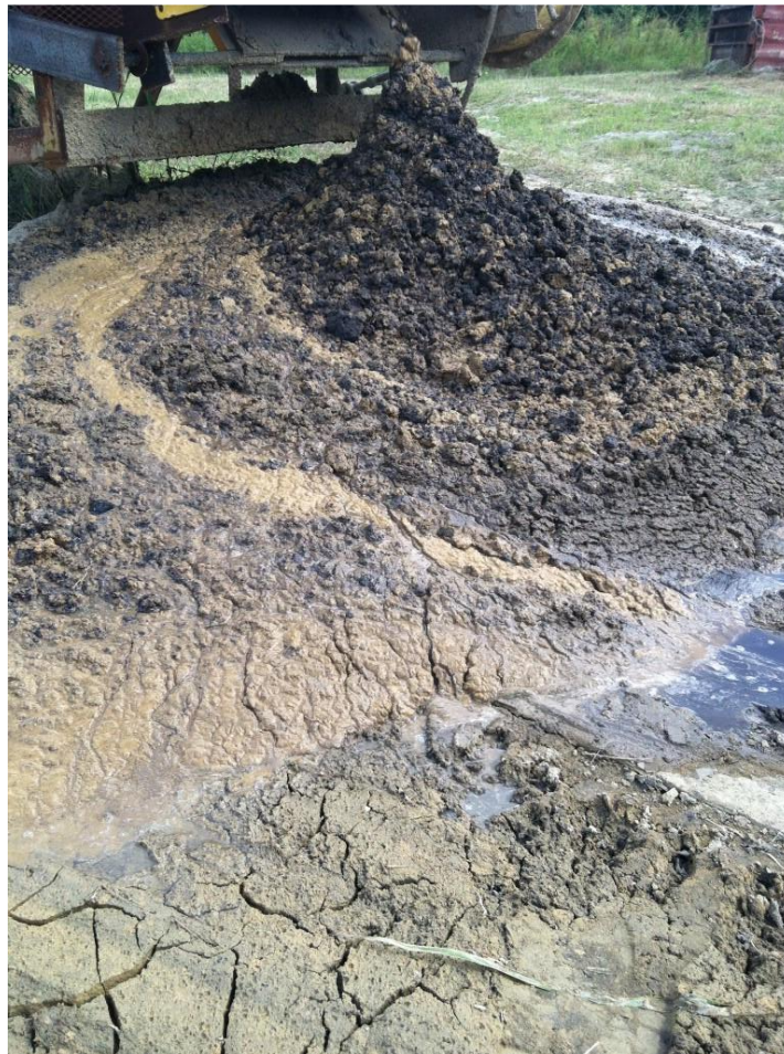
Figure 13. Paste Discharging from the Dewatering Belt
