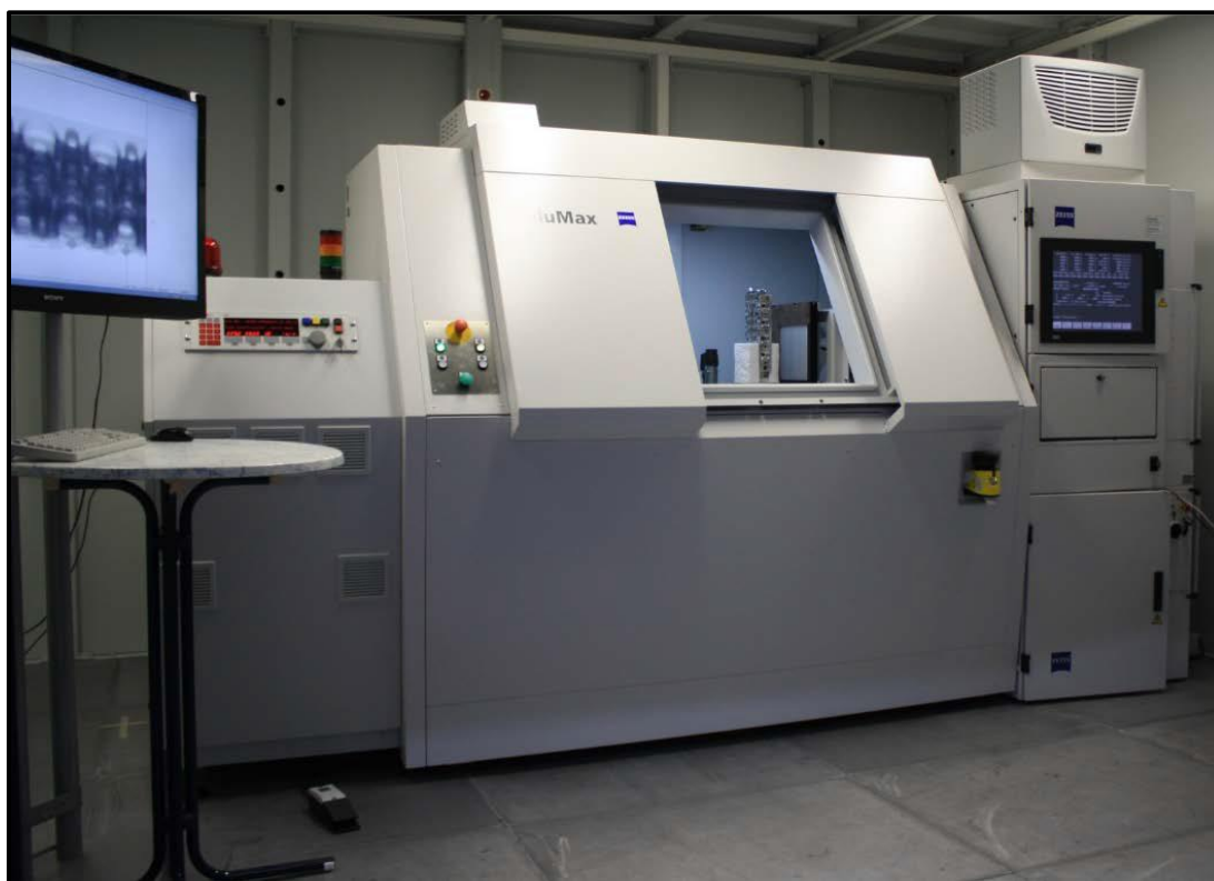
ZEISS VoluMax 800 CT Machine for High-speed X-Ray Tomography.
